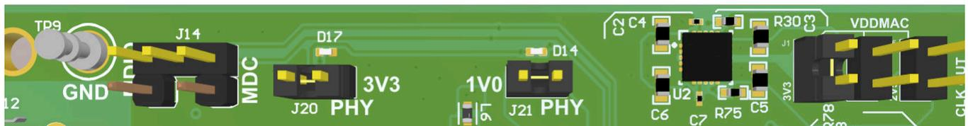
Figure 2-3. Onboard Supply Connection and Jumpers
