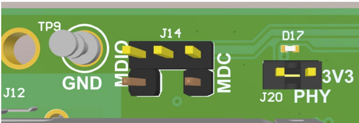
**Figure 2-5. Onboard MSP Connections for MDIO and MDC**
