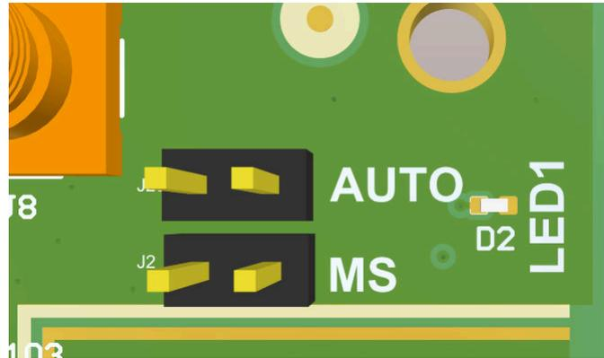
**Figure 2-6. DP83TC813 Configured in Autonomous and Slave Modes**
