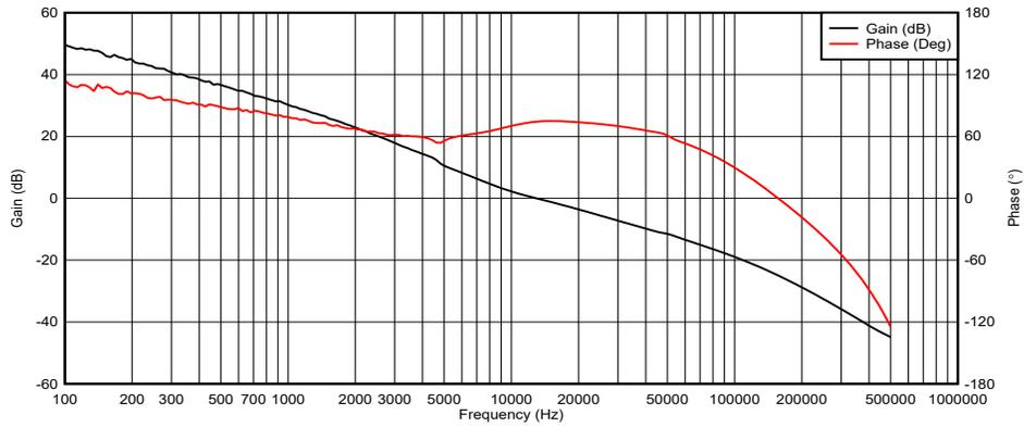
**Figure 5-15. Control Loop Response,  $V_{IN} = 3.3V$ ,  $I_{OUT} = 0.6A$**
