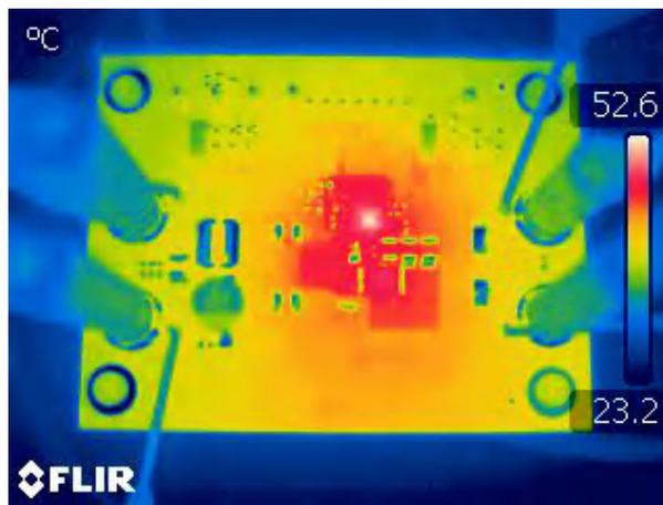
Figure 5-5. Thermal Image:  $V_{IN} = 6V$ ,  $I_{OUT} = 1.2A$ ,  $V_{BIAS} = 6V$ , No Forced Air Cooling
