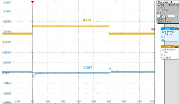
Figure 5-12. Load Transient,  $V_{IN} = 3.3V$ ,  $I_{OUT} = 0.4A$  to  $0.8A$
