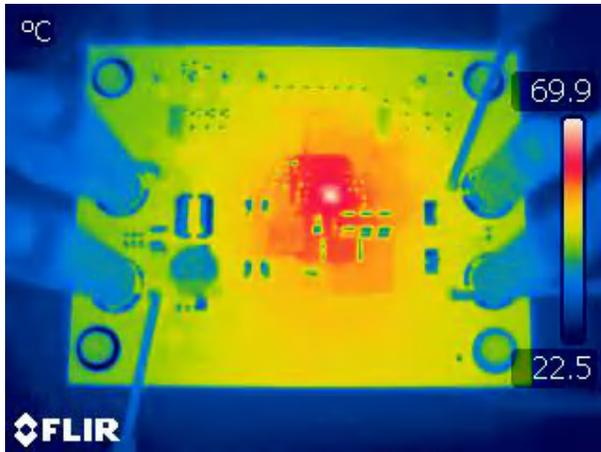
Figure 5-3. Thermal Image:  $V_{IN} = 3.3V$ ,  $I_{OUT} = 0.6A$ ,  $V_{BIAS} = 3.3V$ , No Forced Air Cooling
