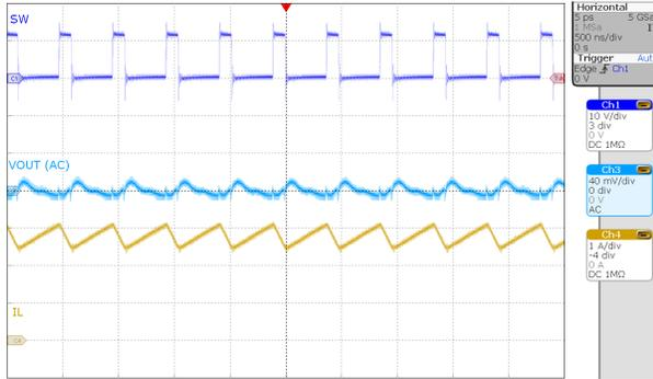
Figure 5-6. Steady State,  $V_{IN} = 3.3V$ ,  $I_{OUT} = 0.6A$
