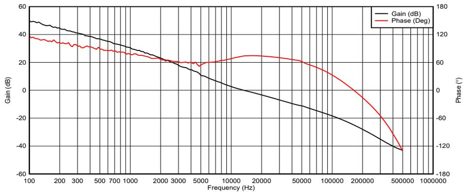
**Figure 5-17. Control Loop Response,  $V_{IN} = 9V$ ,  $I_{OUT} = 1.2A$**
