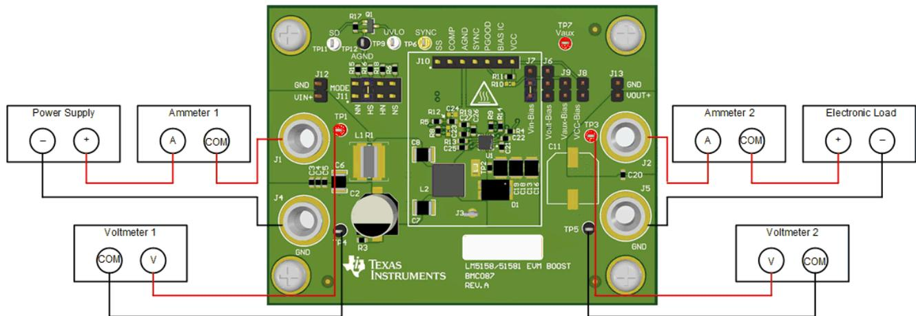
**Figure 4-1. Test Setup**
