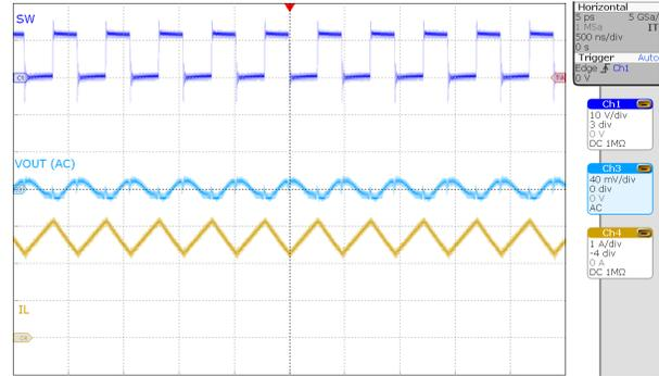
Figure 5-7. Steady State,  $V_{IN} = 6V$ ,  $I_{OUT} = 1.2A$
