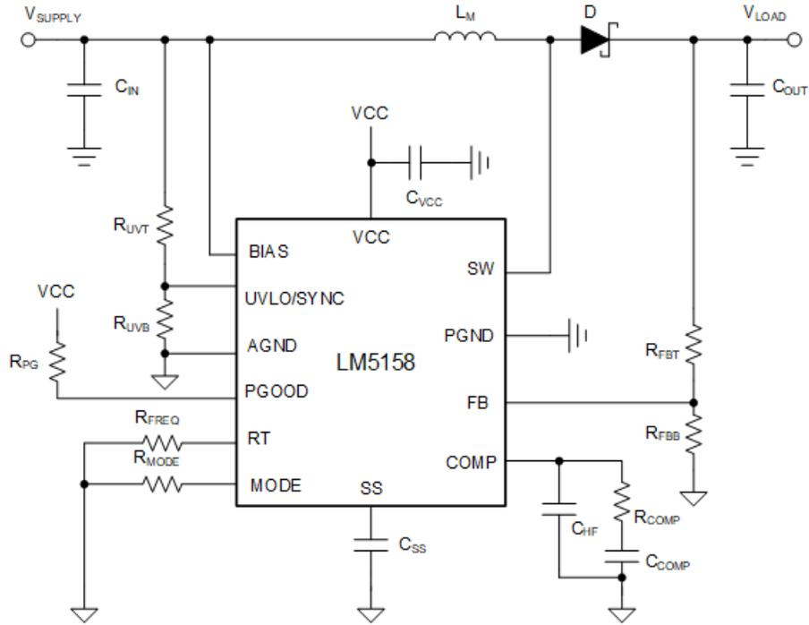
Figure 2-1. Application Circuit
