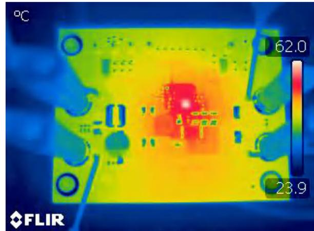
Figure 5-4. Thermal Image:  $V_{IN} = 3.3V$ ,  $I_{OUT} = 0.6A$ ,  $V_{BIAS} = 12V$ , No Forced Air Cooling
