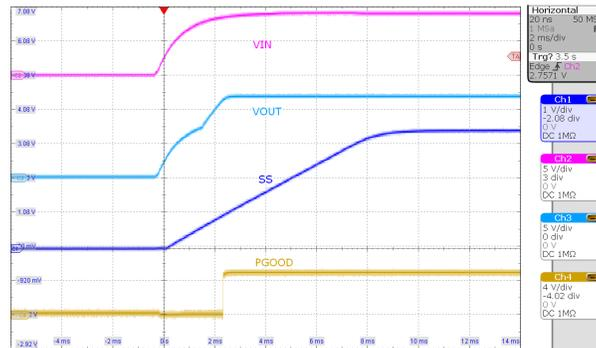
Figure 5-11. Start-Up,  $V_{IN} = 9V$ ,  $I_{OUT} = 1.2A$
