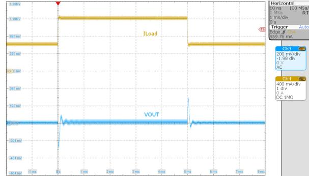
Figure 5-13. Load Transient,  $V_{IN} = 6V$ ,  $I_{OUT} = 0.6A$  to  $1.2A$
