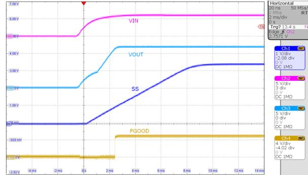
Figure 5-10. Start-Up,  $V_{IN} = 6V$ ,  $I_{OUT} = 1.2A$
