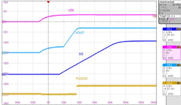
Figure 5-9. Start-Up,  $V_{IN} = 3.3V$ ,  $I_{OUT} = 0.6A$
