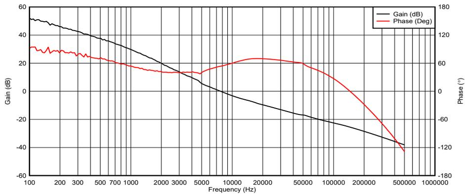
**Figure 5-16. Control Loop Response,  $V_{IN} = 6V$ ,  $I_{OUT} = 0.6A$**
