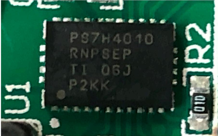
Figure 1-4. TPS7H4010-SEP Package Marking
