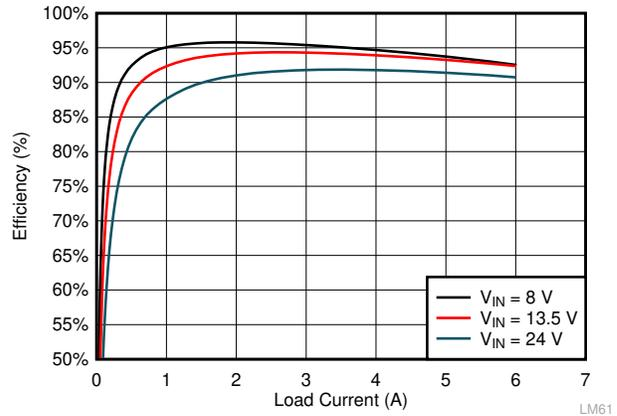
Figure 6-12.  $F_{SW} = 2.1$  MHz, 5 VOUT, FPWM Mode
