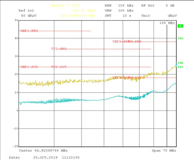
**Figure 6-2. Conducted EMI Measurement with CISPR 25 Class 5 Limit Lines (30 MHz to 108 MHz)**
