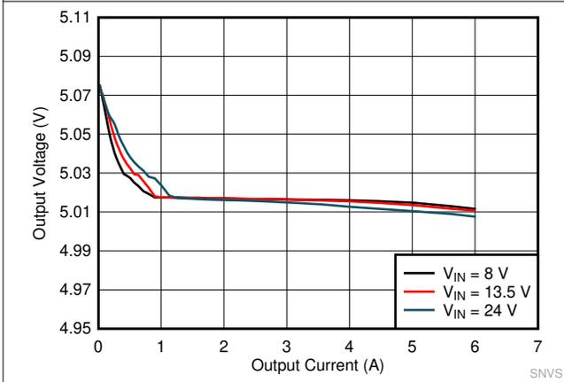
Figure 6-19.  $F_{SW} = 2.1 \text{ MHz}$ , 5 VOUT, Auto Mode
