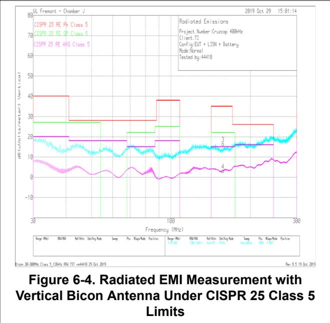
**Figure 6-4. Radiated EMI Measurement with Vertical Bicon Antenna Under CISPR 25 Class 5 Limits**
