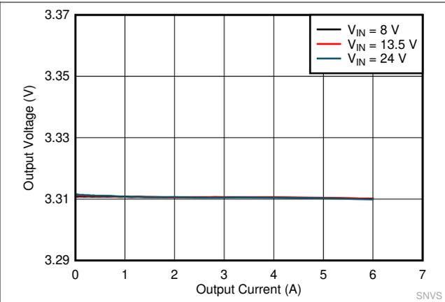
Figure 6-18.  $F_{SW} = 400 \text{ kHz}$ , 3.3 VOUT, FPWM Mode
