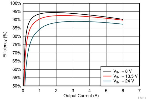
Figure 6-14.  $F_{SW} = 2.1$  MHz, 3.3 VOUT, FPWM Mode
