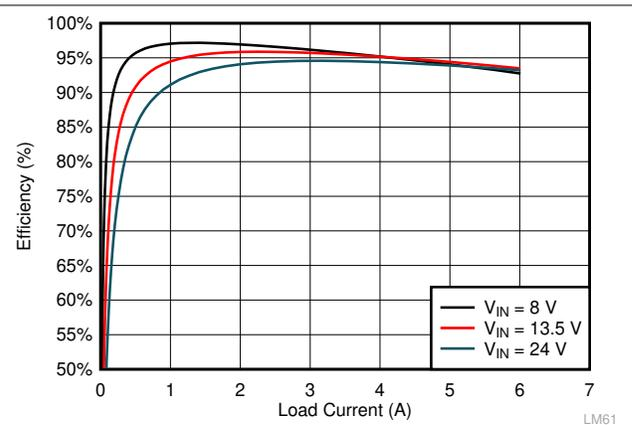
**Figure 6-8.  $F_{sw} = 400$  kHz, 5 VOUT, FPWM Mode**
