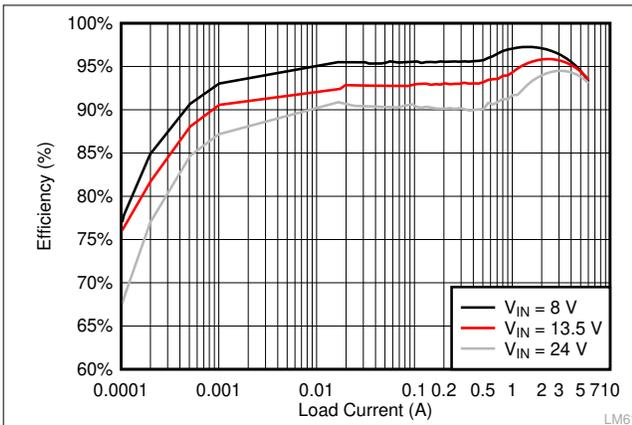
**Figure 6-7.  $F_{sw} = 400$  kHz, 5 VOUT, Auto Mode**
