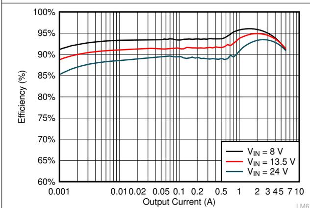
**Figure 6-9.  $F_{sw} = 400$  kHz, 3.3 VOUT, Auto Mode**
