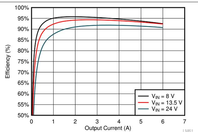
**Figure 6-10.  $F_{sw} = 400$  kHz, 3.3 VOUT, FPWM Mode**
