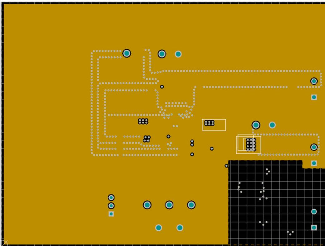
Figure 5-3. Signal Layer 1 - Ground Plane
