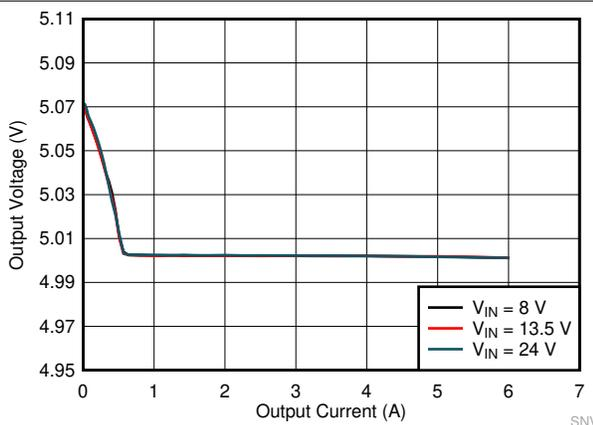
Figure 6-15.  $F_{SW} = 400$  kHz, 5 VOUT, Auto Mode
