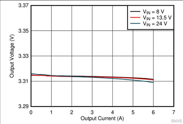
Figure 6-22.  $F_{SW} = 2.1 \text{ MHz}$ , 3.3 VOUT, FPWM Mode
