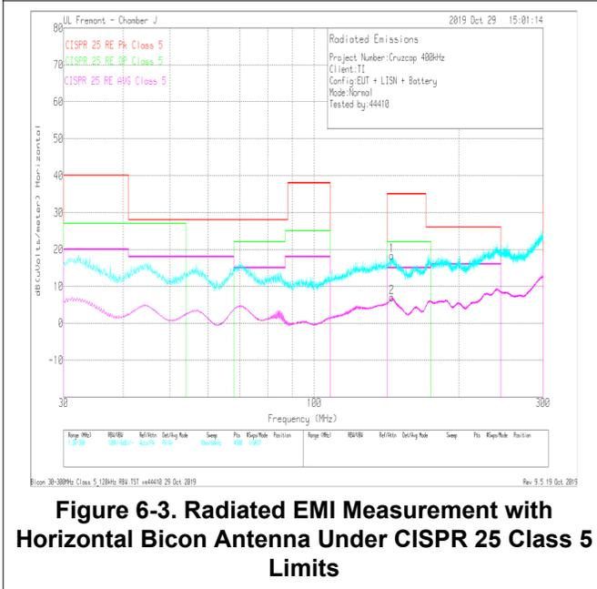
**Figure 6-3. Radiated EMI Measurement with Horizontal Bicon Antenna Under CISPR 25 Class 5 Limits**
