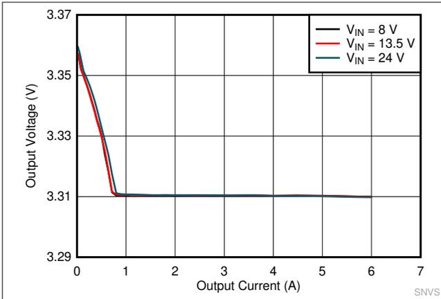
Figure 6-17.  $F_{SW} = 400 \text{ kHz}$ , 3.3 VOUT, Auto Mode
