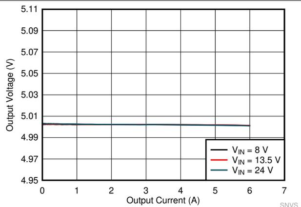
Figure 6-16.  $F_{SW} = 400$  kHz, 5 VOUT, FPWM Mode
