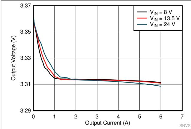
Figure 6-21.  $F_{SW} = 2.1 \text{ MHz}$ , 3.3 VOUT, Auto Mode
