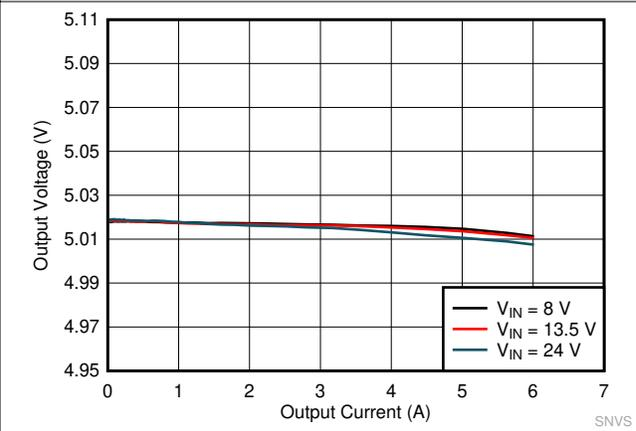
Figure 6-20.  $F_{SW} = 2.1 \text{ MHz}$ , 5 VOUT, FPWM Mode
