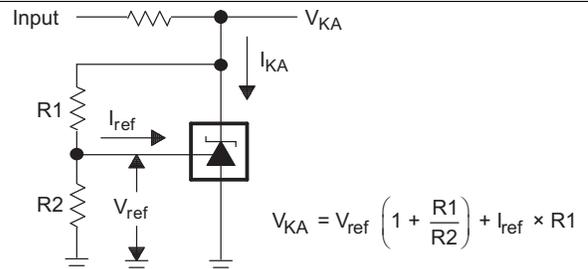
Figure 5. Test Circuit for  $V_{KA} > V_{ref}$
