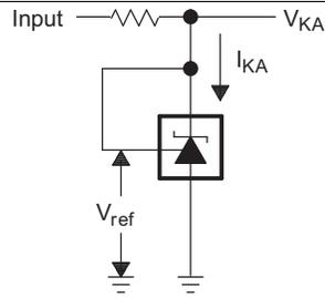
Figure 4. Test Circuit for  $V_{KA} = V_{ref}$
