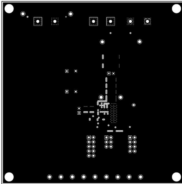
**Figure 8-3. Layer 2 Copper (Top View)**
