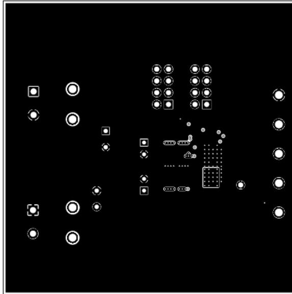
**Figure 9. Layer 2 Copper (Top View)**
