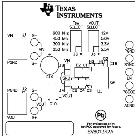
Figure 7. Topside Component Layout (Top View)
