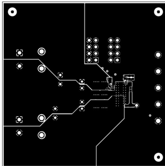
Figure 8. Topside Copper (Top View)
