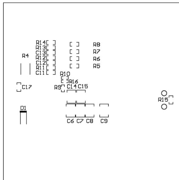
Figure 12. Bottom-Side Component Layout (Bottom View)
