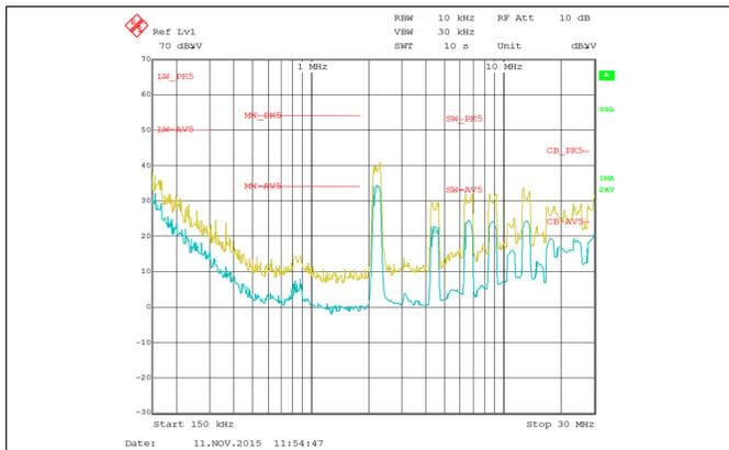
Figure 8. CISPR 25 Class 5 Peak Detection
