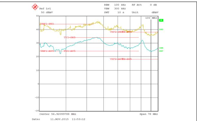
Figure 9. CISPR 25 Class 5 Peak Detection
