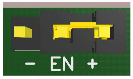
Figure 1. Enable Jumper Settings
