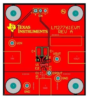
Figure 2. Top Assembly Layer
