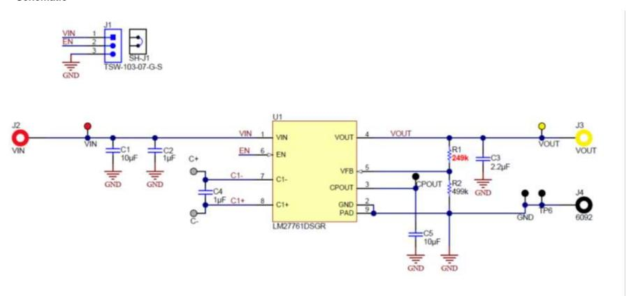
Figure 4. LM27761EVM Schematic
