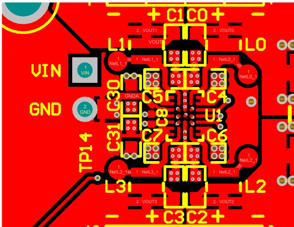
Input capacitors are placed close to the LP8758-E0 and routed on top layer. GND nets are connected to the GND plane (2nd layer) with microvias. VIN nets are connected to the VIN plane (3rd layer) with vias in pads of the input capacitors. VOUT pads of the output capacitors and inductors are connected together with large copper area.
