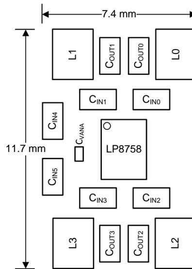
Figure 9. Component Placement near the LP8758-E0 Device
