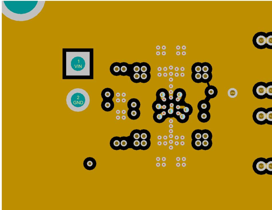
GND plane kept intact under the high current traces to provide shortest possible return path for high frequencies.
