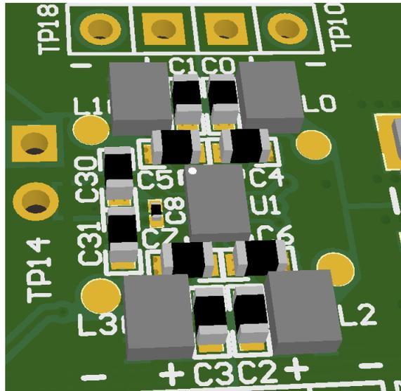
Figure 14. 3-D View Showing the LP8758-E0 Device and Nearest Components
