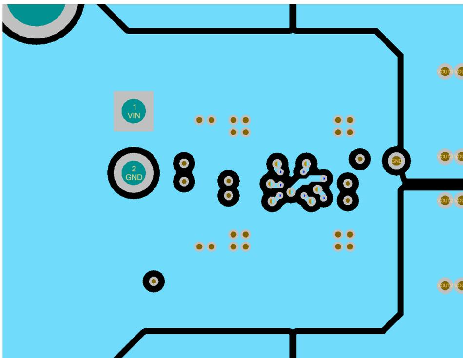
Plane kept intact around the LP8758-E0 device.
