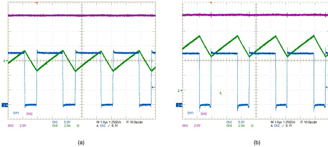
Figure 15. SW1, SW2,  $I_L$  Waveforms:  $V_{IN} = 18\text{ V}$ ,  $V_{OUT} = 12\text{ V}$ , (a)  $I_{OUT} = 0\text{ A}$ , (b)  $I_{OUT} = 6\text{ A}$
