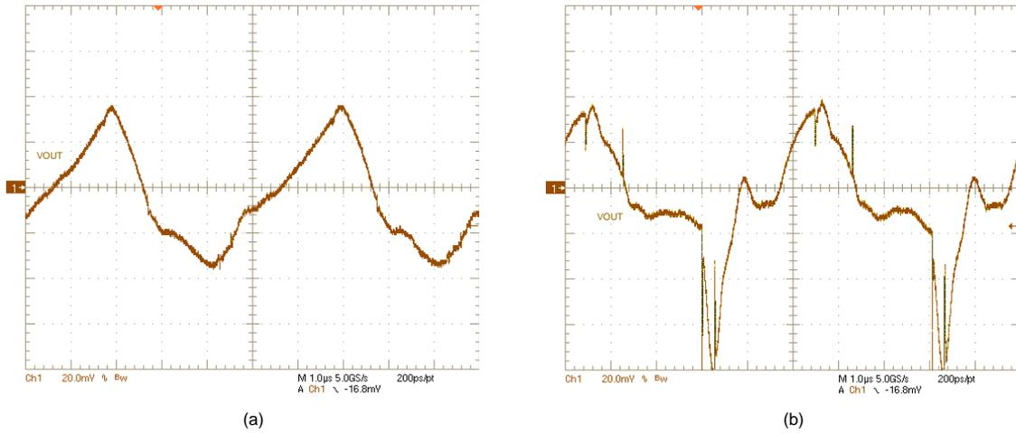
Figure 46.  $V_{OUT}$  ripple:  $V_{IN} = 14\text{ V}$ ,  $V_{OUT} = 12\text{ V}$ , (a)  $I_{OUT} = 0\text{ A}$ , (b)  $I_{OUT} = 6\text{ A}$
