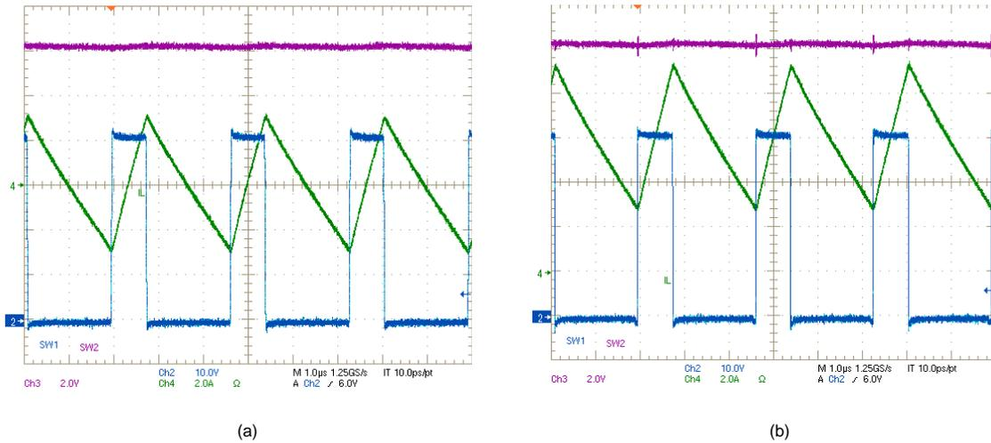
Figure 18. SW1, SW2,  $I_L$  Waveforms:  $V_{IN} = 42\text{ V}$ ,  $V_{OUT} = 12\text{ V}$ , (a)  $I_{OUT} = 0\text{ A}$ , (b)  $I_{OUT} = 6\text{ A}$
