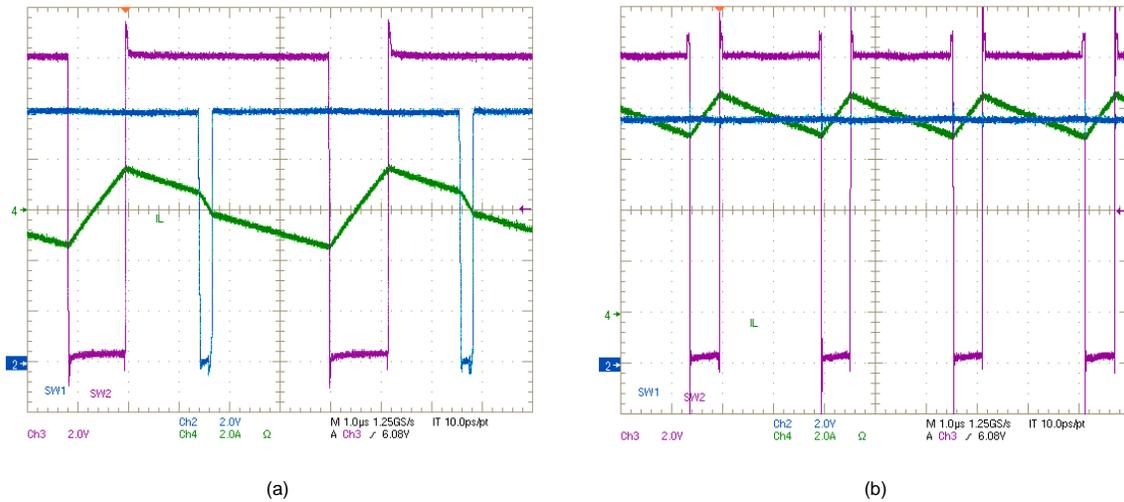
Figure 11. SW1, SW2,  $I_L$  Waveforms:  $V_{IN} = 10\text{ V}$ ,  $V_{OUT} = 12\text{ V}$ , (a)  $I_{OUT} = 0\text{ A}$ , (b)  $I_{OUT} = 6\text{ A}$
