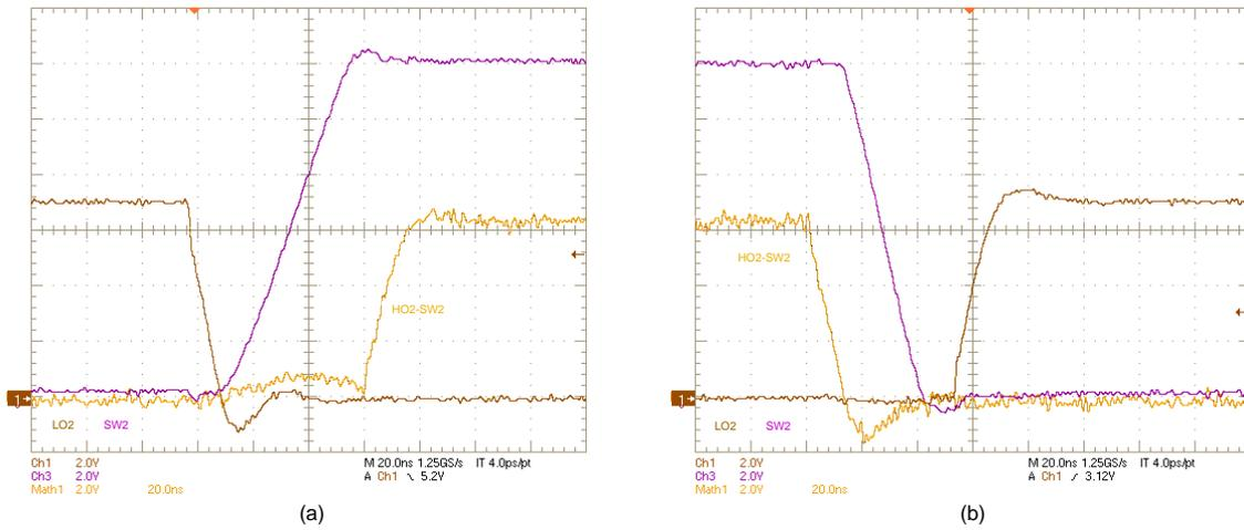
Figure 37. SW2, LO2, (HO2-SW2) Voltages:  $V_{IN} = 14\text{ V}$ ,  $V_{OUT} = 12\text{ V}$ ,  $I_{OUT} = 0\text{ A}$ , (a) OFF, (b) ON
