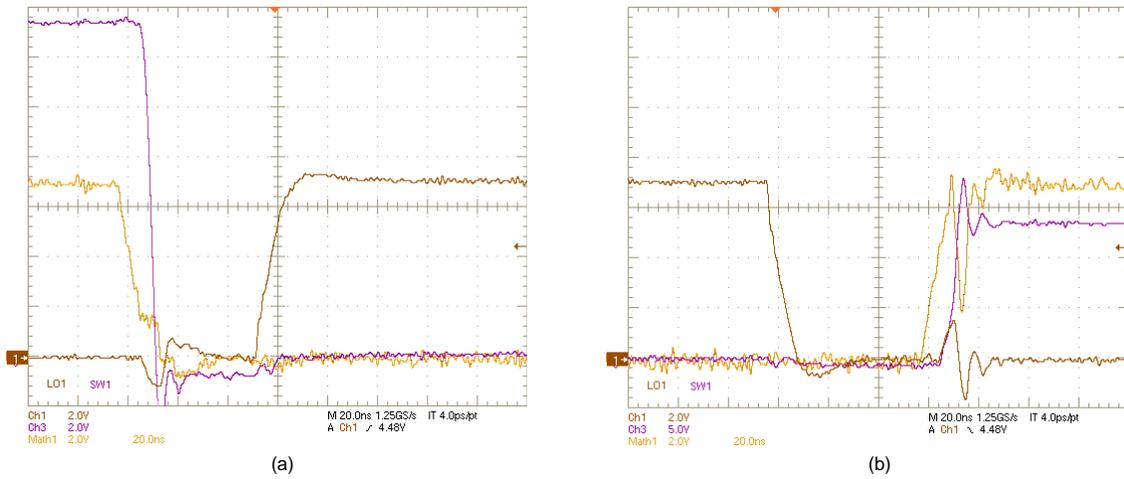
Figure 28. SW1, LO1, (HO1–SW1) Voltages:  $V_{IN} = 14\text{ V}$ ,  $V_{OUT} = 12\text{ V}$ ,  $I_{OUT} = 6\text{ A}$ , (a) OFF, (b) ON
