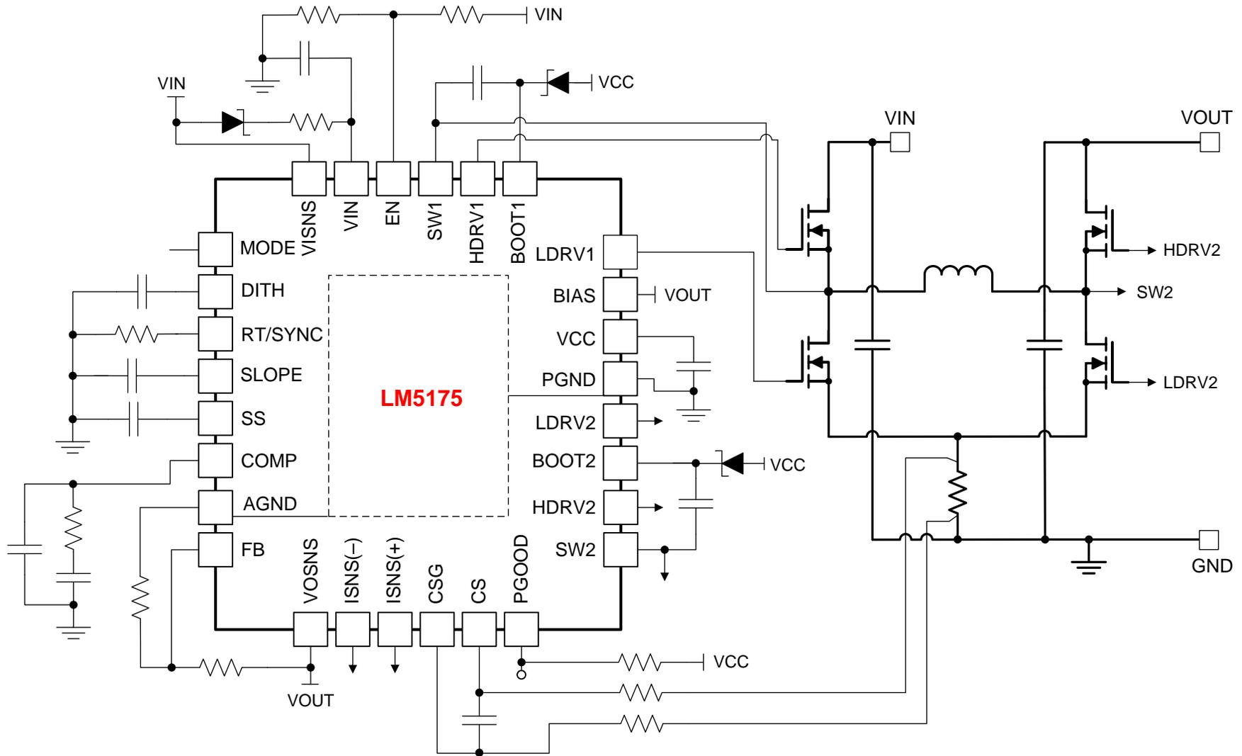
Figure 1. LM5175 Buck-boost Converter Circuit Diagram
