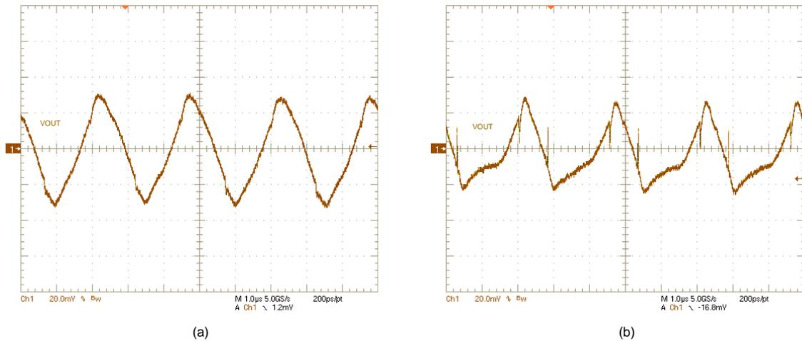
Figure 48.  $V_{OUT}$  ripple:  $V_{IN} = 24\text{ V}$ ,  $V_{OUT} = 12\text{ V}$ , (a)  $I_{OUT} = 0\text{ A}$ , (b)  $I_{OUT} = 6\text{ A}$
