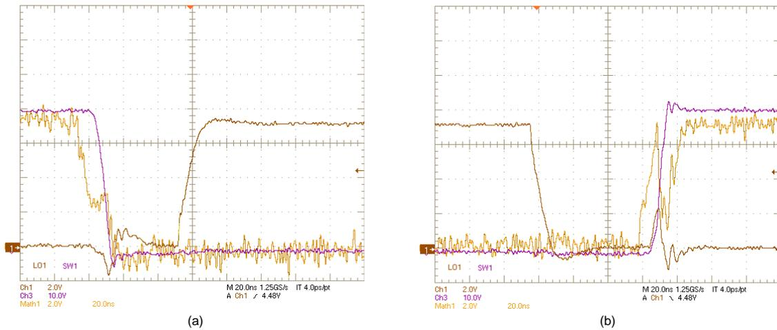
Figure 32. SW1, LO1, (HO1–SW1) Voltages:  $V_{IN} = 42\text{ V}$ ,  $V_{OUT} = 12\text{ V}$ ,  $I_{OUT} = 6\text{ A}$ , (a) OFF, (b) ON
