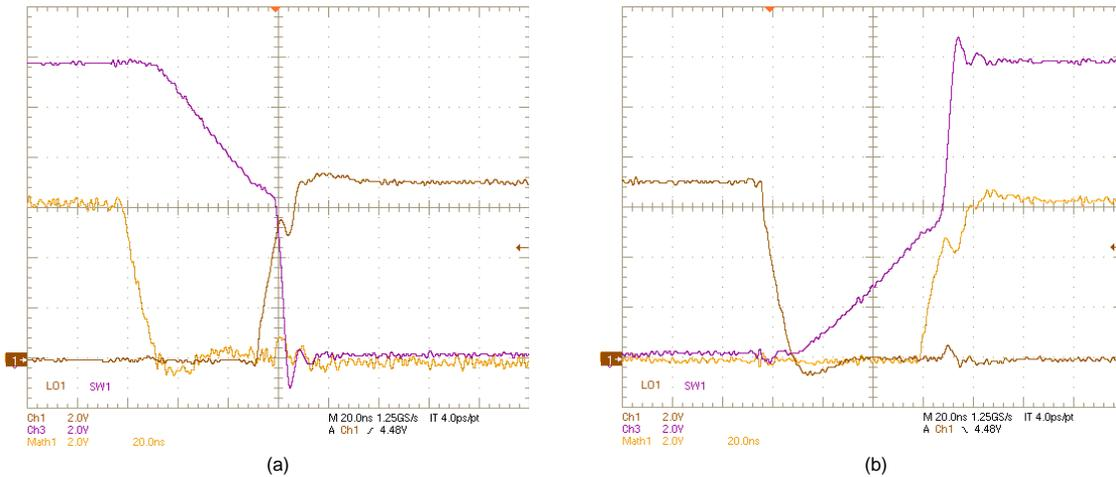
Figure 20. SW1, LO1, (HO1–SW1) Voltages:  $V_{IN} = 12\text{ V}$ ,  $V_{OUT} = 12\text{ V}$ ,  $I_{OUT} = 0\text{ A}$ , (a) OFF, (b) ON
