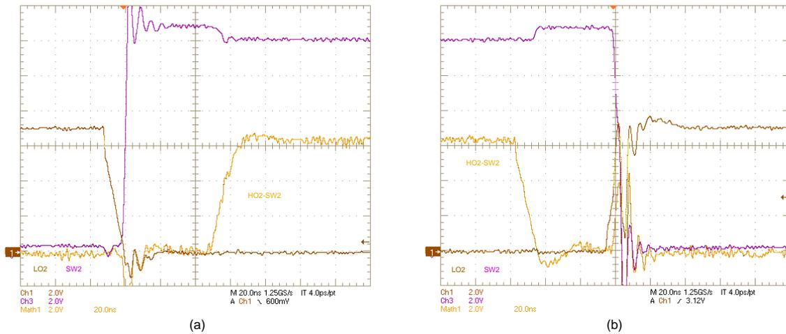
Figure 41. SW2, LO2, (HO2-SW2) Voltages:  $V_{IN} = 12\text{ V}$ ,  $V_{OUT} = 12\text{ V}$ ,  $I_{OUT} = 6\text{ A}$ , (a) OFF, (b) ON
