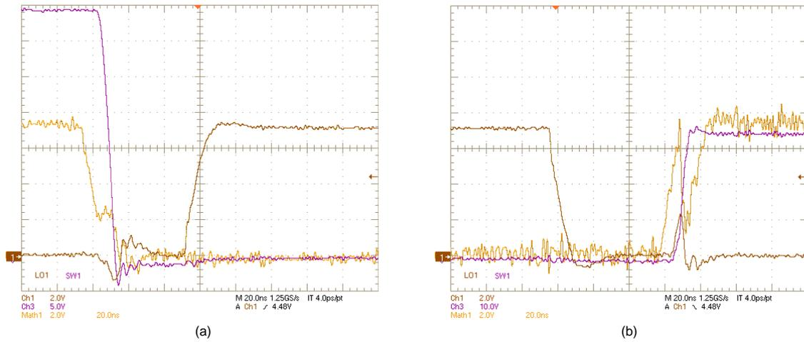
Figure 31. SW1, LO1, (HO1–SW1) Voltages:  $V_{IN} = 36\text{ V}$ ,  $V_{OUT} = 12\text{ V}$ ,  $I_{OUT} = 6\text{ A}$ , (a) OFF, (b) ON
