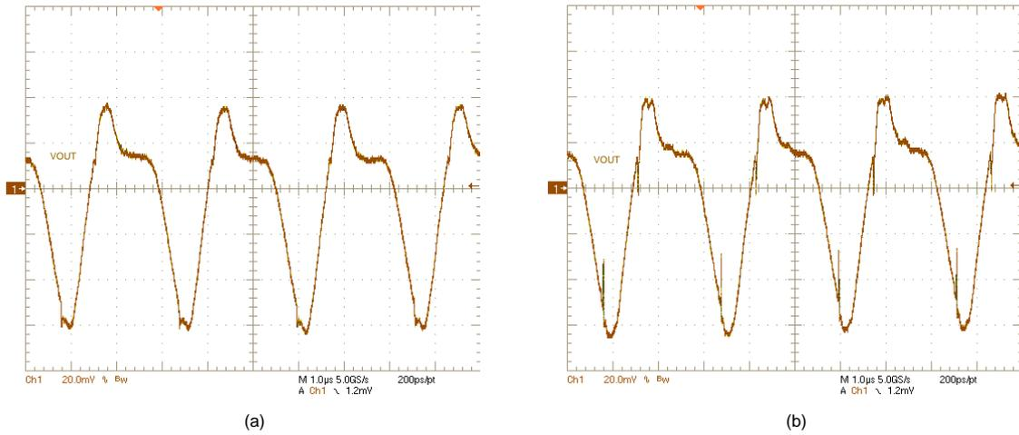
Figure 50.  $V_{OUT}$  ripple:  $V_{IN} = 42\text{ V}$ ,  $V_{OUT} = 12\text{ V}$ , (a)  $I_{OUT} = 0\text{ A}$ , (b)  $I_{OUT} = 6\text{ A}$
