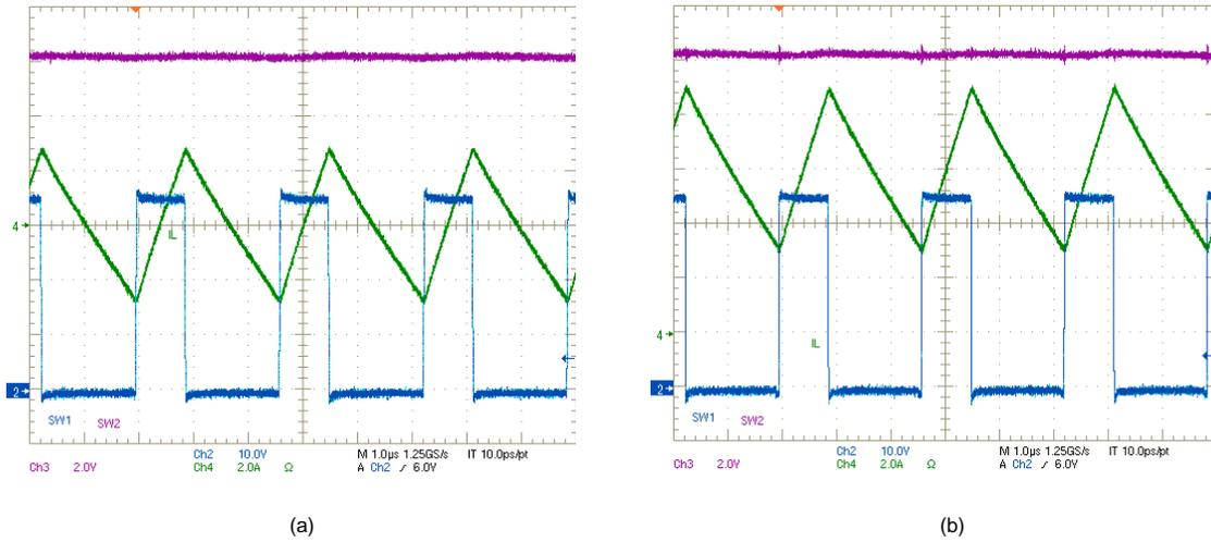
Figure 17. SW1, SW2,  $I_L$  Waveforms:  $V_{IN} = 36\text{ V}$ ,  $V_{OUT} = 12\text{ V}$ , (a)  $I_{OUT} = 0\text{ A}$ , (b)  $I_{OUT} = 6\text{ A}$
