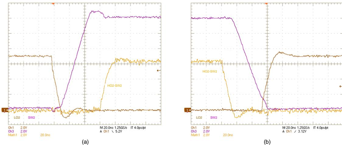
Figure 36. SW2, LO2, (HO2–SW2) Voltages:  $V_{IN} = 12\text{ V}$ ,  $V_{OUT} = 12\text{ V}$ ,  $I_{OUT} = 0\text{ A}$ , (a) OFF, (b) ON
