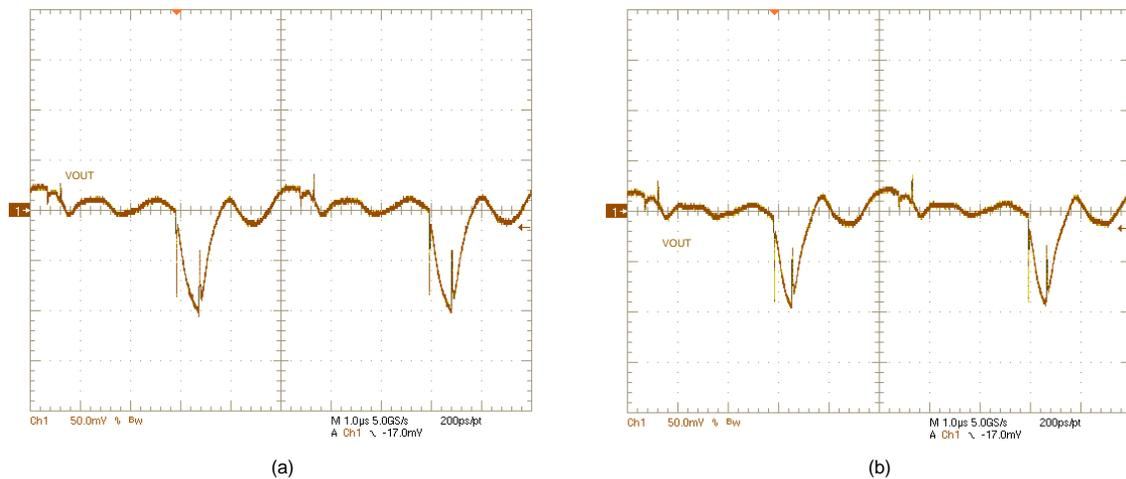
Figure 45.  $V_{OUT}$  ripple:  $V_{IN} = 12\text{ V}$ ,  $V_{OUT} = 12\text{ V}$ , (a)  $I_{OUT} = 0\text{ A}$ , (b)  $I_{OUT} = 6\text{ A}$
