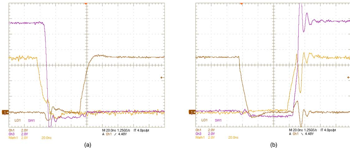
**Figure 27. SW1, LO1, (HO1–SW1) Voltages:  $V_{IN} = 12\text{ V}$ ,  $V_{OUT} = 12\text{ V}$ ,  $I_{OUT} = 6\text{ A}$ , (a) OFF, (b) ON**
