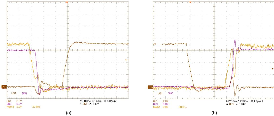
Figure 29. SW1, LO1, (HO1–SW1) Voltages:  $V_{IN} = 16\text{ V}$ ,  $V_{OUT} = 12\text{ V}$ ,  $I_{OUT} = 6\text{ A}$ , (a) OFF, (b) ON
