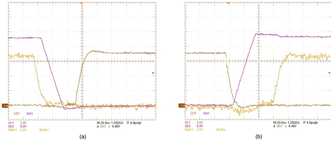
Figure 23. SW1, LO1, (HO1-SW1) Voltages:  $V_{IN} = 24\text{ V}$ ,  $V_{OUT} = 12\text{ V}$ ,  $I_{OUT} = 0\text{ A}$ , (a) OFF, (b) ON
