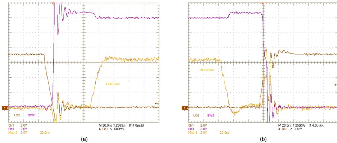
Figure 38. SW2, LO2, (HO2-SW2) Voltages:  $V_{IN} = 6\text{ V}$ ,  $V_{OUT} = 12\text{ V}$ ,  $I_{OUT} = 6\text{ A}$ , (a) OFF, (b) ON
