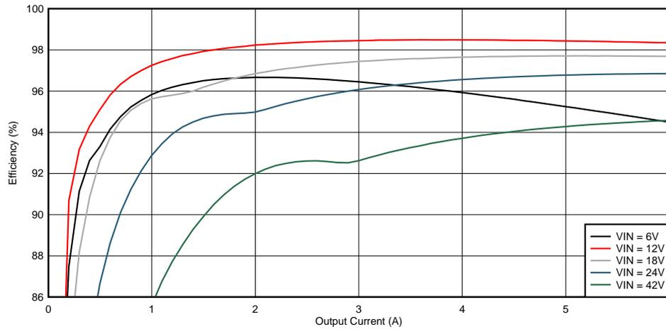
Figure 5. Efficiency vs. Output Current
