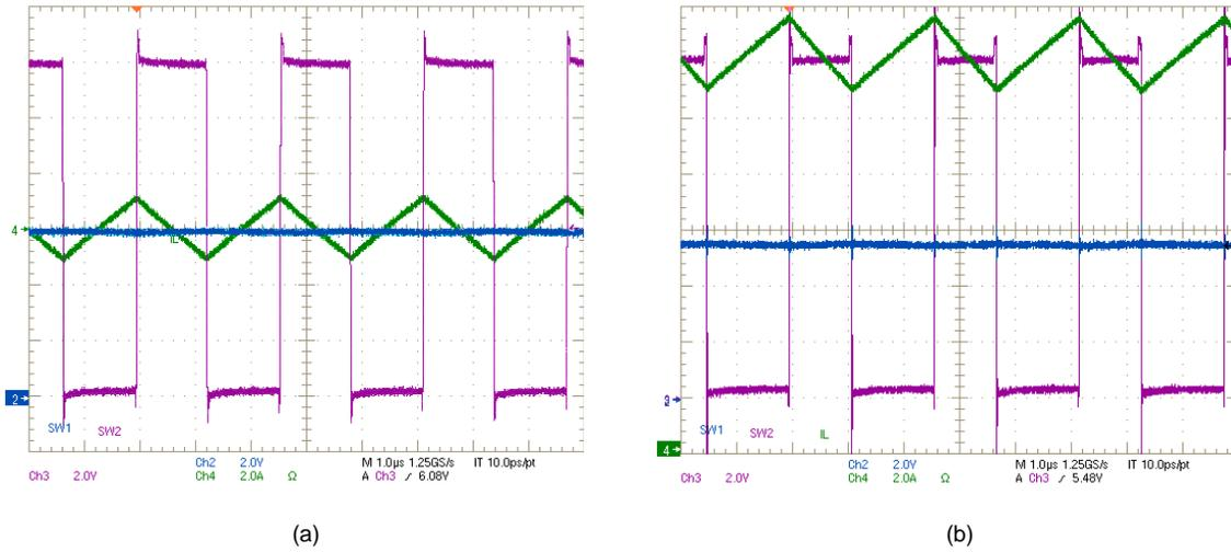
Figure 9. SW1, SW2,  $I_L$  Waveforms:  $V_{IN} = 6\text{ V}$ ,  $V_{OUT} = 12\text{ V}$ , (a)  $I_{OUT} = 0\text{ A}$ , (b)  $I_{OUT} = 6\text{ A}$
