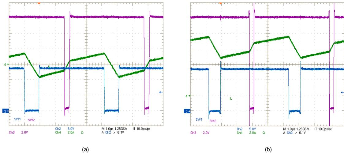
Figure 13. SW1, SW2,  $I_L$  Waveforms:  $V_{IN} = 14\text{ V}$ ,  $V_{OUT} = 12\text{ V}$ , (a)  $I_{OUT} = 0\text{ A}$ , (b)  $I_{OUT} = 6\text{ A}$
