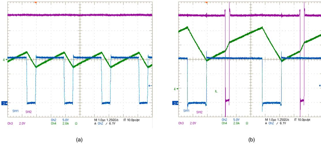
Figure 14. SW1, SW2,  $I_L$  Waveforms:  $V_{IN} = 16\text{ V}$ ,  $V_{OUT} = 12\text{ V}$ , (a)  $I_{OUT} = 0\text{ A}$ , (b)  $I_{OUT} = 6\text{ A}$
