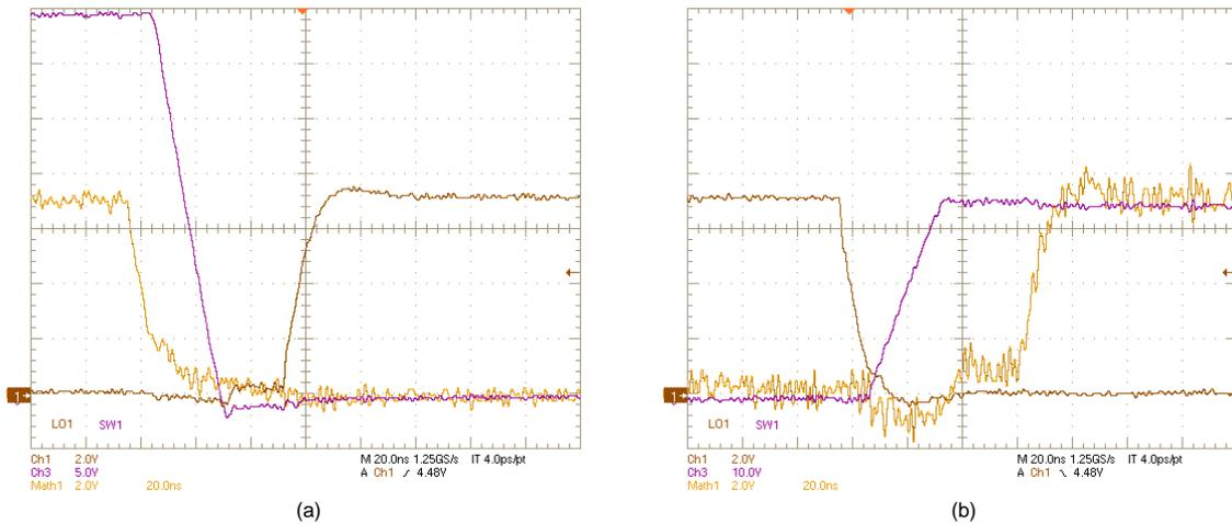
Figure 24. SW1, LO1, (HO1-SW1) Voltages:  $V_{IN} = 36\text{ V}$ ,  $V_{OUT} = 12\text{ V}$ ,  $I_{OUT} = 0\text{ A}$ , (a) OFF, (b) ON
