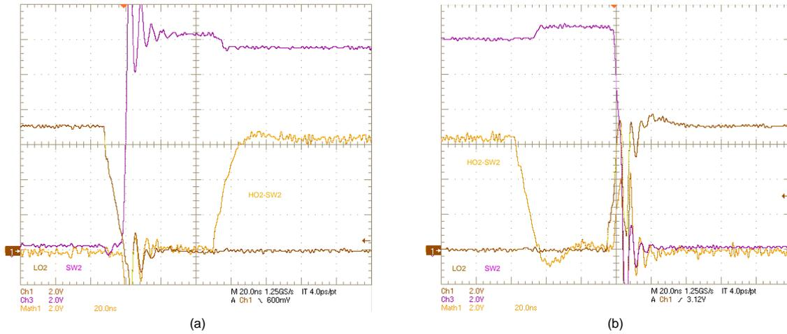
Figure 40. SW2, LO2, (HO2-SW2) Voltages:  $V_{IN} = 10\text{ V}$ ,  $V_{OUT} = 12\text{ V}$ ,  $I_{OUT} = 6\text{ A}$ , (a) OFF, (b) ON
