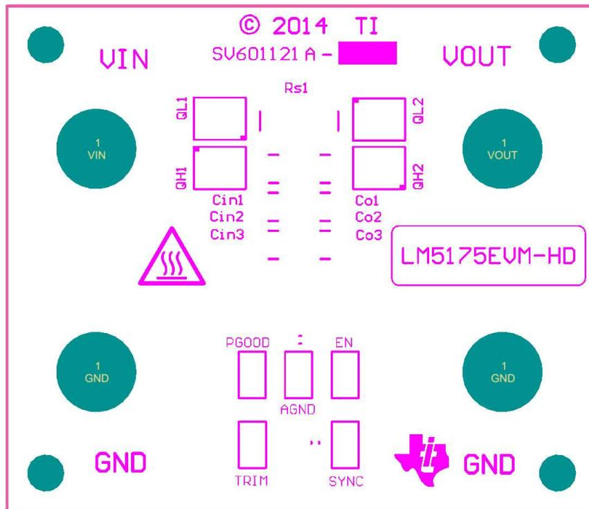
Figure 58. Top Layer Silkscreen (Top view)
