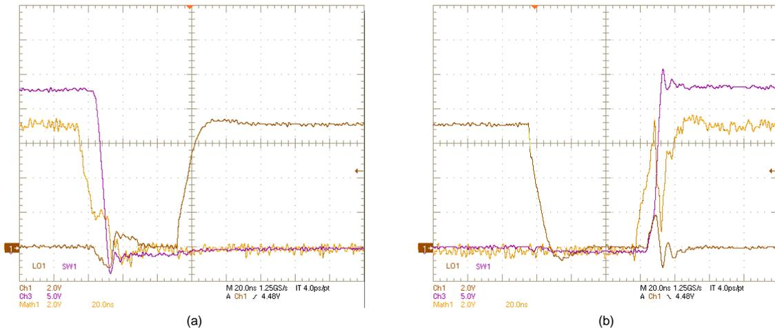
Figure 30. SW1, LO1, (HO1–SW1) Voltages:  $V_{IN} = 24\text{ V}$ ,  $V_{OUT} = 12\text{ V}$ ,  $I_{OUT} = 6\text{ A}$ , (a) OFF, (b) ON
