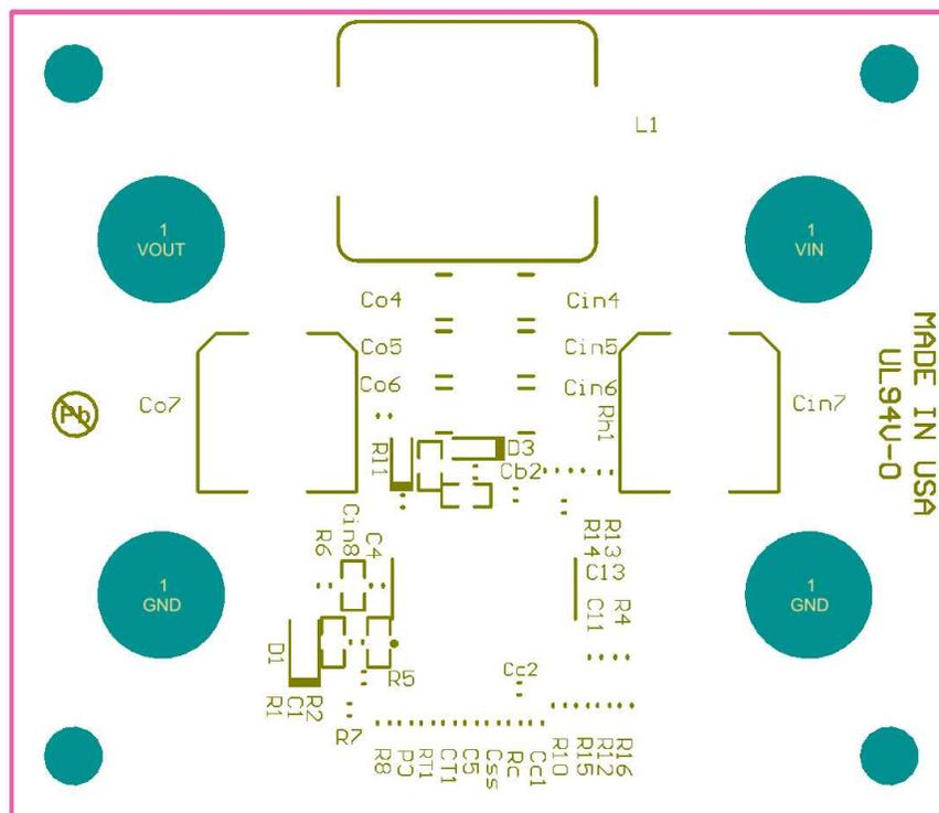
Figure 59. Bottom Layer Silkscreen (Bottom view)
