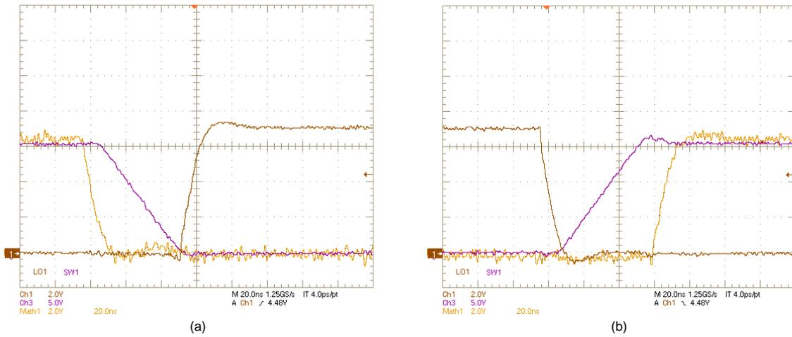
Figure 22. SW1, LO1, (HO1-SW1) Voltages:  $V_{IN} = 16\text{ V}$ ,  $V_{OUT} = 12\text{ V}$ ,  $I_{OUT} = 0\text{ A}$ , (a) OFF, (b) ON
