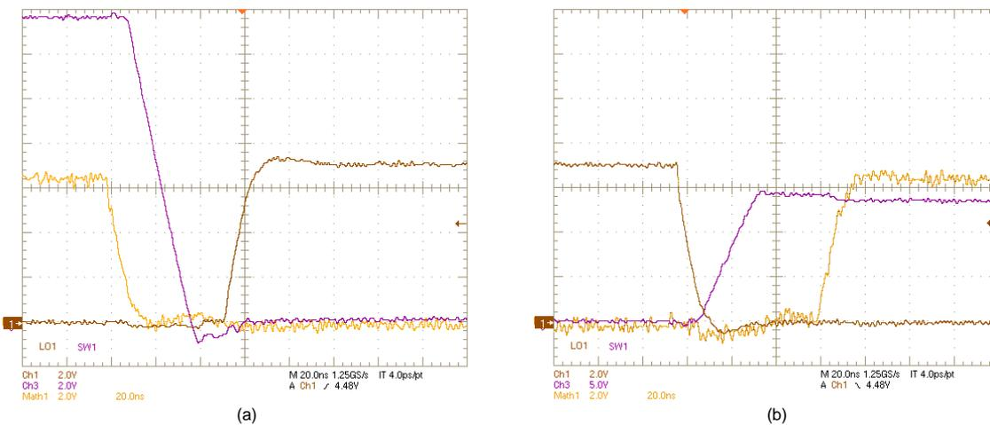
Figure 21. SW1, LO1, (HO1–SW1) Voltages:  $V_{IN} = 14\text{ V}$ ,  $V_{OUT} = 12\text{ V}$ ,  $I_{OUT} = 0\text{ A}$ , (a) OFF, (b) ON
