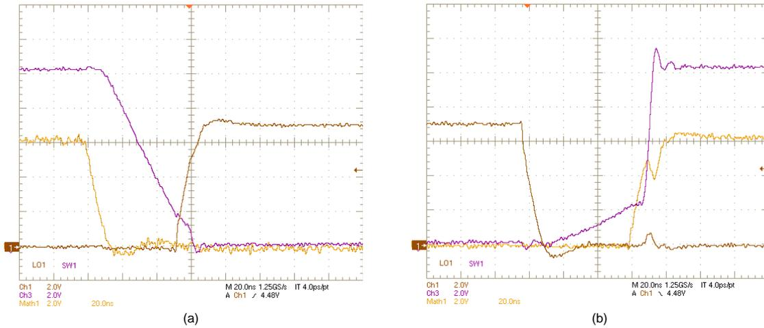
Figure 19. SW1, LO1, (HO1–SW1) Voltages:  $V_{IN} = 10.5\text{ V}$ ,  $V_{OUT} = 12\text{ V}$ ,  $I_{OUT} = 0\text{ A}$ , (a) OFF, (b) ON
