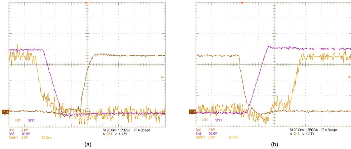
**Figure 25. SW1, LO1, (HO1–SW1) Voltages:  $V_{IN} = 42\text{ V}$ ,  $V_{OUT} = 12\text{ V}$ ,  $I_{OUT} = 0\text{ A}$ , (a) OFF, (b) ON**
