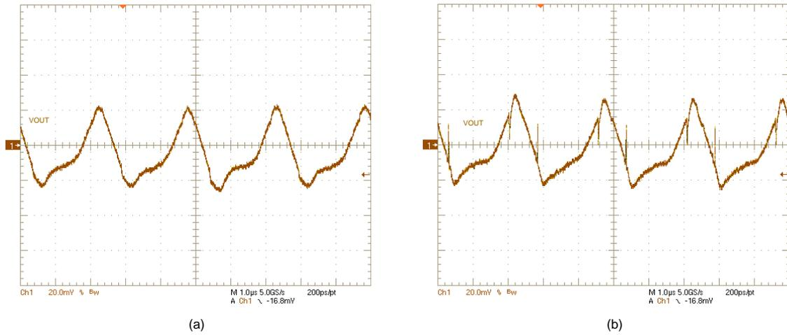
Figure 47.  $V_{OUT}$  ripple:  $V_{IN} = 18\text{ V}$ ,  $V_{OUT} = 12\text{ V}$ , (a)  $I_{OUT} = 0\text{ A}$ , (b)  $I_{OUT} = 6\text{ A}$
