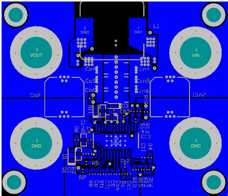
Figure 57. Bottom Copper (Bottom view)
