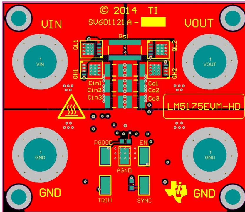
Figure 52. Top Copper (Top view)
