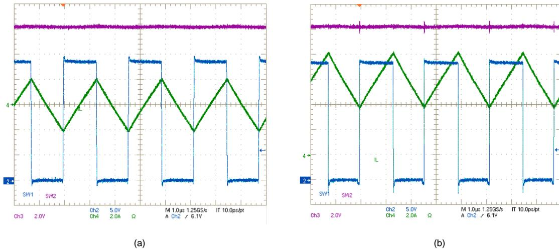
Figure 16. SW1, SW2,  $I_L$  Waveforms:  $V_{IN} = 24\text{ V}$ ,  $V_{OUT} = 12\text{ V}$ , (a)  $I_{OUT} = 0\text{ A}$ , (b)  $I_{OUT} = 6\text{ A}$
