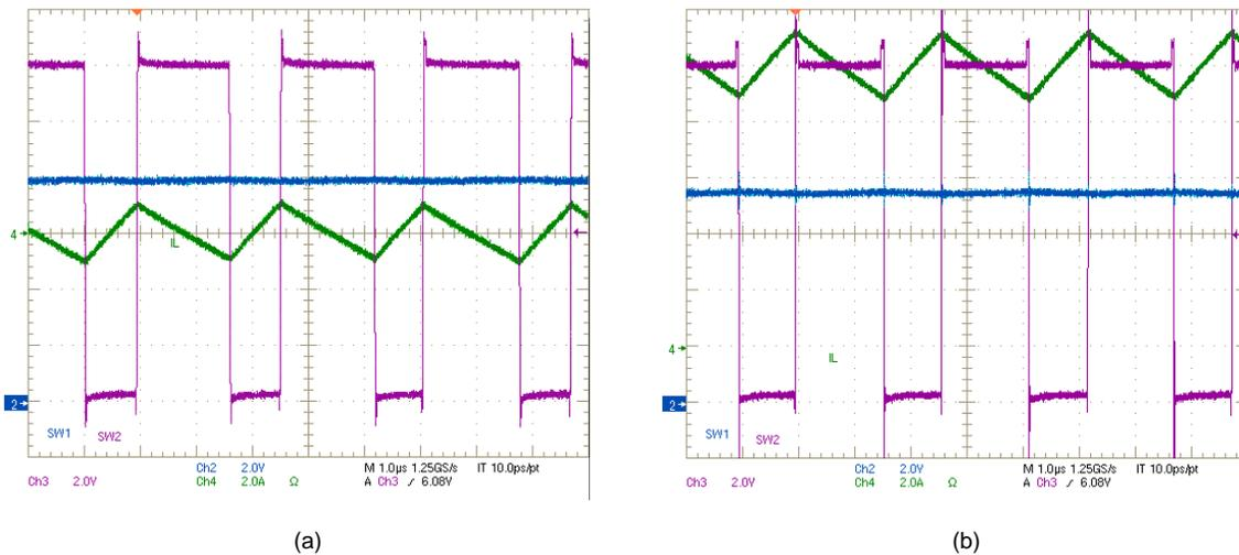
Figure 10. SW1, SW2,  $I_L$  Waveforms:  $V_{IN} = 8\text{ V}$ ,  $V_{OUT} = 12\text{ V}$ , (a)  $I_{OUT} = 0\text{ A}$ , (b)  $I_{OUT} = 6\text{ A}$
