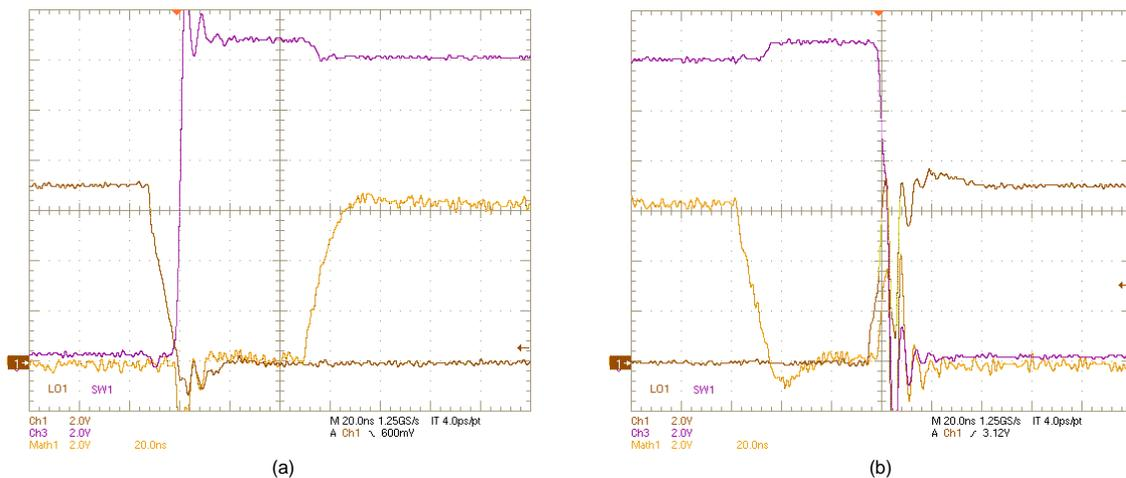
Figure 42. SW2, LO2, (HO2-SW2) Voltages:  $V_{IN} = 14\text{ V}$ ,  $V_{OUT} = 12\text{ V}$ ,  $I_{OUT} = 6\text{ A}$ , (a) OFF, (b) ON
