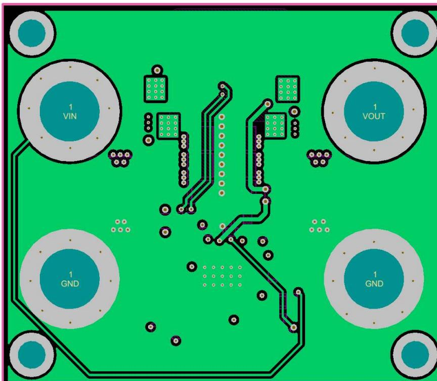
Figure 55. Layer 4 (Top view)
