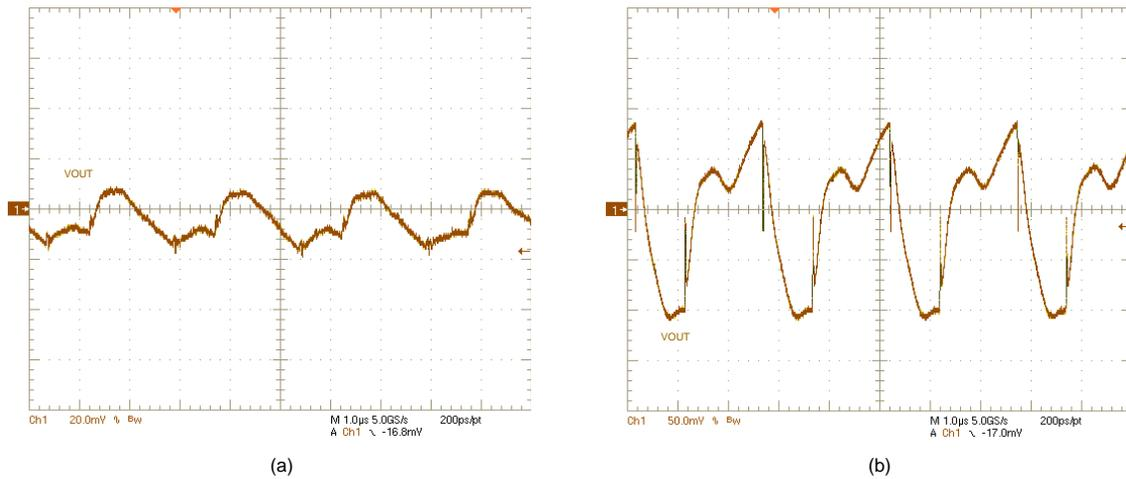
Figure 44.  $V_{OUT}$  ripple:  $V_{IN} = 8\text{ V}$ ,  $V_{OUT} = 12\text{ V}$ , (a)  $I_{OUT} = 0\text{ A}$ , (b)  $I_{OUT} = 6\text{ A}$
