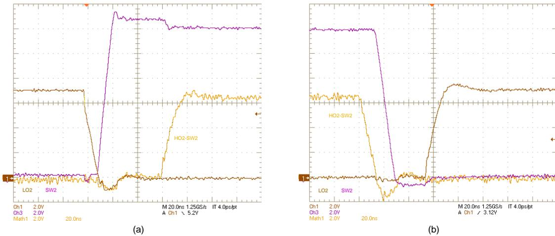
Figure 35. SW2, LO2, (HO2–SW2) Voltages:  $V_{IN} = 10\text{ V}$ ,  $V_{OUT} = 12\text{ V}$ ,  $I_{OUT} = 0\text{ A}$ , (a) OFF, (b) ON
