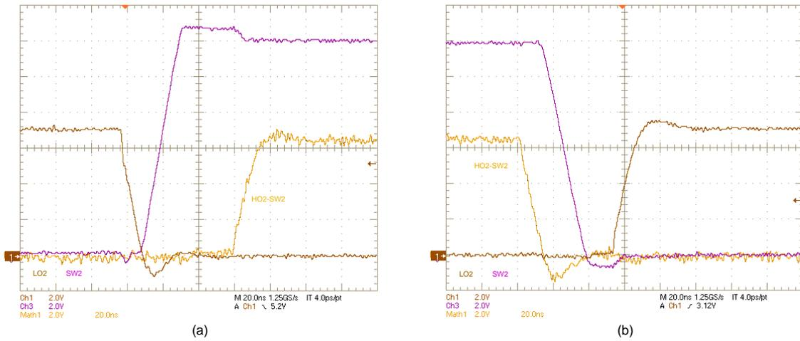
Figure 34. SW2, LO2, (HO2–SW2) Voltages:  $V_{IN} = 8\text{ V}$ ,  $V_{OUT} = 12\text{ V}$ ,  $I_{OUT} = 0\text{ A}$ , (a) OFF, (b) ON
