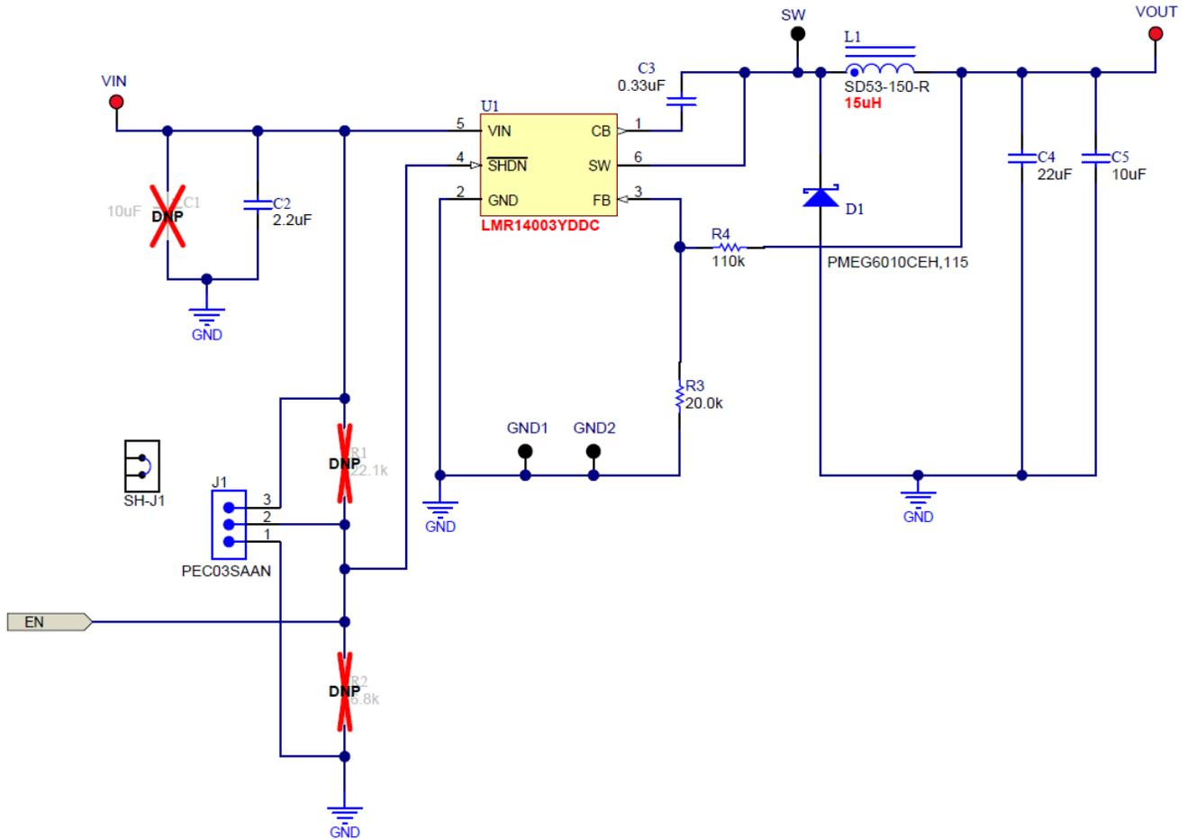
Figure 5. LMR14006YEVM Schematic
