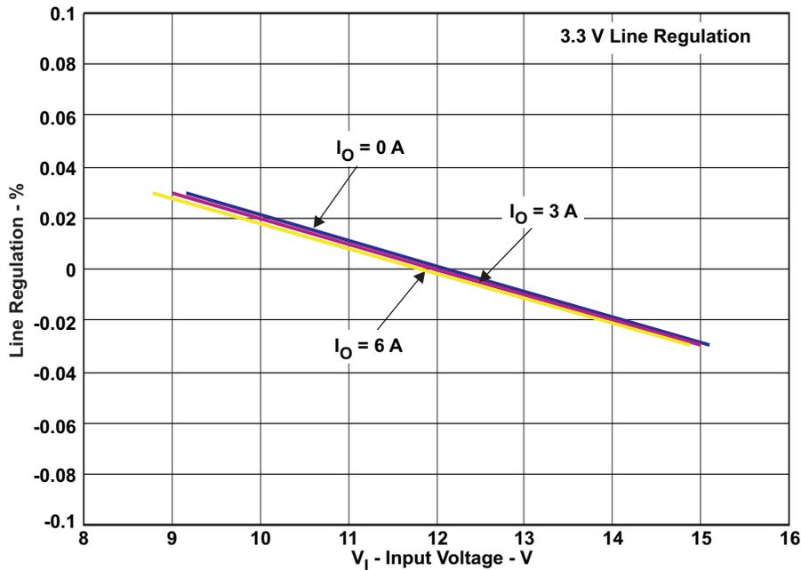
Figure 7. Line Regulation at 25°C
