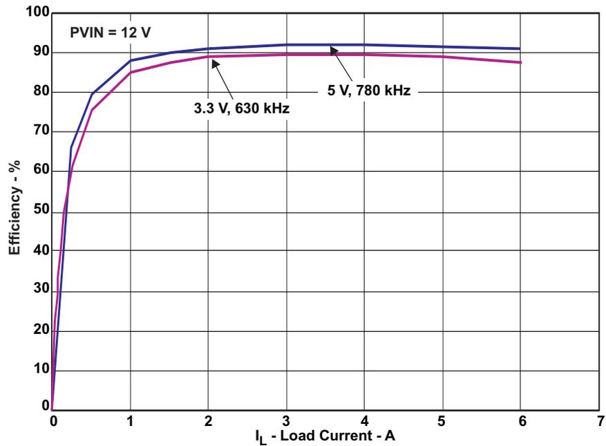
Figure 4. Efficiency vs Output Voltage at 25°C
