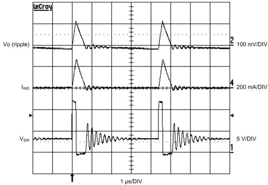
Trace 2 = V<sub>OUT</sub> ripple (ac coupled)
