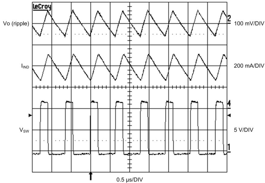
Trace 2 = V<sub>OUT</sub> ripple (ac coupled)
