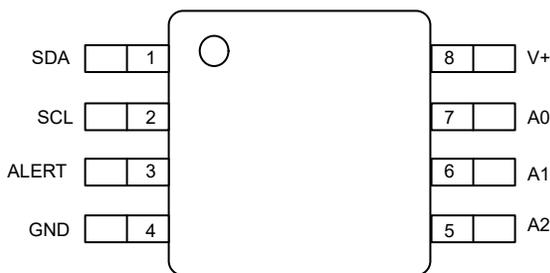
**Figure 4-1. 8-Pin VSSOP Top View**
