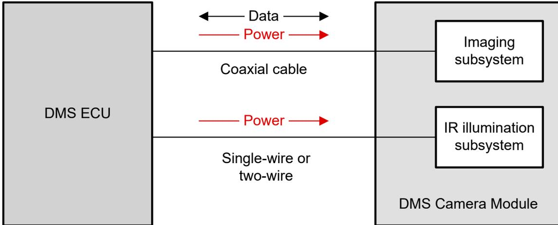
Figure 2-2. DMS ECU and Camera Dual Cable Implementation
