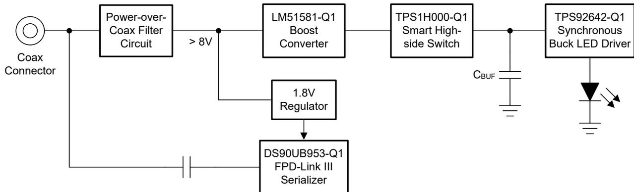
**Figure 3-1. Block Diagram of DMS Camera Module With Single Coax Connection**
