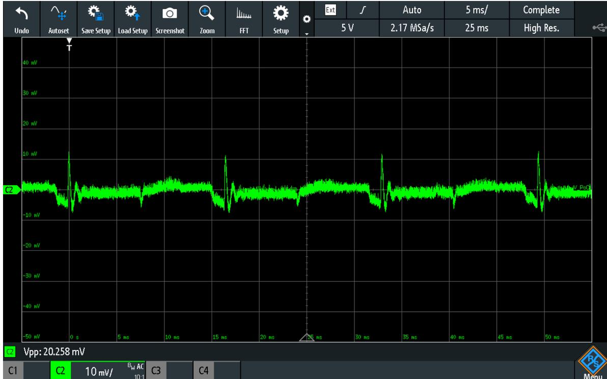
Figure 4-4. Differential Supply Noise
