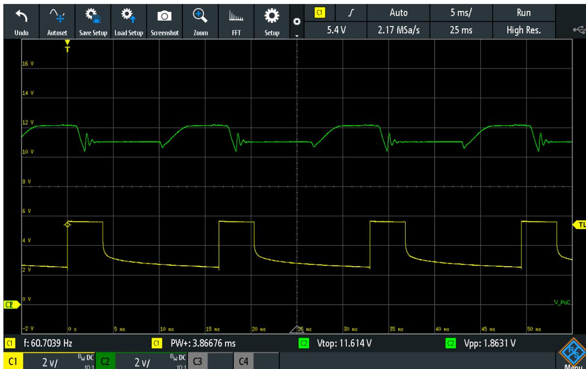
**Figure 4-1. LED and PoC Voltage Waveform**
