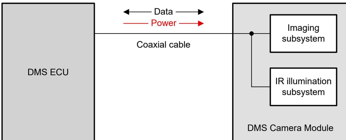
Figure 2-3. DMS ECU and Camera Single Cable Implementation
