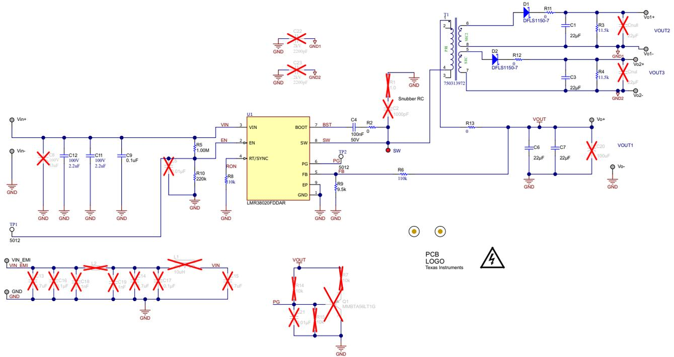
Figure 4-1. LMR38020 Fly-Buck Application Schematic for Micro Inverter
