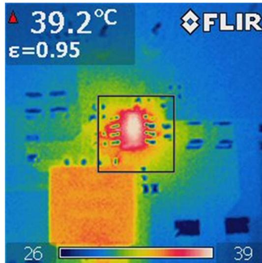
Figure 4-15. Thermal Performance When  $V_{IN} = 48\text{ V}$ , Full Load
