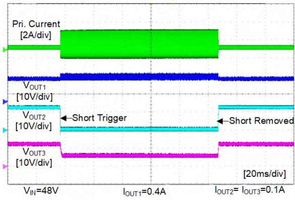
Figure 4-14. Short Circuit- Secondary Output
