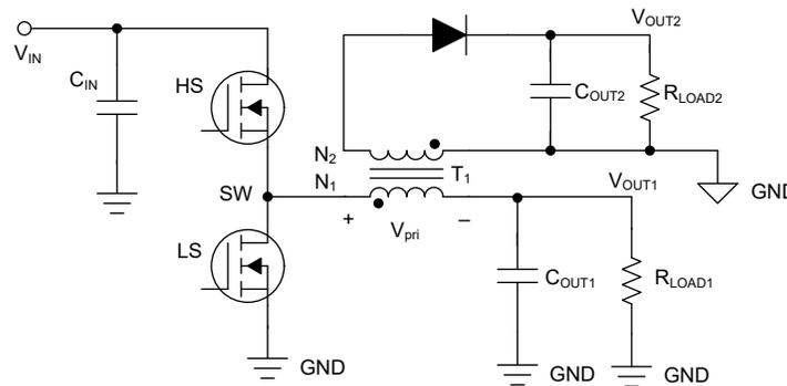
**Figure 3-1. Simplified Fly-Buck™ Circuit Schematic**
