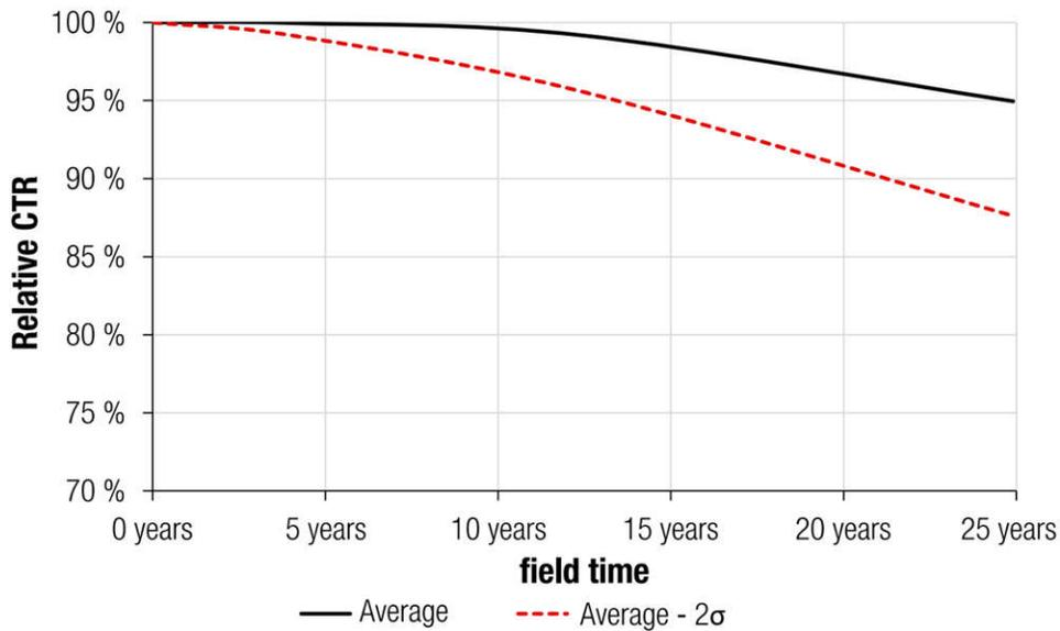
Figure 2-3. Optocouplers Expected CTR Degradation With Field Time
