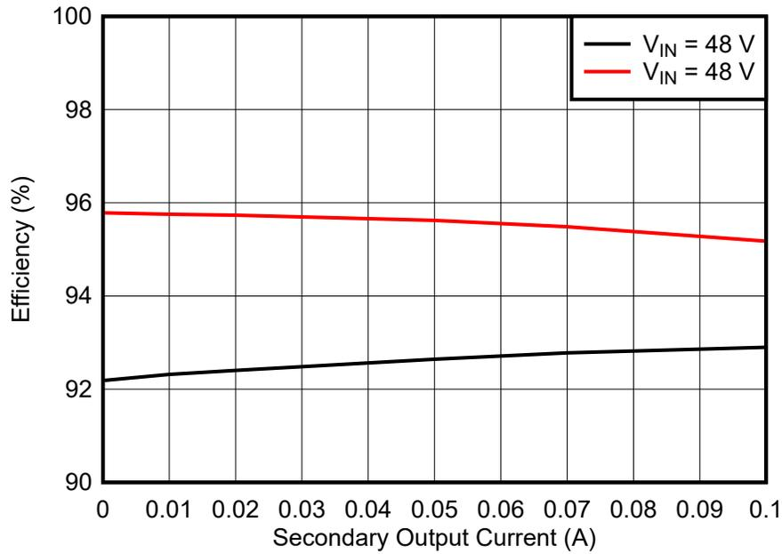
Figure 4-10. Efficiency: I<sub>OUT1</sub> = 0.4A
