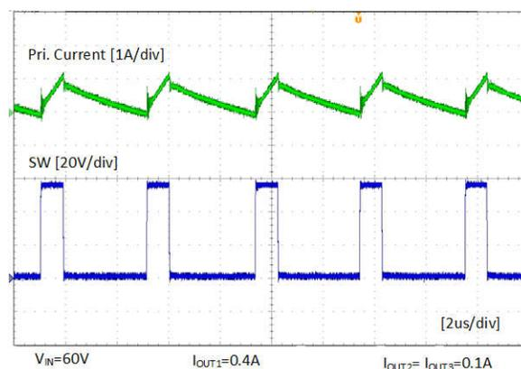
**Figure 4-6. Steady State When  $V_{IN} = 60\text{ V}$ ,  $I_{OUT1} = 0.4\text{ A}$ ,  $I_{OUT2} = I_{OUT3} = 0.1\text{ A}$**
