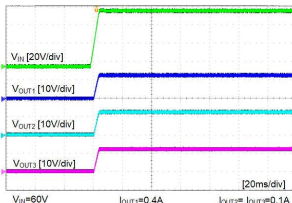
**Figure 4-4. Start Up, Full Load,  $V_{IN}=60\text{ V}$**
