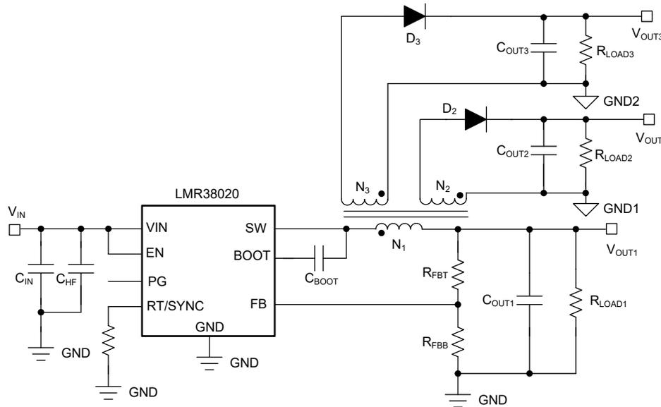
Figure 3-2. LMR38020 Fly-Buck Application Circuit Example
