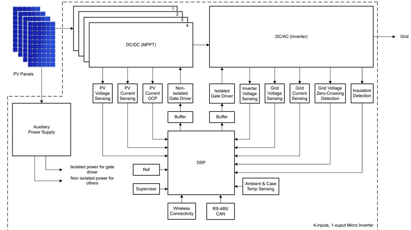
Figure 1-3. Block Diagram of Micro Inverter
