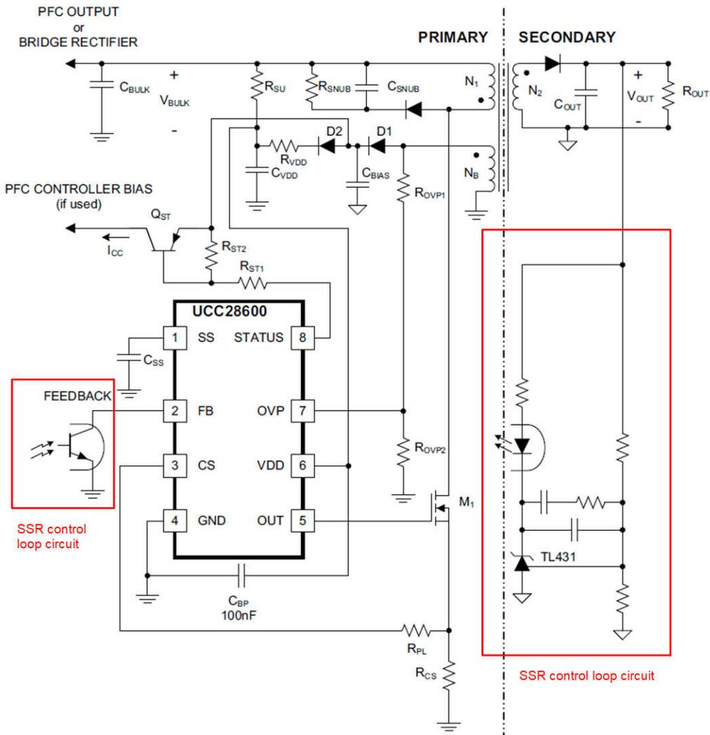
Figure 2-2. SSR Control Loop Example Circuit Based on UCC28600
