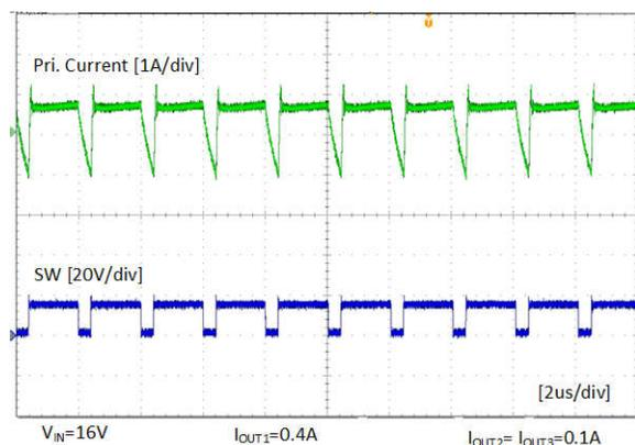
**Figure 4-5. Steady State When  $V_{IN} = 16\text{ V}$ ,  $I_{OUT1} = 0.4\text{ A}$ ,  $I_{OUT2} = I_{OUT3} = 0.1\text{ A}$**
