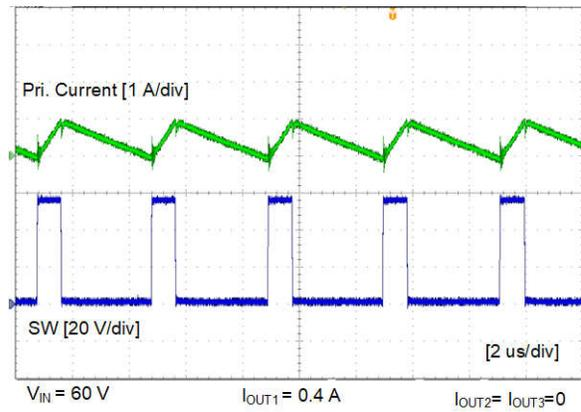
Figure 4-8. Steady State When  $V_{IN} = 60 V$ ,  $I_{OUT1} = 0.4 A$ ,  $I_{OUT2} = I_{OUT3} = 0 A$
