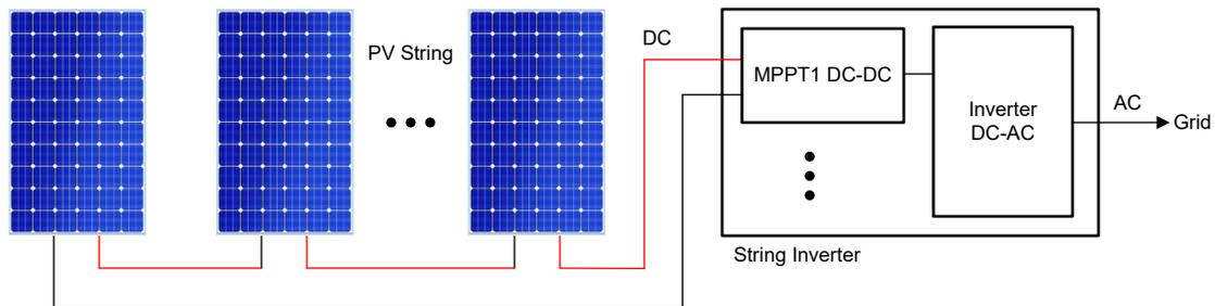
Figure 1-1. PV System Deployment with String Inverter
