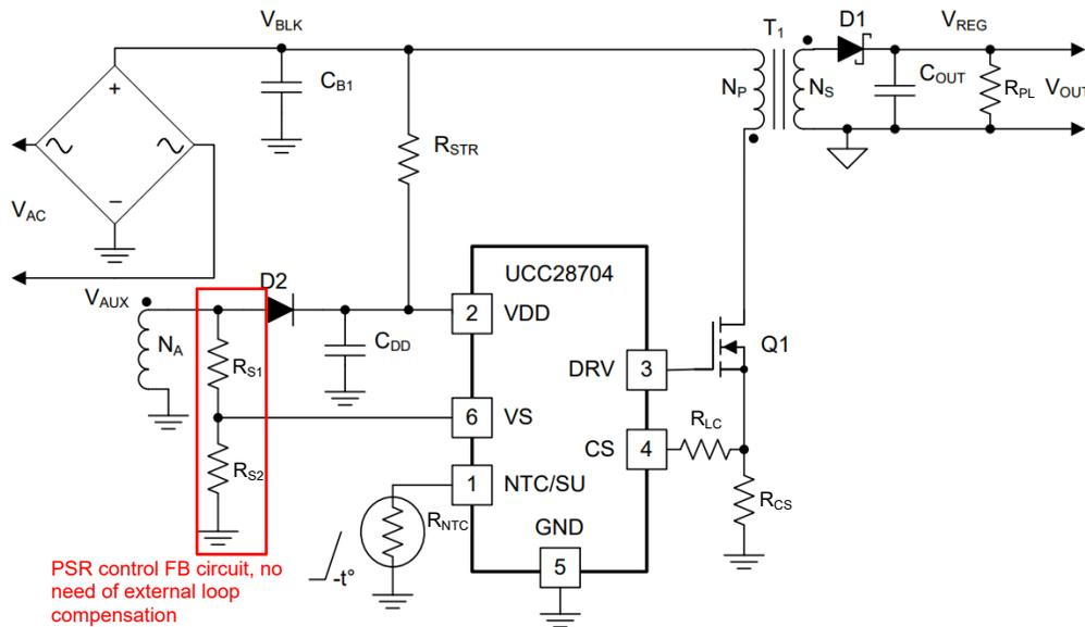
Figure 2-5. PSR Control Example Circuit Based on UCC28704
