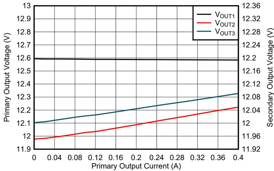
Figure 4-11. Load Regulation V.S. Primary Output Current: V<sub>IN</sub> = 48 V
