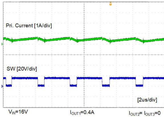
Figure 4-7. Steady State When  $V_{IN} = 16 V$ ,  $I_{OUT1} = 0.4 A$ ,  $I_{OUT2} = I_{OUT3} = 0 A$
