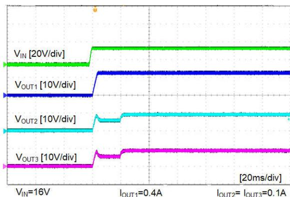
**Figure 4-3. Start Up, Full Load,  $V_{IN}=16\text{ V}$**
