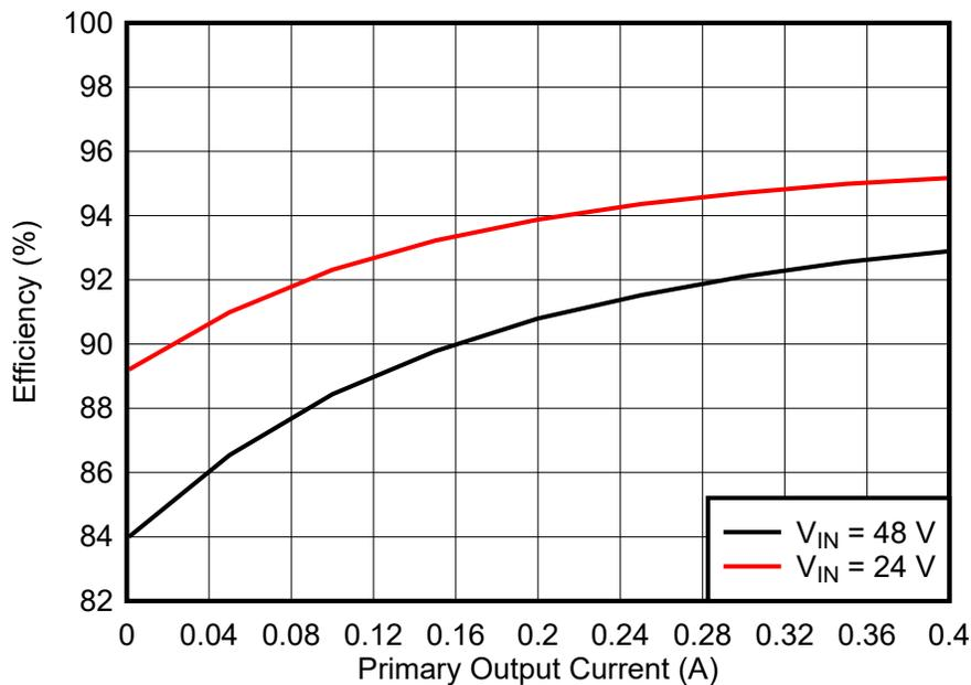
Figure 4-9. Efficiency:  $I_{OUT2} = I_{OUT3} = 0.1A$
