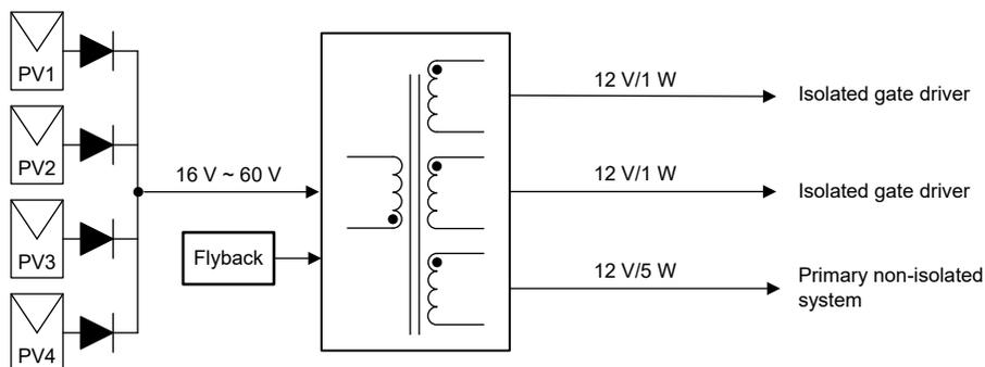
Figure 1-4. Typical Power Tree of Micro Inverters Auxiliary Power Supply
