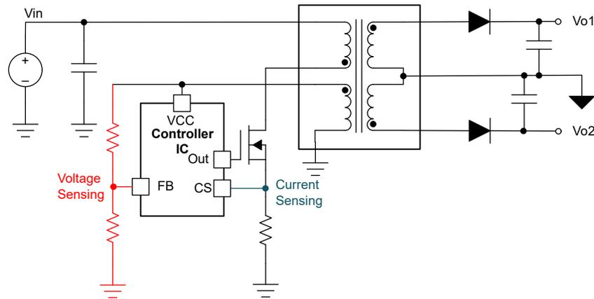
Figure 2-4. Simplified PSR Circuit Schematic
