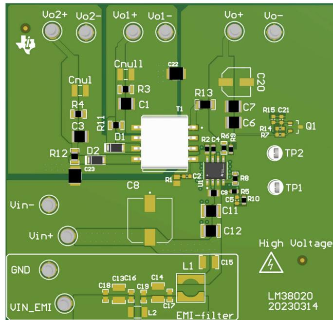
Figure 4-2. LMR38020 Fly-Buck Demo board for Micro Inverter
