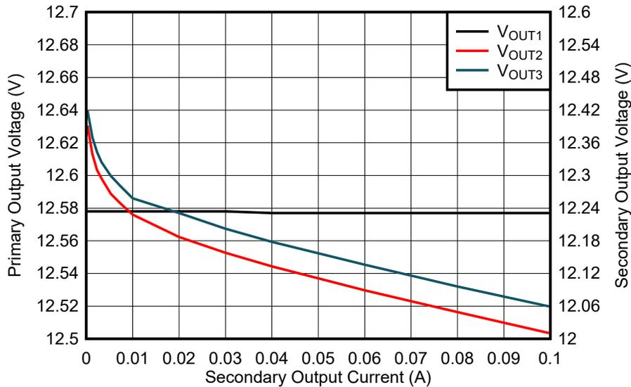
Figure 4-12. Load Regulation V.S. Secondary Output Current:  $V_{IN} = 48\text{ V}$
