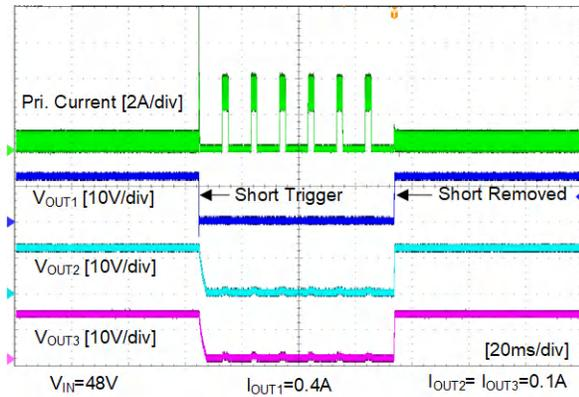
Figure 4-13. Short Circuit- Primary Output
