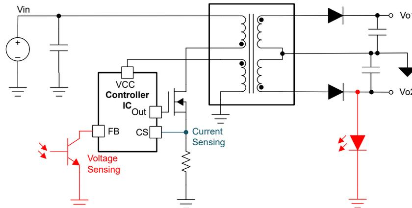
**Figure 2-1. Simplified SSR Control Schematic**
