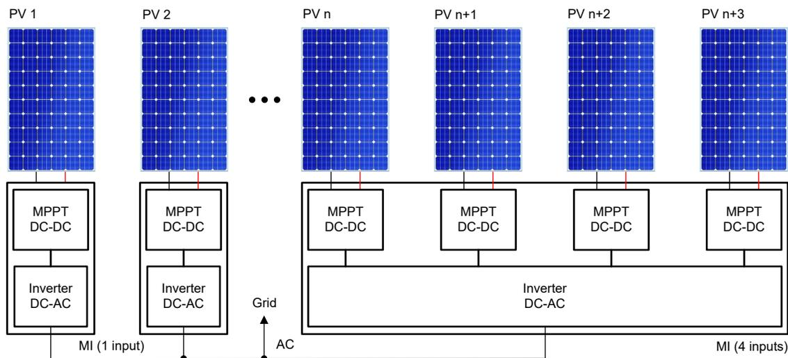
Figure 1-2. PV System Deployment with Micro Inverter
