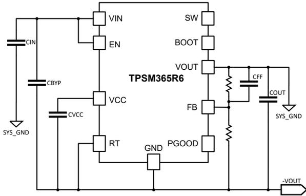
Figure 4-1. Basic Schematic Used
