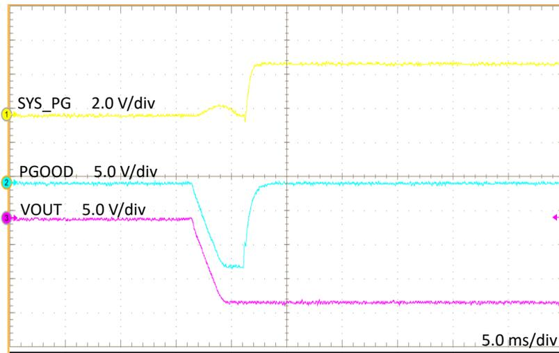
**Figure 5-5. PG Pin Level Shifter on Start-Up**
