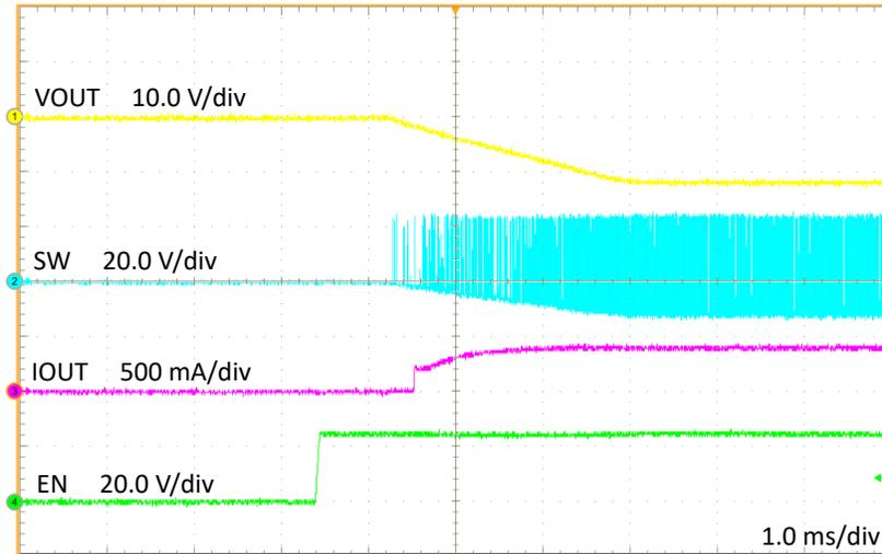
**Figure 2-3. SW Node Voltage During Start-Up**
