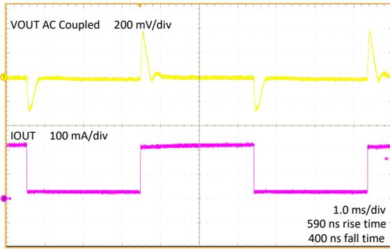
Figure 4-7. Load Transient Response, 100 mA to 410 mA With  $V_{IN} = 24\text{ V}$ ,  $V_{OUT} = -12\text{ V}$
