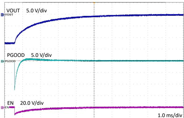
Figure 4-6. Shutdown on  $V_{IN} = 24$  V,  $V_{OUT} = -12$  V, Expected Performance With no Level Shifters
