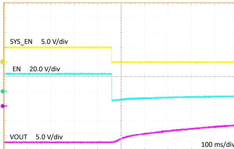
**Figure 5-3. EN Pin Level Shifter on Shutdown**
