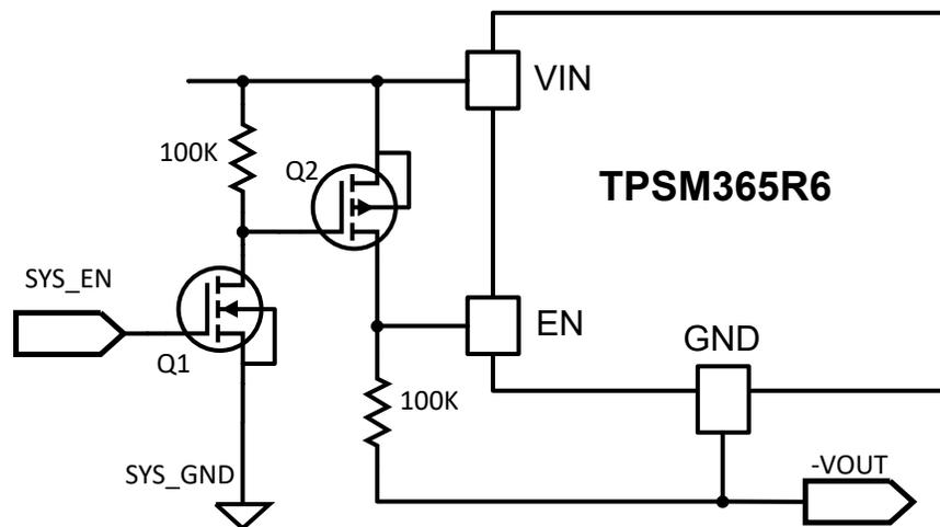
**Figure 5-1. EN Pin Level Shifter**
