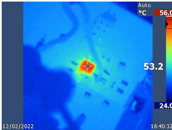
Figure 4-11. Temperature Response,  $V_{IN} = 24\text{ V}$ ,  $V_{OUT} = -5\text{ V}$ ,  $I_{OUT} = 450\text{ mA}$
