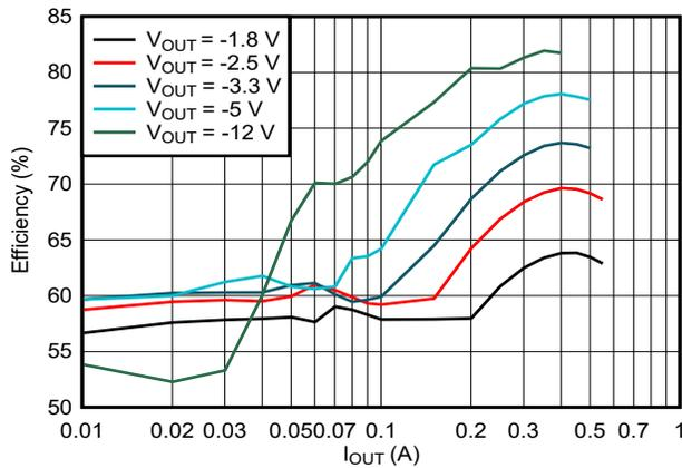
Figure 4-3. Efficiency vs. Load Current at  $V_{IN} = 24$  V
