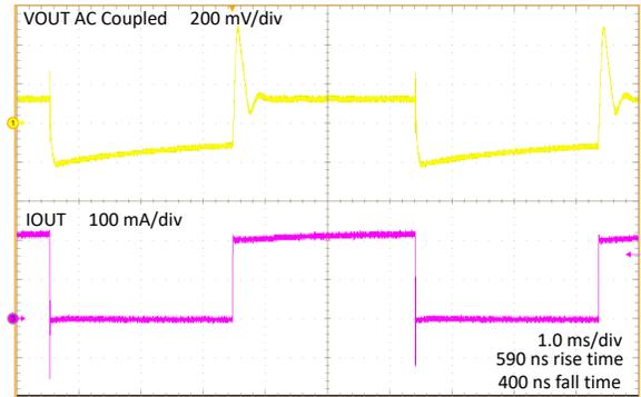
Figure 4-8. Load Transient Response, 0 mA to 410 mA With  $V_{IN} = 24\text{ V}$ ,  $V_{OUT} = -12\text{ V}$
