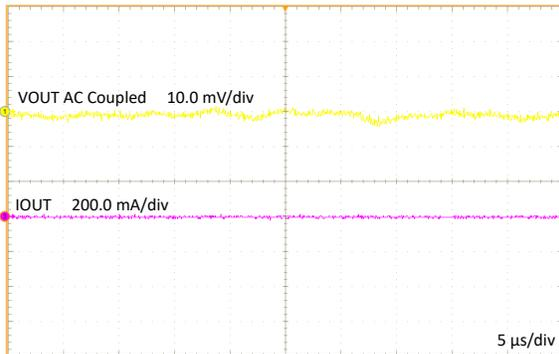
Figure 4-9. Output Voltage Ripple,  $V_{IN} = 24\text{ V}$ ,  $V_{OUT} = -12\text{ V}$ ,  $I_{OUT} = 0\text{ mA}$
