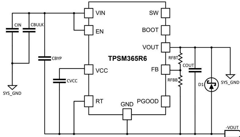
Figure 2-1. TPSM365R6 IBB with Schottky Diode and Bulk and Bypass Capacitors
