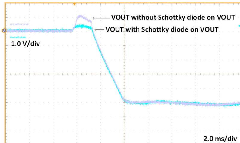
Figure 2-2. TPSM365R6 IBB Startup with Schottky Diode
