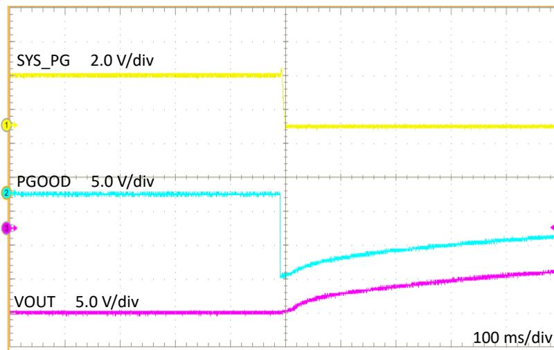
**Figure 5-6. PG Pin Level Shifter on Shutdown**
