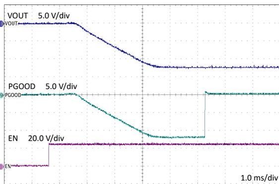
Figure 4-5. Start-up on  $V_{IN} = 24$  V,  $V_{OUT} = -12$  V, Expected Performance With no Level Shifters
