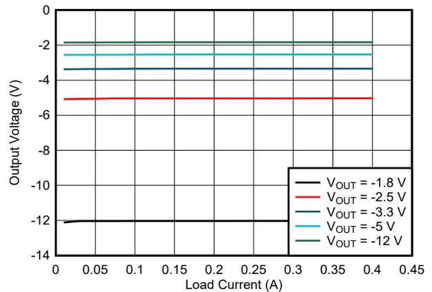
Figure 4-4. Load Regulation at  $V_{IN} = 24$  V
