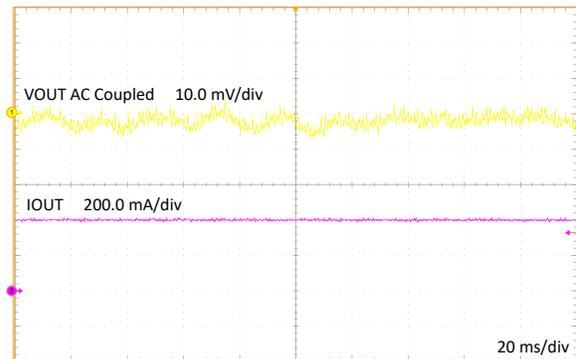
Figure 4-10. Output Voltage Ripple,  $V_{IN} = 24\text{ V}$ ,  $V_{OUT} = -12\text{ V}$ ,  $I_{OUT} = 410\text{ mA}$
