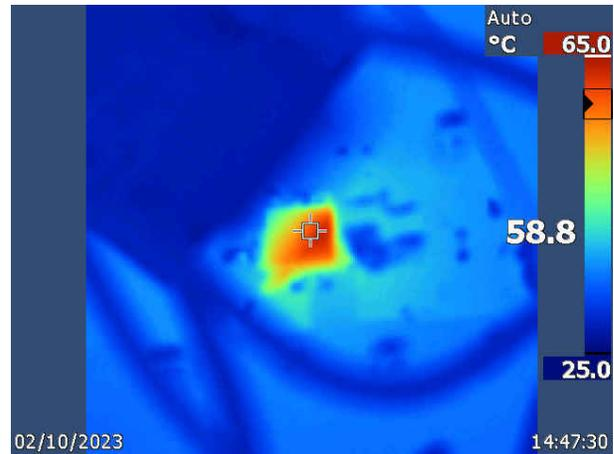
Figure 4-12. Temperature Response,  $V_{IN} = 24\text{ V}$ ,  $V_{OUT} = -12\text{ V}$ ,  $I_{OUT} = 410\text{ mA}$
