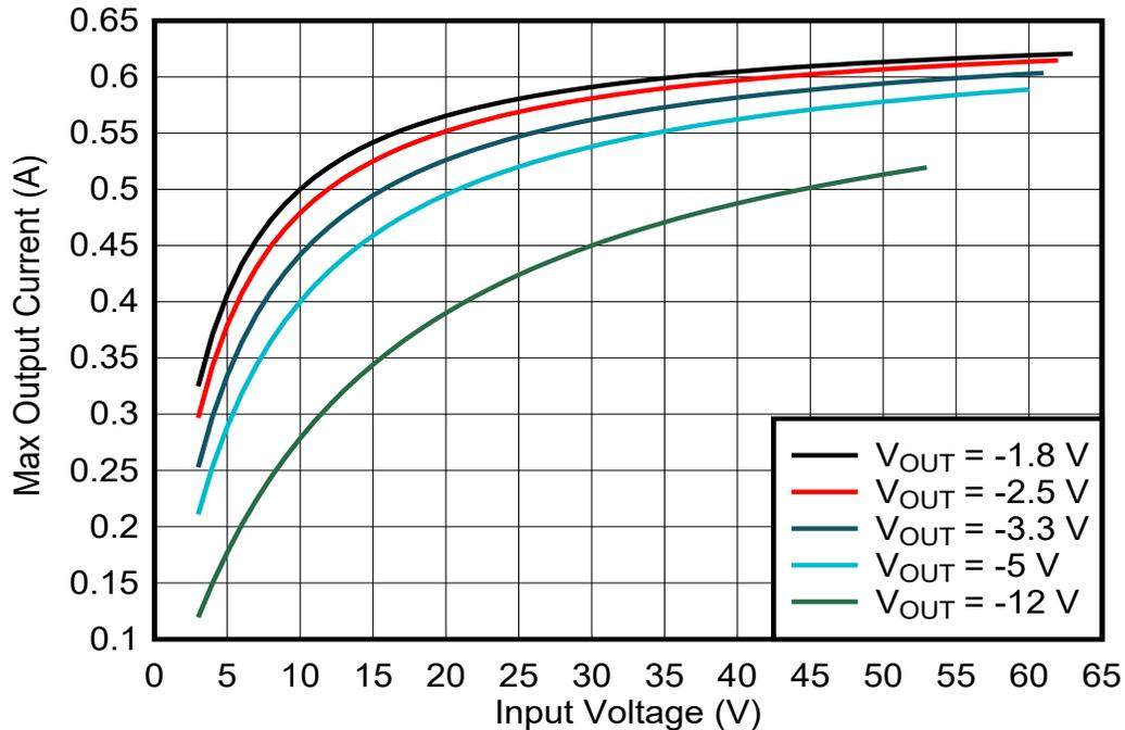
**Figure 1-2. Recommended Maximum Output Current for TPSM365R6**
