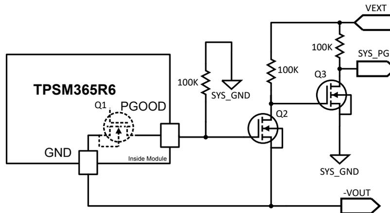
**Figure 5-4. PGOOD Pin Level Shifter**
