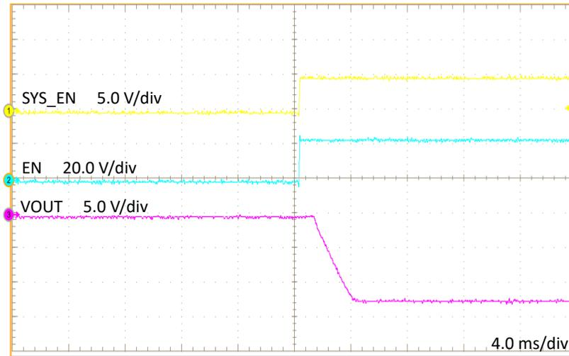
**Figure 5-2. EN Pin Level Shifter on Start-Up**
