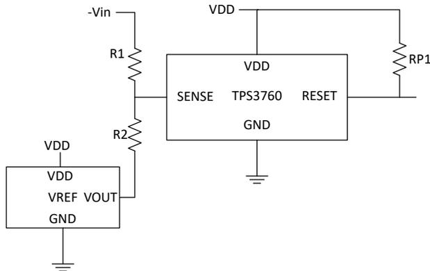
**Device shown:** [TPS3760A012DYR](#) adjustable threshold variant
