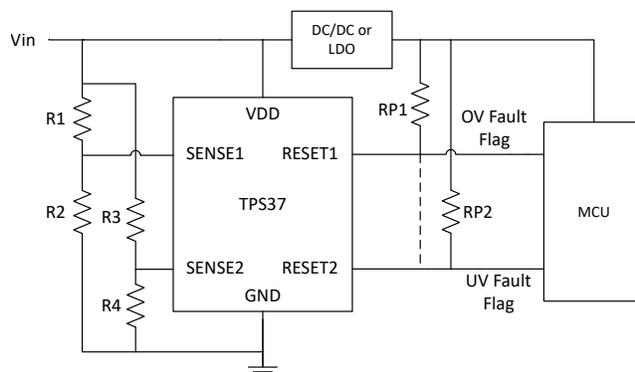
Device shown: [TPS37A010122DSKR](#) adjustable threshold variant
