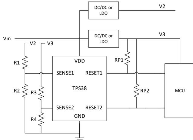
**Device shown:** [TPS38A010122DSKRQ1](#) adjustable threshold variant
