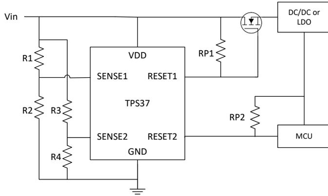
**Device shown:** [TPS37A010122DSKR](#) adjustable threshold variant
