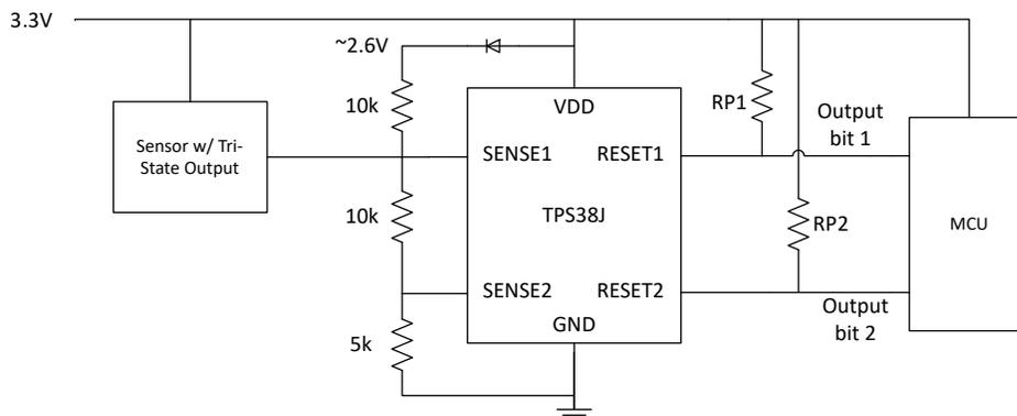
**Device shown:** [TPS38J010155DSKRQ1](#) adjustable threshold variant
