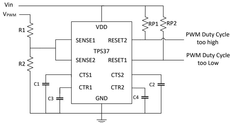
**Device shown:** [TPS37A010122DSKR](#) adjustable threshold variant
