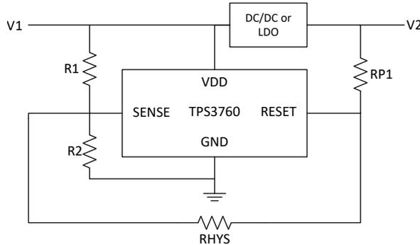
**Device shown:** [TPS3760A012DYR](#) adjustable threshold variant
