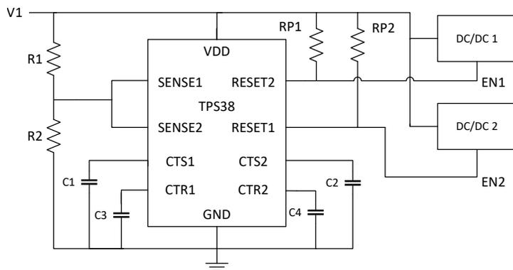
**Device shown:** [TPS38A010122DSKRQ1](#) adjustable threshold variant
