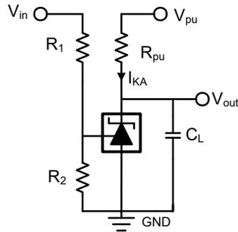
Figure 4-1. Comparator Mode Design Example
