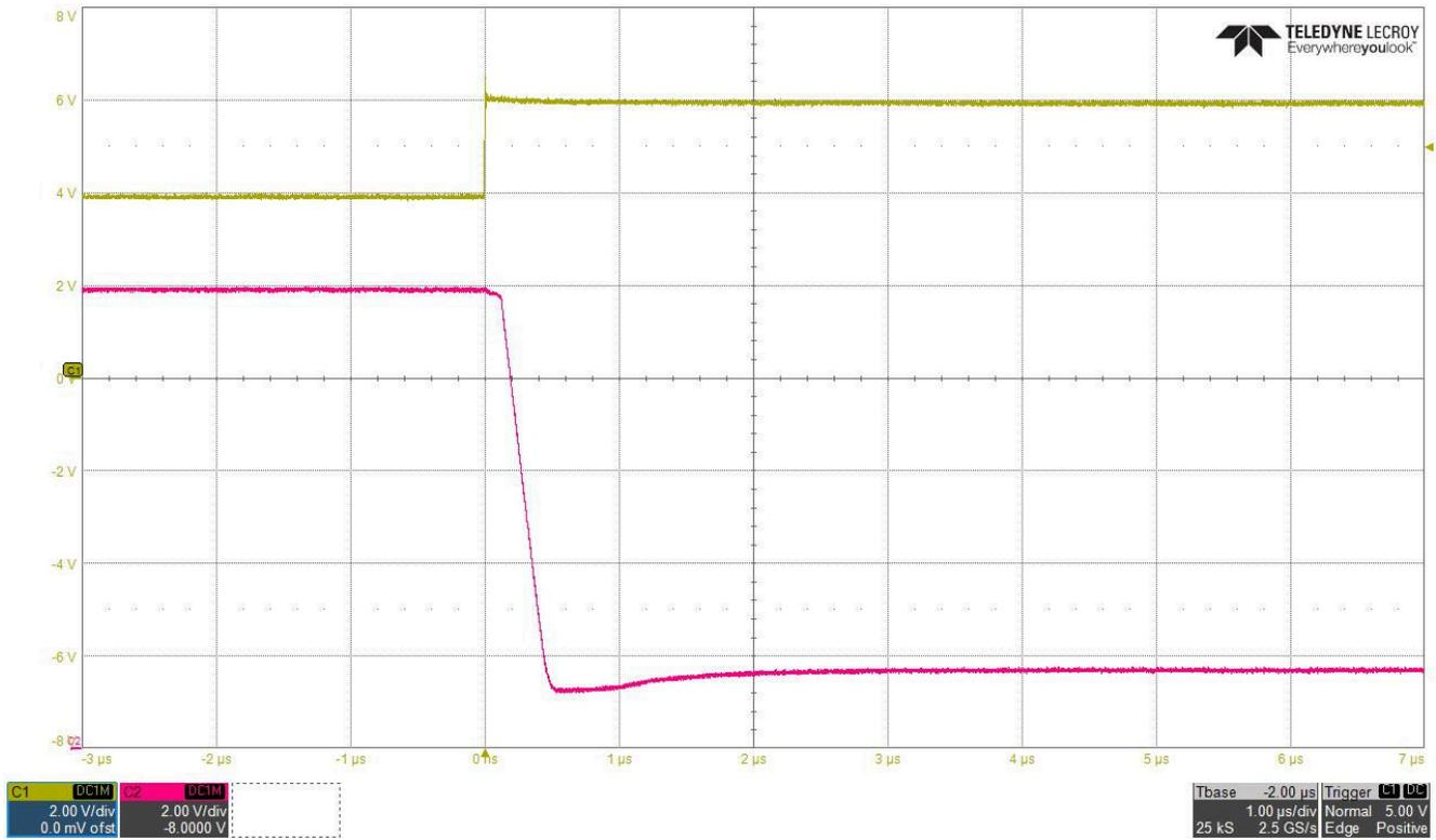
Figure 4-3. Propagation Delay (T<sub>PLH</sub>): TL431LI
