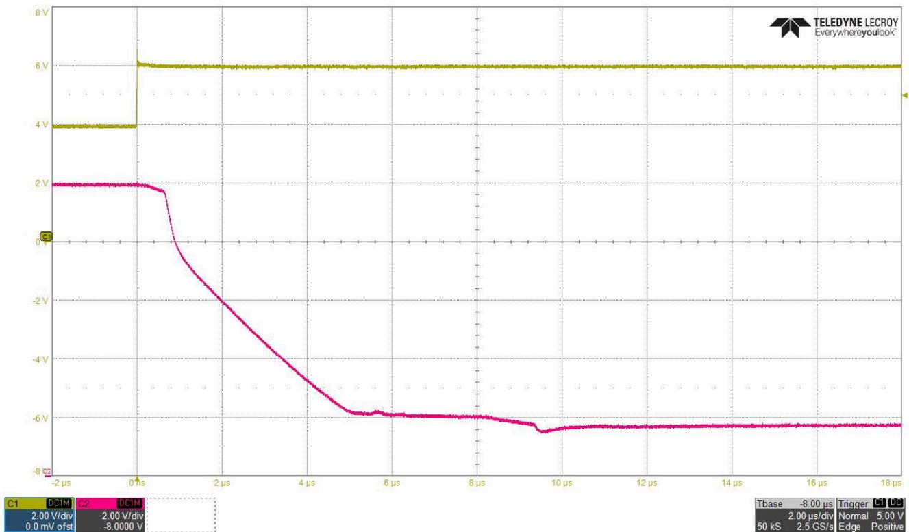
Figure 4-4. Propagation Delay (T<sub>PLH</sub>): ATL431
