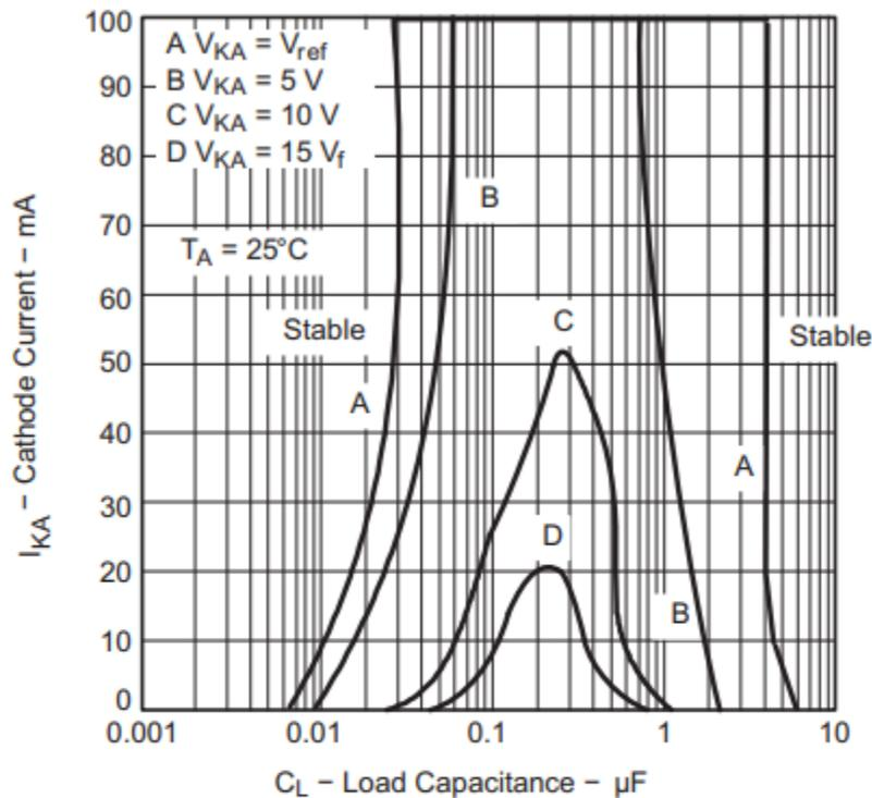
The areas under the curves represent conditions that may cause the device to oscillate. For curves B, C, and D, R2 and V+ are adjusted to establish the initial  $V_{KA}$  and  $I_{KA}$  conditions, with  $C_L = 0$ .  $V_{BATT}$  and  $C_L$  then are adjusted to determine the ranges of stability.
