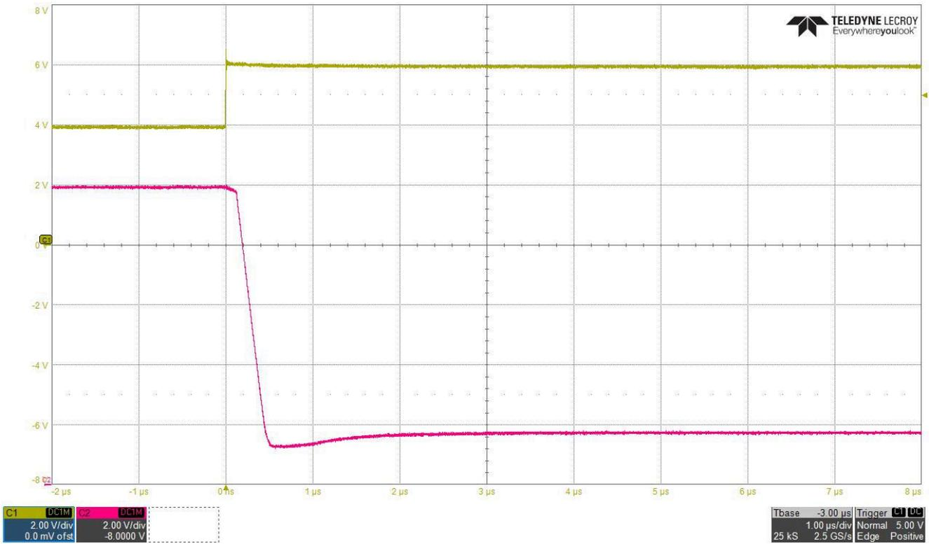
**Figure 4-5. Propagation Delay (T<sub>PLH</sub>): ATL431LI**
