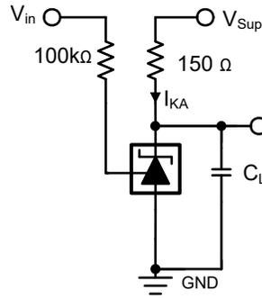
Figure 3-1. Test Circuit for Stability of TL431 in Comparator Mode
