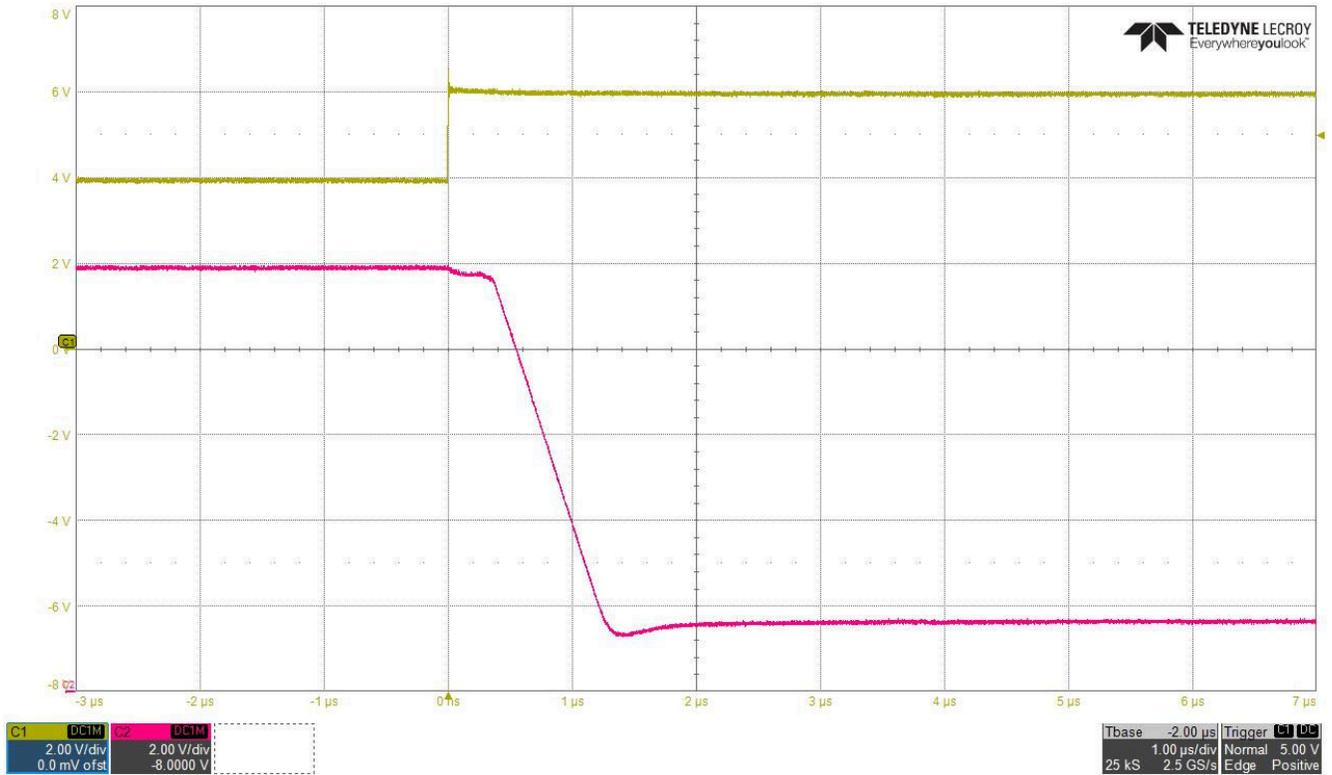
**Figure 4-2. Propagation Delay (T<sub>PLH</sub>): TL431**
