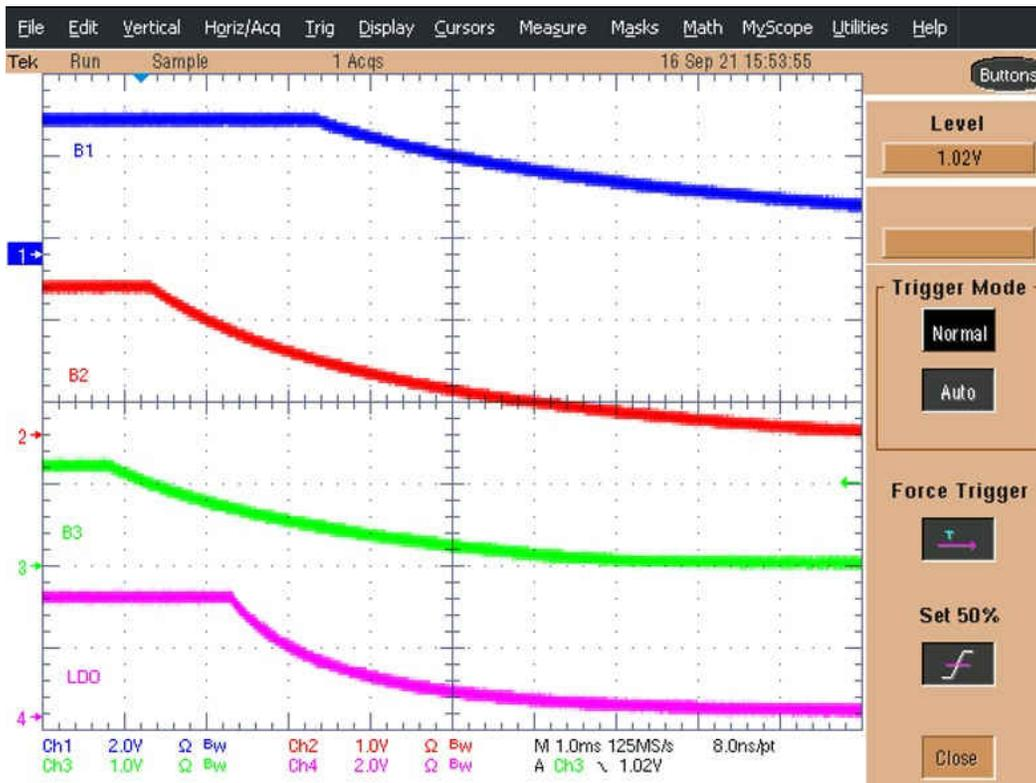
Figure 2-5. TPS650330-Q1 Programmable Power Down Sequence
