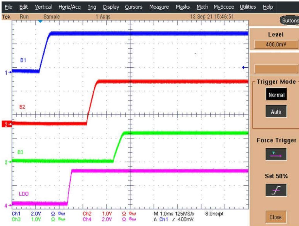
Figure 2-4. TPS650330-Q1 Programmable Power Up Sequence
