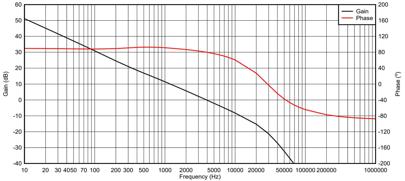
**Figure 2-5. Bode Plot of Outer Voltage Loop**
