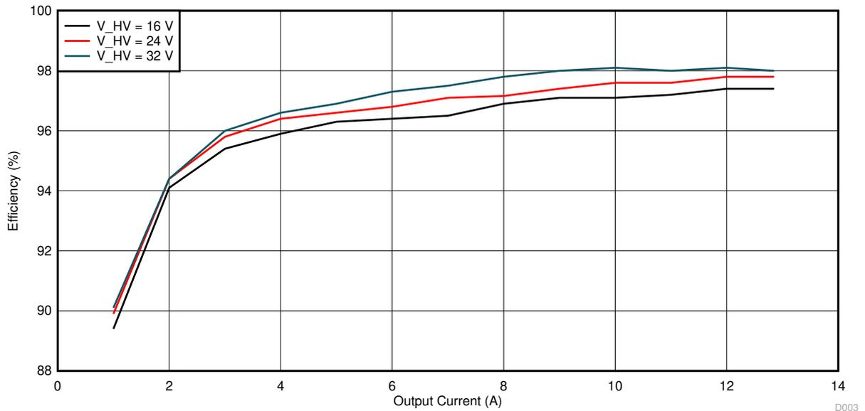
Figure 3-2. Buck Converter Efficiency
