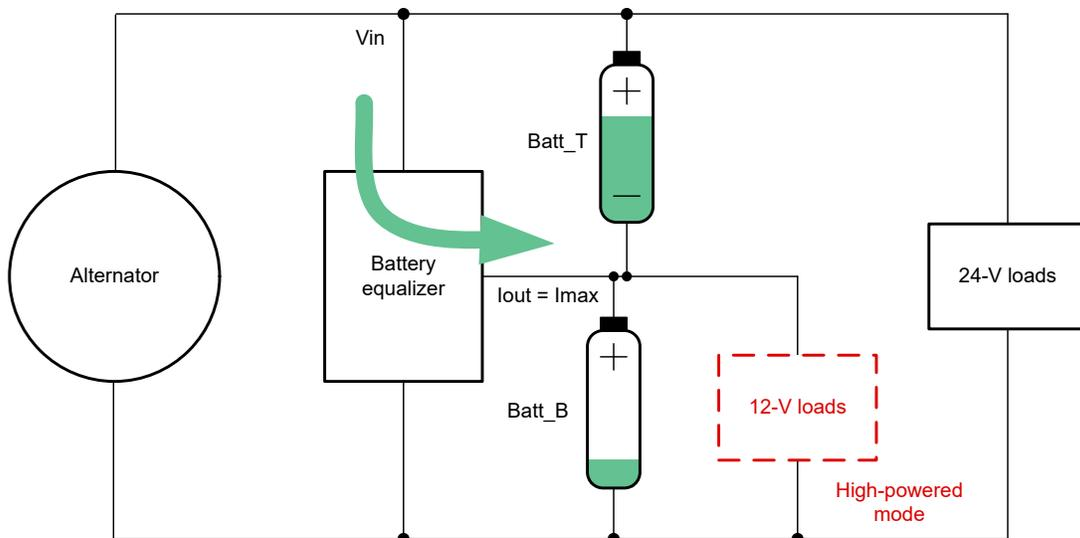
Figure 1-3. Constant Current Mode of Battery Equalizer
