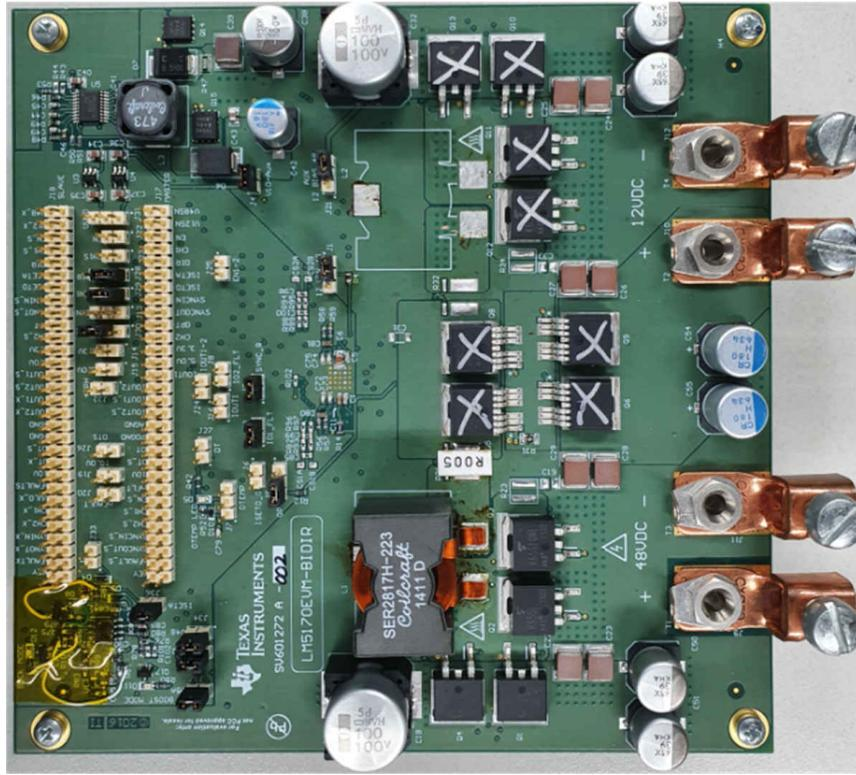
Figure 3-1. Test Board (Texas Instruments LM5170EVM-BIDR Modified)
