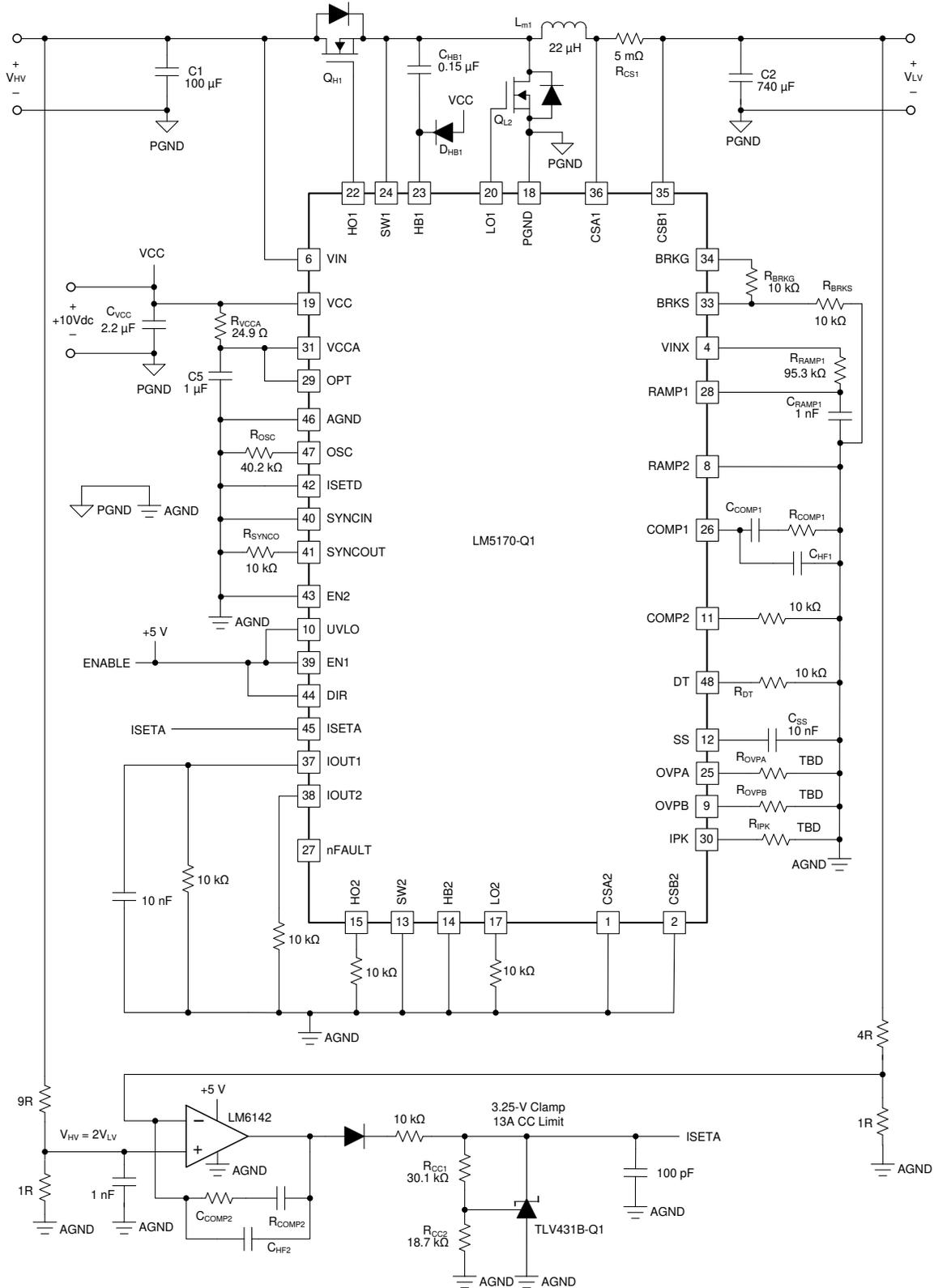
Figure 2-1. Schematic of Buck Converter for Battery Equalizer
