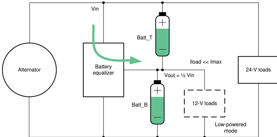
Figure 1-2. Constant Voltage Mode of Battery Equalizer
