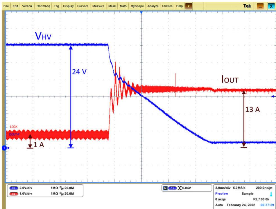
Figure 3-4. Input Voltage and Output Current Waveform in Constant Current Mode
