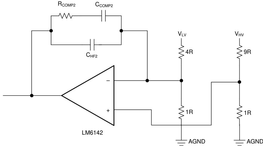
**Figure 2-4. Outer Voltage Loop Control in LM5170-Q1**
