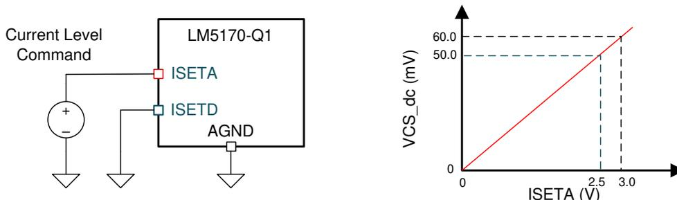
**Figure 2-6. ISETA vs VCS<sub>dc</sub> Graph of LM5170-Q1**
