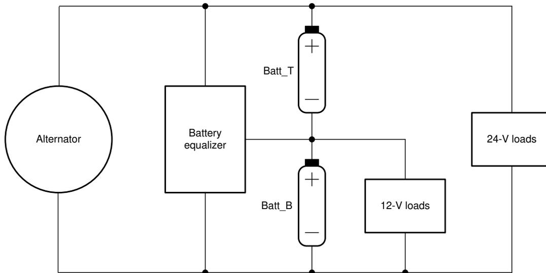
**Figure 1-1. Power System of Commercial Vehicles**
