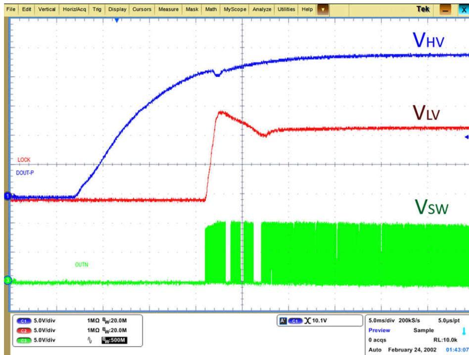
Figure 3-5. Start-up Sequence of Buck Converter
