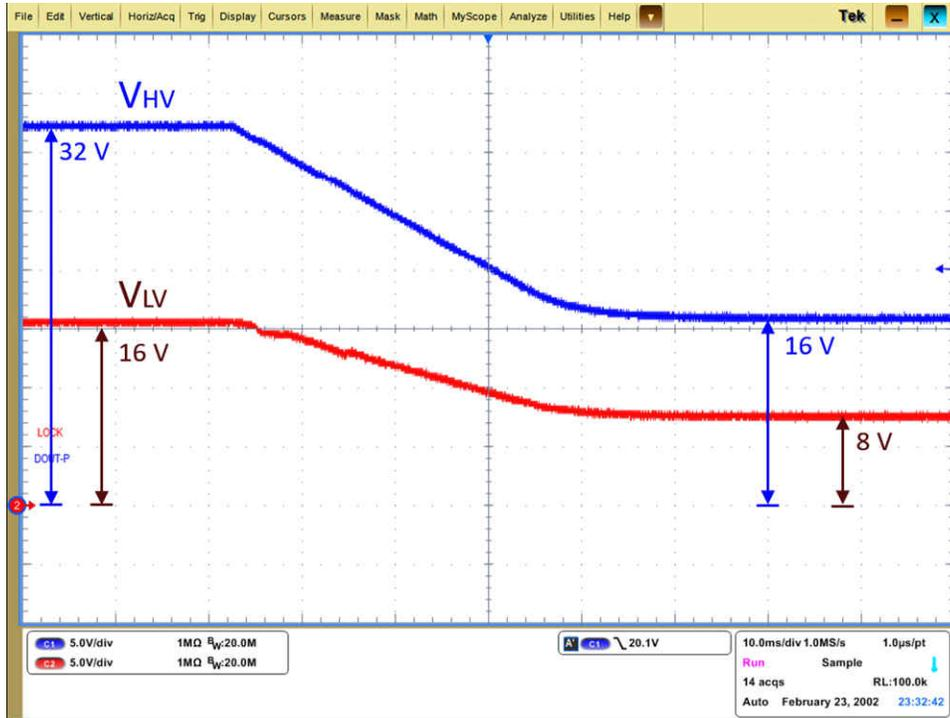
Figure 3-3. Input Voltage and Output Voltage Waveform in Constant Voltage Mode
