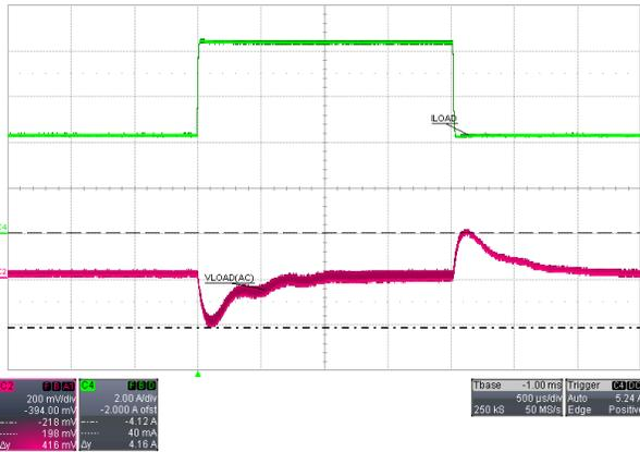
Figure 3-3. Load Transient  $V_{LOAD} = 24V, V_{SUPPLY} = 8 V$
