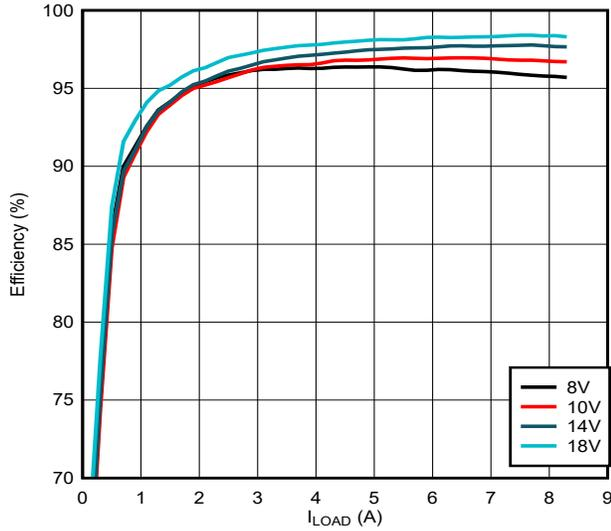
Figure 3-1. Efficiency  $V_{LOAD} = 24 V$
