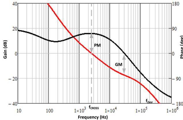
**Figure 4-3. Open Loop Transfer function**
