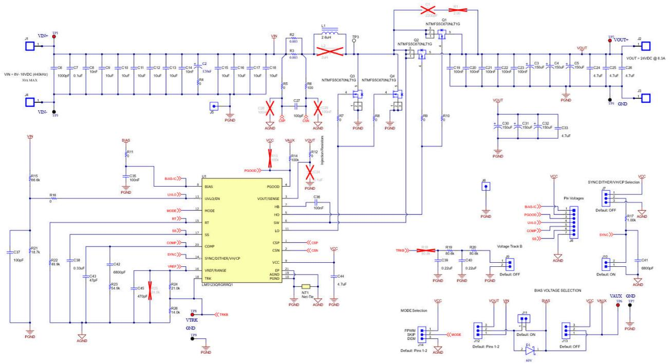
Figure 3-7. LM5123EVM-BST Schematic
