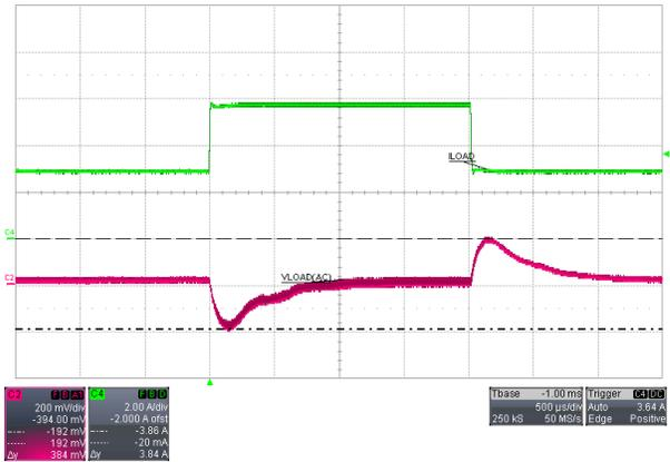
Figure 3-4. Load Transient  $V_{LOAD} = 35 V, V_{SUPPLY} = 8 V$
