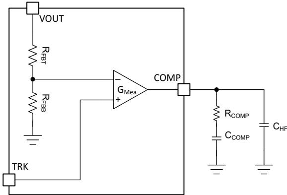
Figure 2-5. Control loop compensation network
