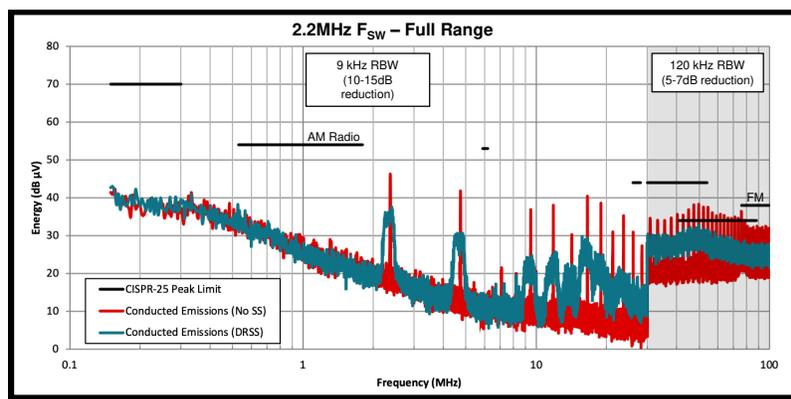
**Figure 3-3. Conduction EMI Reduction by DRSS (LM5156, Switching at 2.2 MHz)**
