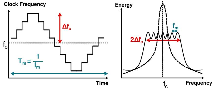
**Figure 2-2. Triangular Modulation in the Time (Left) and Frequency Domain (Right)**
