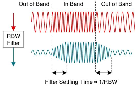
**Figure 2-3. Settling Time Effects of the RBW Filter**
