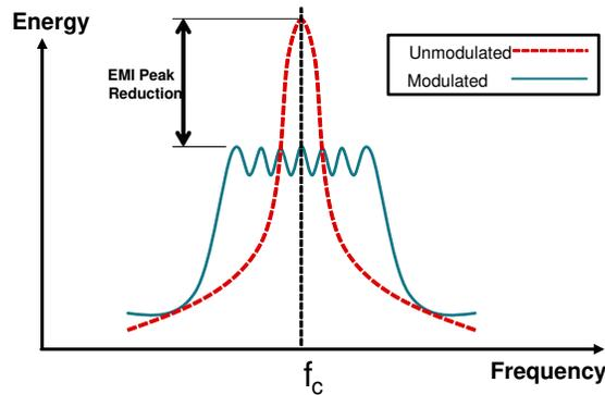
**Figure 2-1. EMI Reduction by Spread Spectrum, Frequency Modulation**
