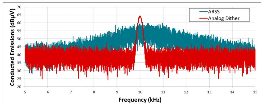
**Figure 3-1. ARSS Improves Audible Noise by Spreading the 10-kHz Tone**
