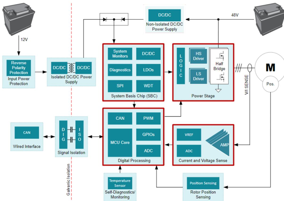
Figure 1. Starter Generation Unit Block Diagram
