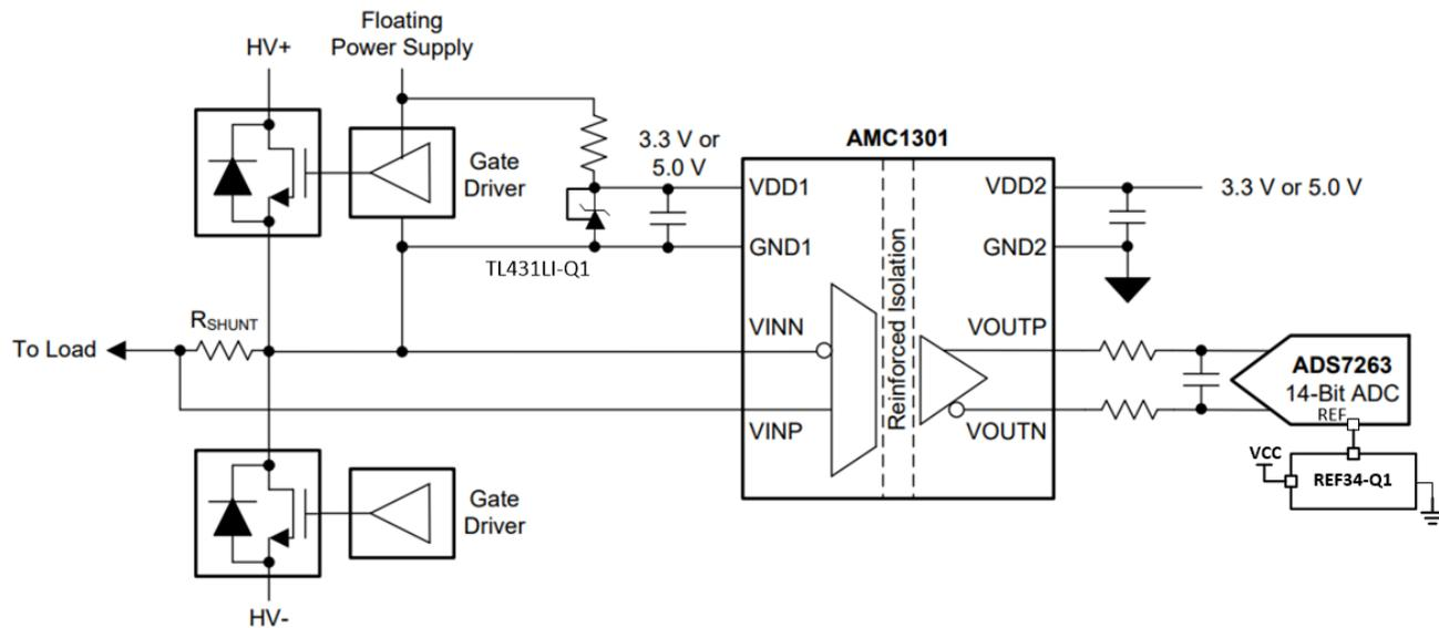
**Figure 12. High Voltage Current Monitoring Application Design**
