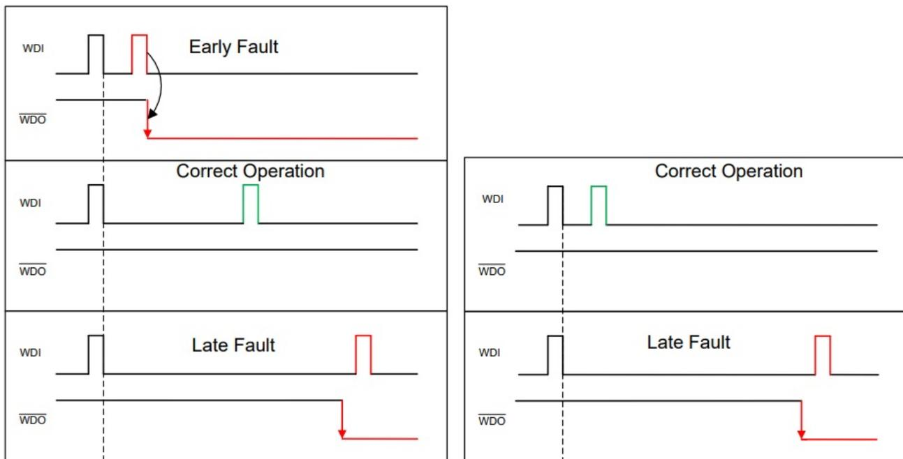
Figure 5. Window Watchdog (Left) Vs. Standard Watchdog (Right)
