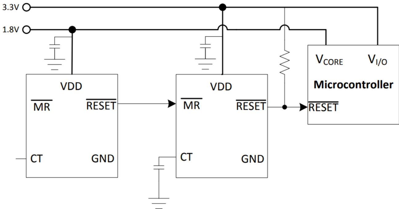
Figure 4. Microcontroller Supply Monitoring With Voltage Supervisor(s)
