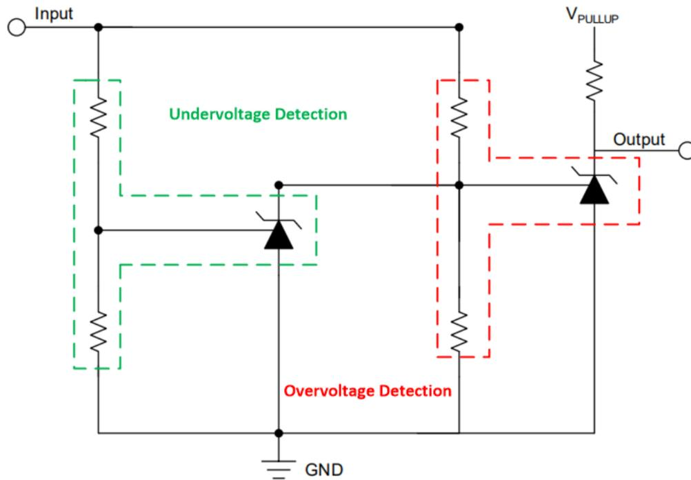
Figure 7. Circuit Topology for TL431 as a Window Comparator
