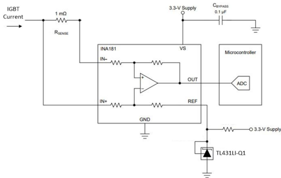
Figure 15. Current Sensing With INA181-Q1 and TL431LI-Q1
