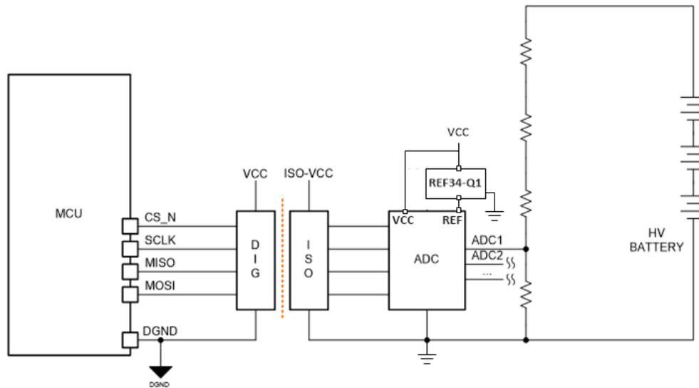
Figure 13. High-Side Voltage Sense Design Approach
