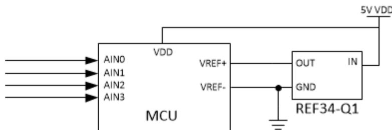
Figure 11. External ADC Referencing With REF34-Q1
