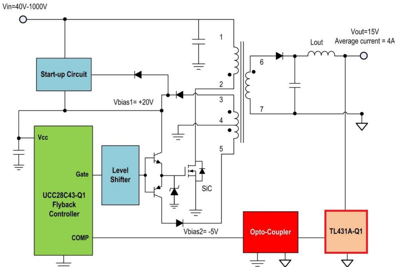
**Figure 19. Isolation Compensation with TL431A-Q1 in TIDA-01505**
