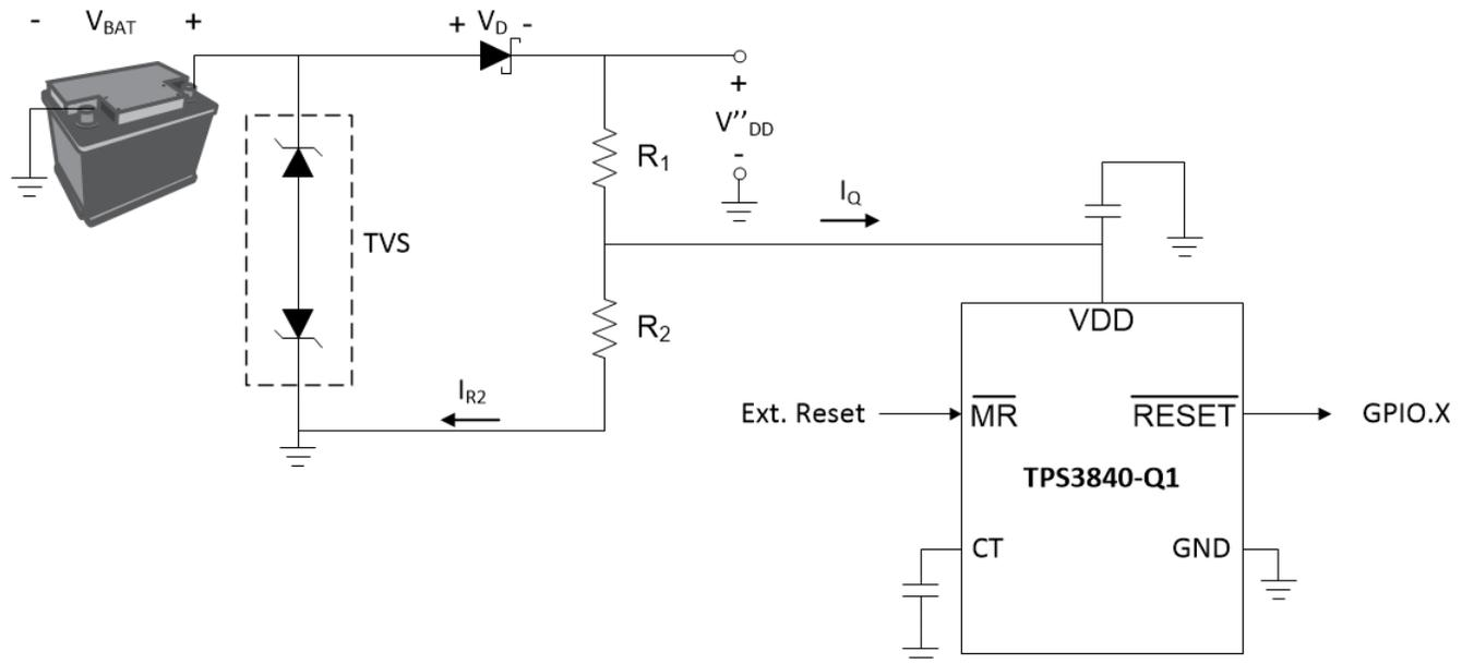
Figure 9. Illustrating TPS3840-Q1 Implementation For Wide- $V_{IN}$  Designs
