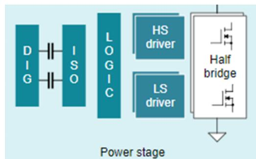
Figure 16. Power Stage Entities And Functional Blocks
