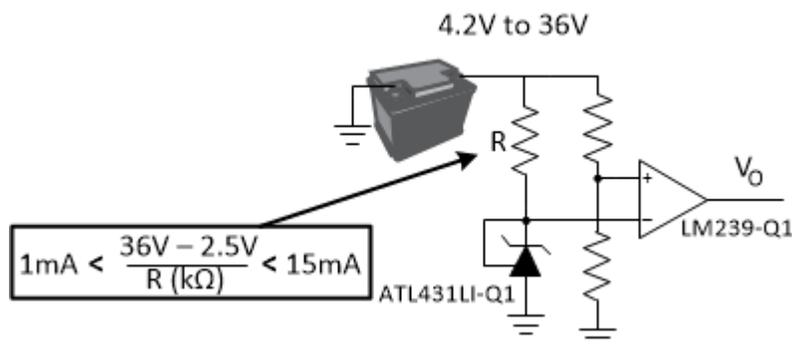
Figure 8. Detecting Off-Battery Fault With Comparator and TL431LI-Q1
