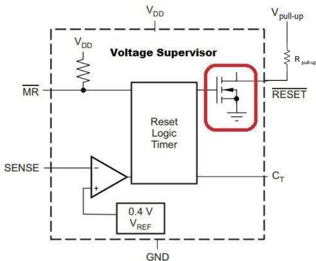
Figure 1. Voltage Supervisor Latch Circuit
