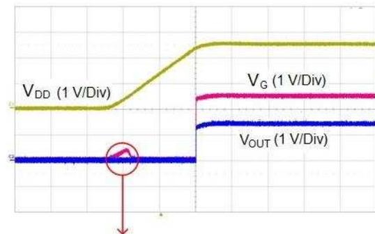
$V_G$  rises up to  $\sim 400$  mV because  $V_{DD}$  is too low to pull  $V_G$  to 0V
