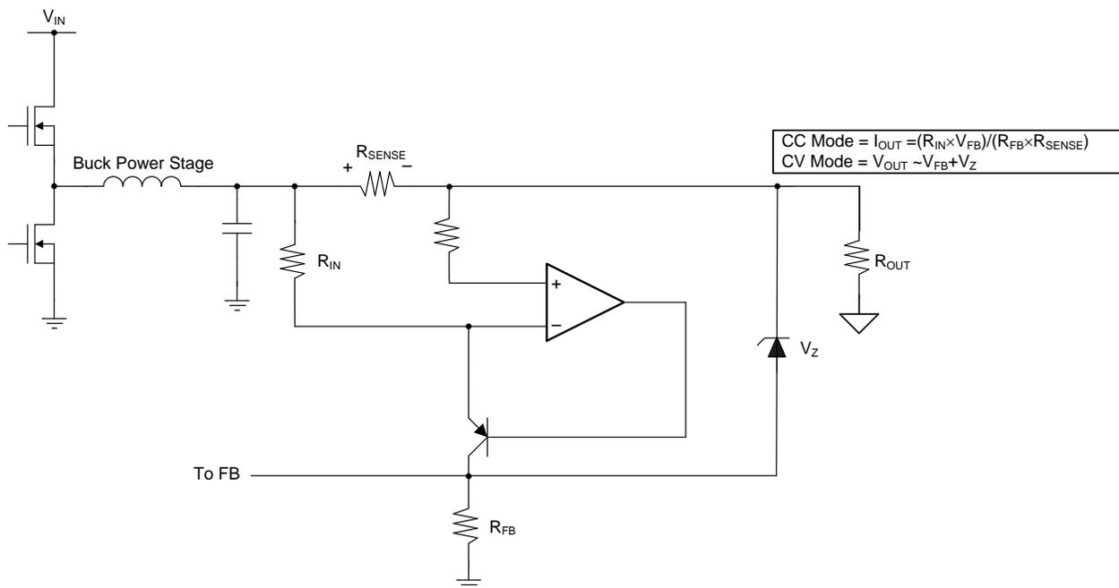
Figure 1. CC/CV Implementation With a Buck Topology
