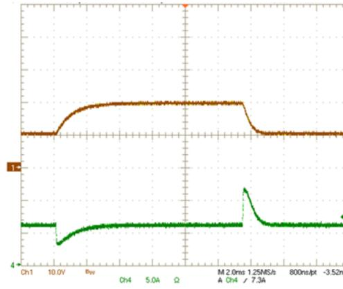
**Figure 7. Load-Transient Performance**
