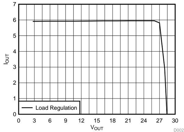
Figure 5. Load Regulation at 30 V<sub>IN</sub> With Increasing R<sub>LOAD</sub> (V<sub>OUT</sub> / I<sub>OUT</sub>)
