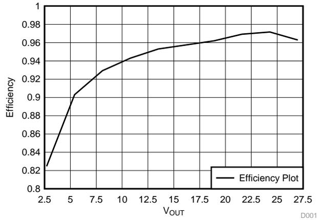
Figure 4. Efficiency at 30 V<sub>IN</sub>
