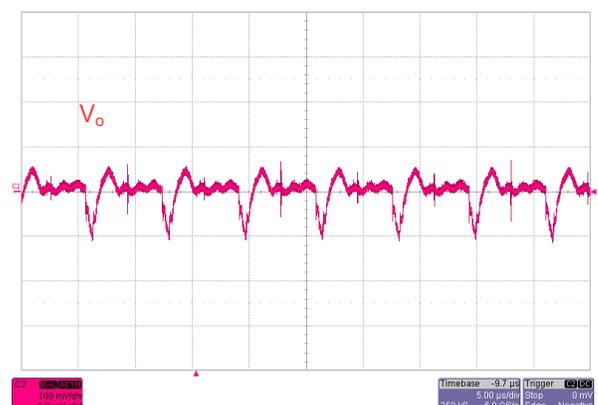
Figure 49. Output Voltage Ripple in 12-V Buck-Boost Region—40-A Load
