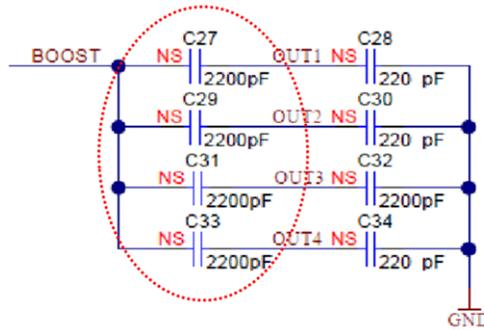
Figure 34. Circuit With Capacitors Between Boost Out and LED Drive
