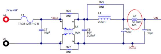
Figure 20. Circuit With Boost Input Filter: Ferrite Bead
