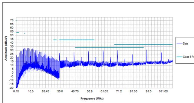
**Figure 63. Conducted Emissions for 400-kHz Return**
