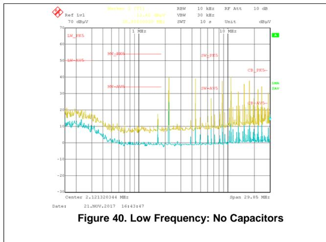
Figure 40. Low Frequency: No Capacitors
