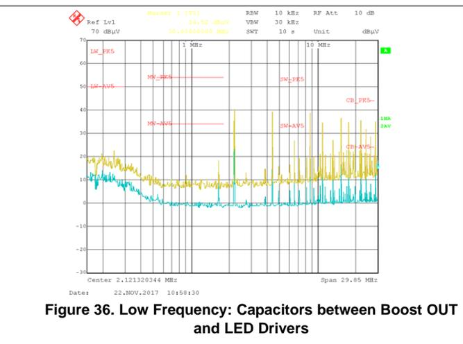
Figure 36. Low Frequency: Capacitors between Boost OUT and LED Drivers
