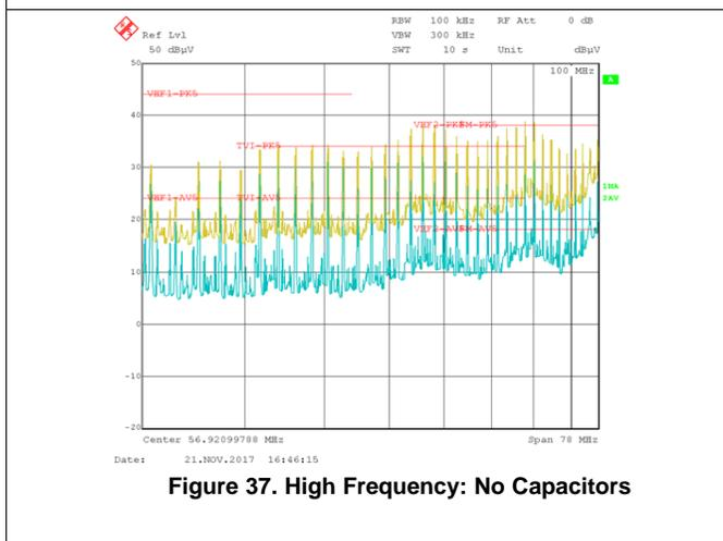
Figure 37. High Frequency: No Capacitors
