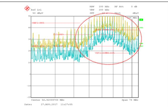
Figure 19. High Frequency: Bypassed CM Choke
