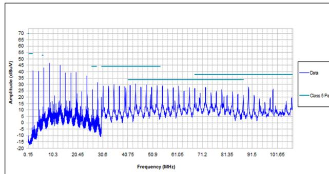
**Figure 62. Conducted Emissions for 400-kHz Line**
