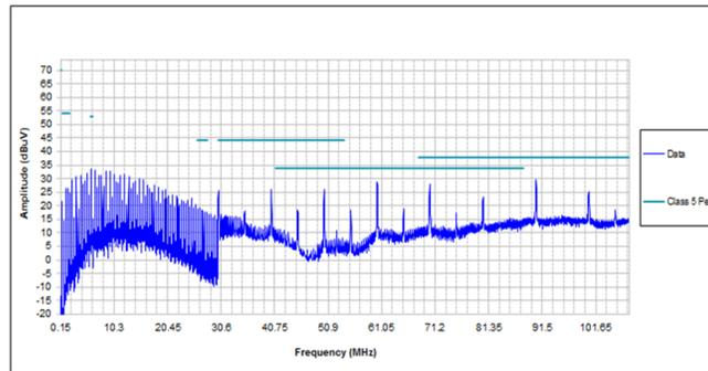
**Figure 61. Conducted Emissions for 2.2-MHz Return**
