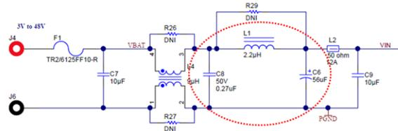
Figure 10. Circuit With Boost Input Filter: Pi Filter
