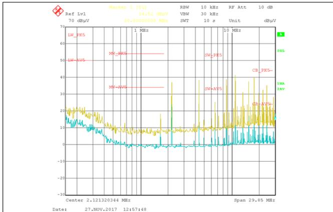
Figure 21. Low Frequency: Used Ferrite Bead
