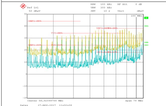
Figure 18. High Frequency: Used CM Choke
