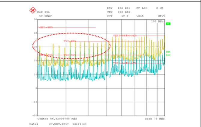
Figure 14. High Frequency: Bypassed Pi Filter
