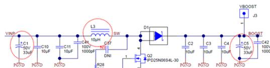
**Figure 5. Boost Section of LP8860-Q1 EMI Test Board**
