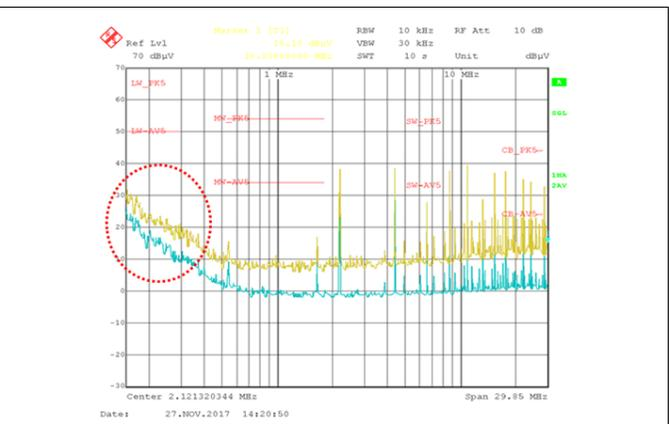
Figure 12. Low Frequency: Bypassed Pi Filter
