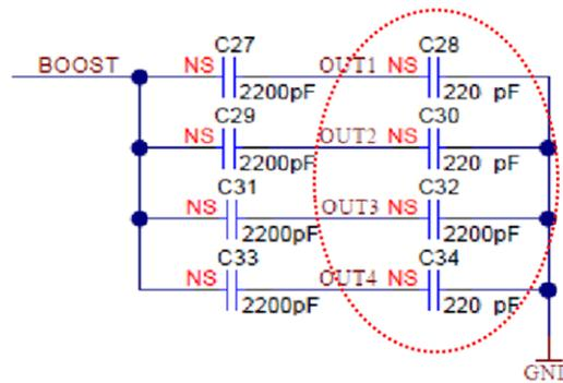
Figure 39. Circuit With Capacitors Between LED Drivers and GND
