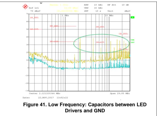
Figure 41. Low Frequency: Capacitors between LED Drivers and GND
