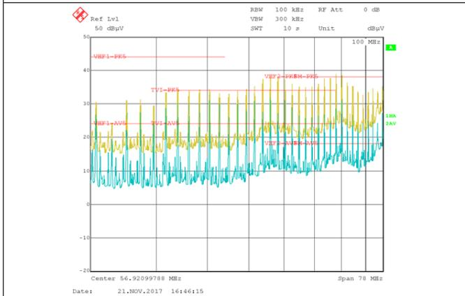
**Figure 50. High Frequency: 120 mA**
