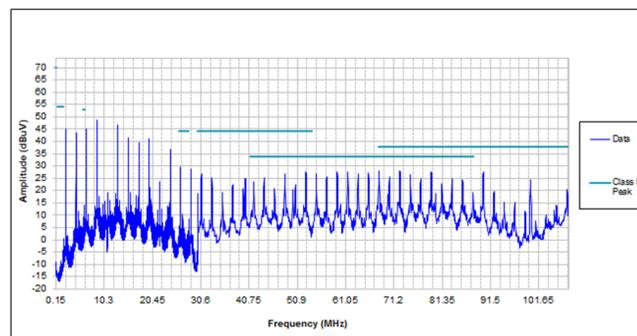
Figure 60. Conducted Emissions for 2.2-MHz Line
