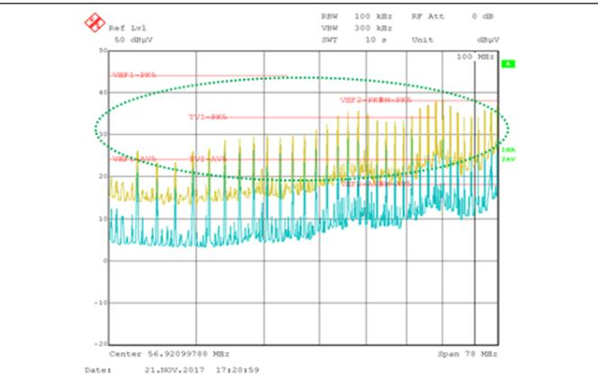
**Figure 51. High Frequency: 80 mA**
