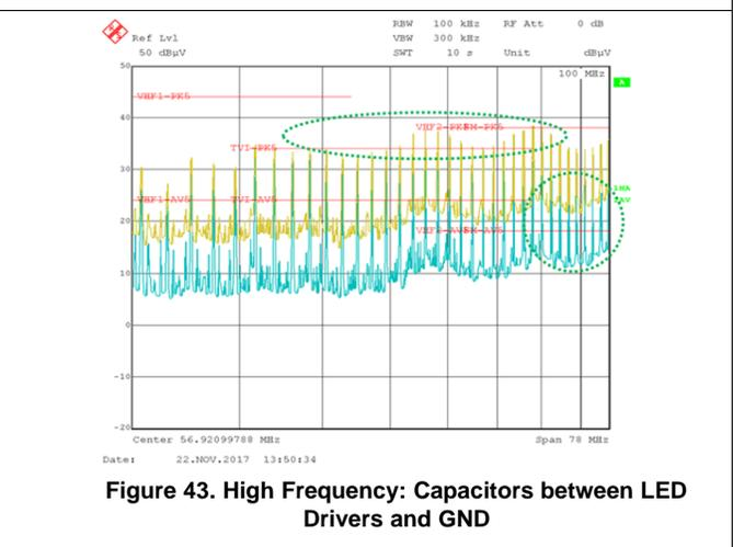
Figure 43. High Frequency: Capacitors between LED Drivers and GND
