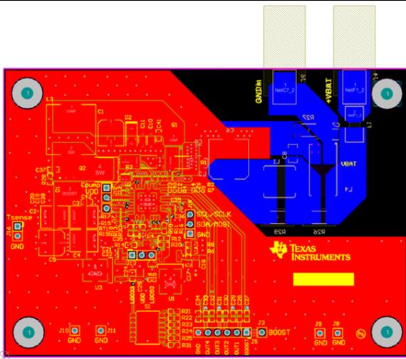
Figure 1. Top Layer of PCB Layout of LP8860-Q1 EMI Test Board
