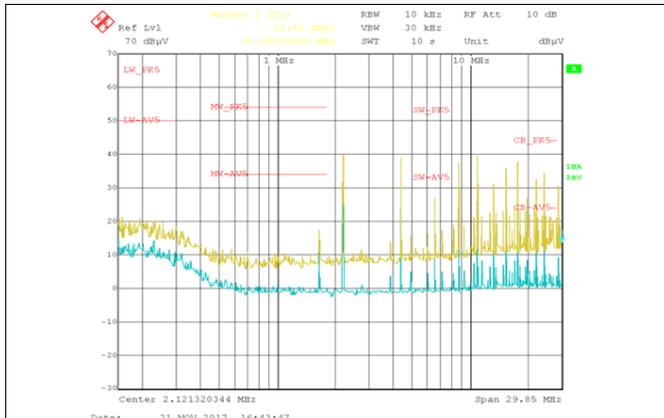
Figure 52. Low Frequency: 100% Brightness
