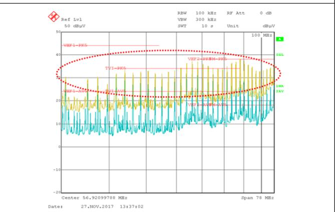
Figure 24. High Frequency: Bypassed Ferrite Bead
