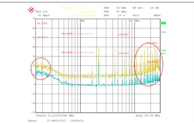
Figure 17. Low Frequency: Bypassed CM Choke
