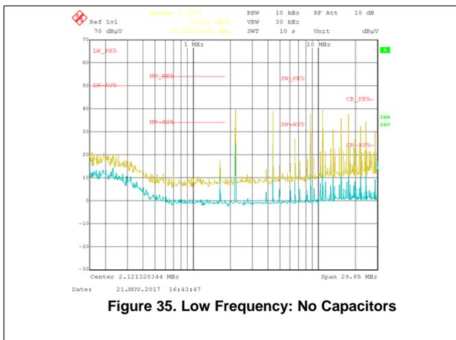
Figure 35. Low Frequency: No Capacitors
