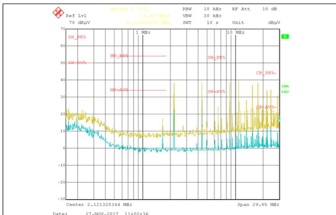
Figure 16. Low Frequency: Used CM Choke
