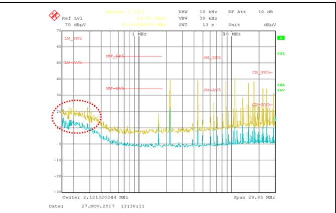
Figure 22. Low Frequency: Bypassed Ferrite Bead
