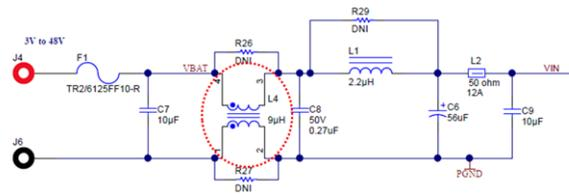
Figure 15. Circuit With Boost Input Filter: CM Choke
