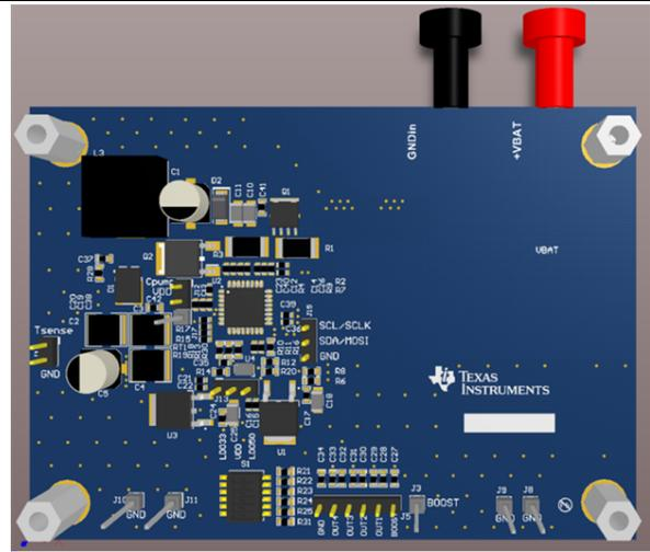
Figure 2. Top View of LP8860-Q1 EMI Test Board
