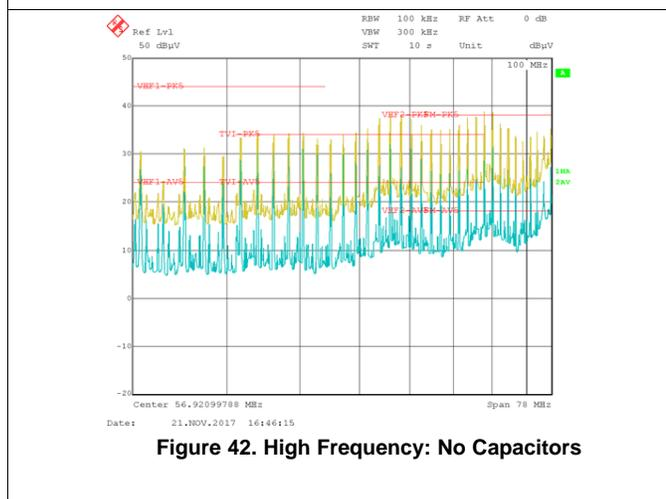
Figure 42. High Frequency: No Capacitors
