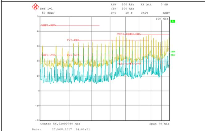
Figure 13. High Frequency: Pi Filter Used
