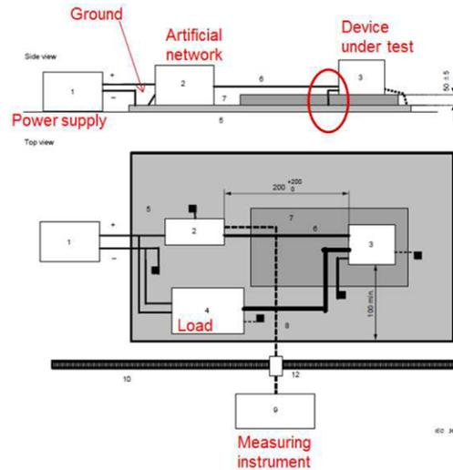
Figure 4. Schematic of LP8860-Q1 EMI Test Board
