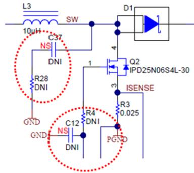
Figure 25. Circuit Using Snubbers
