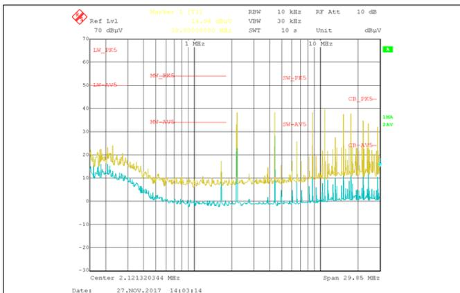
Figure 11. Low Frequency: Pi Filter Used
