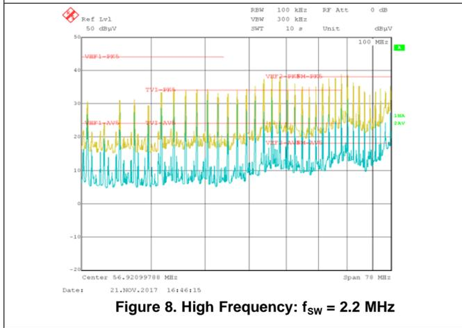
Figure 8. High Frequency:  $f_{SW} = 2.2 \text{ MHz}$
