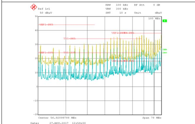
Figure 23. High Frequency: Used Ferrite Bead
