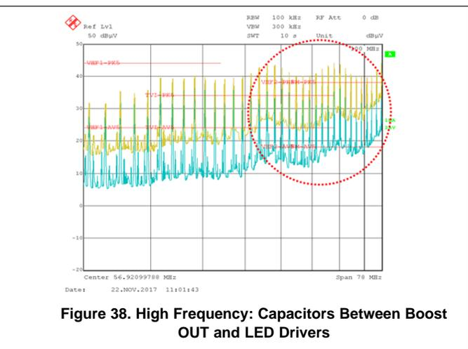
Figure 38. High Frequency: Capacitors Between Boost OUT and LED Drivers
