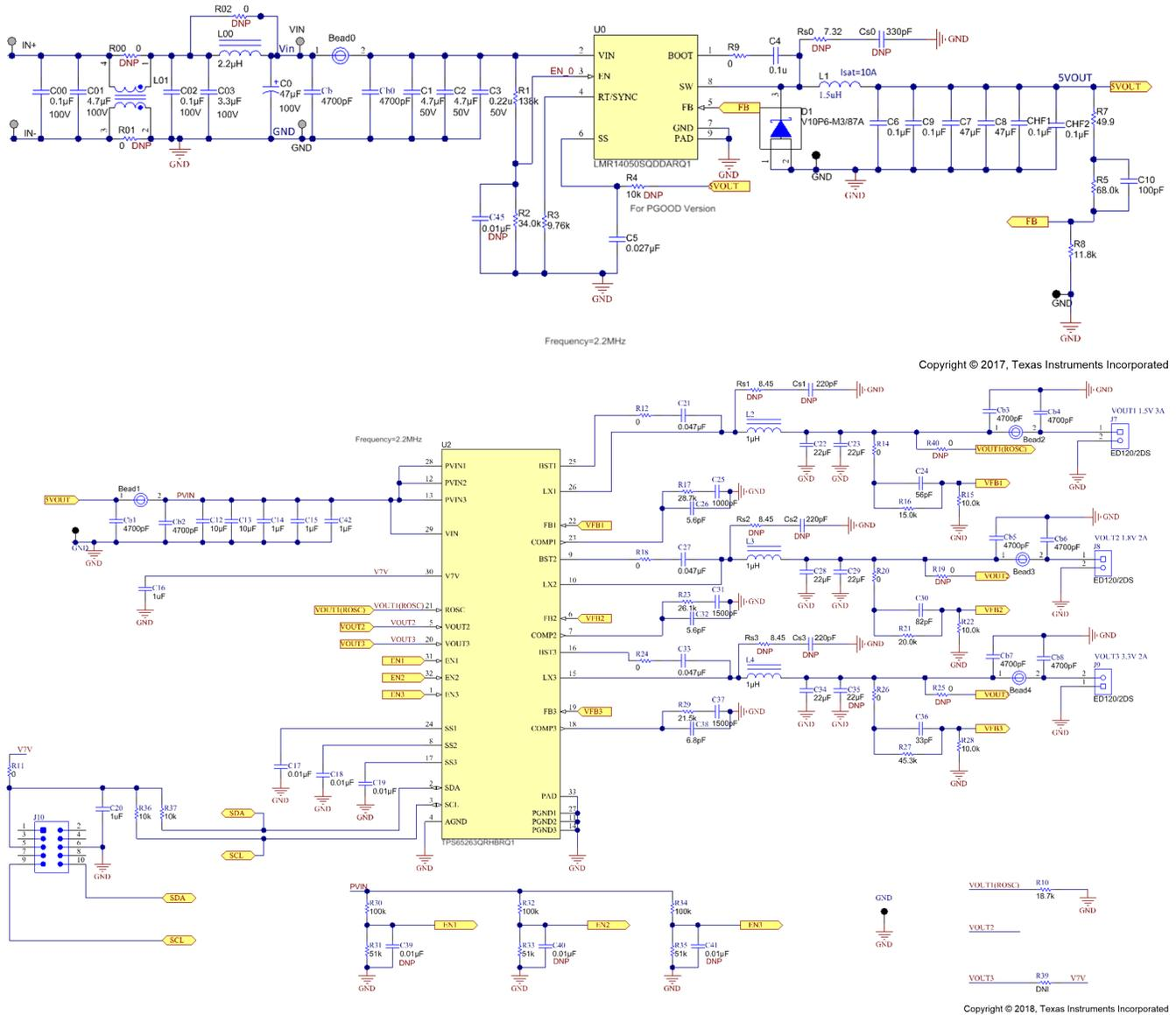
Figure 6. Solution for Processor of Automotive Digital Cockpit
