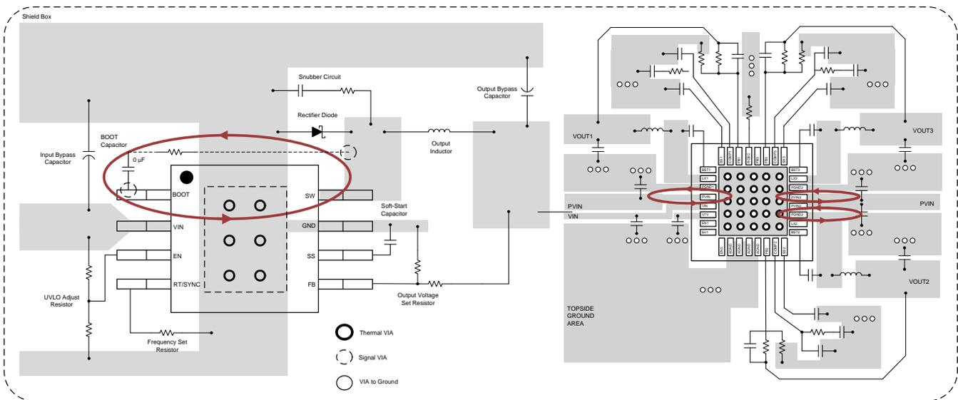
Figure 3. Pin Configuration Compact With the Layout
