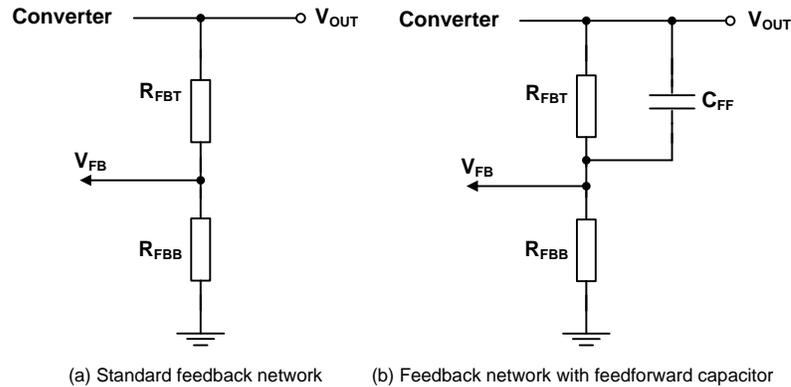
Figure 1. Feedback Network With and Without Feedforward Capacitor
