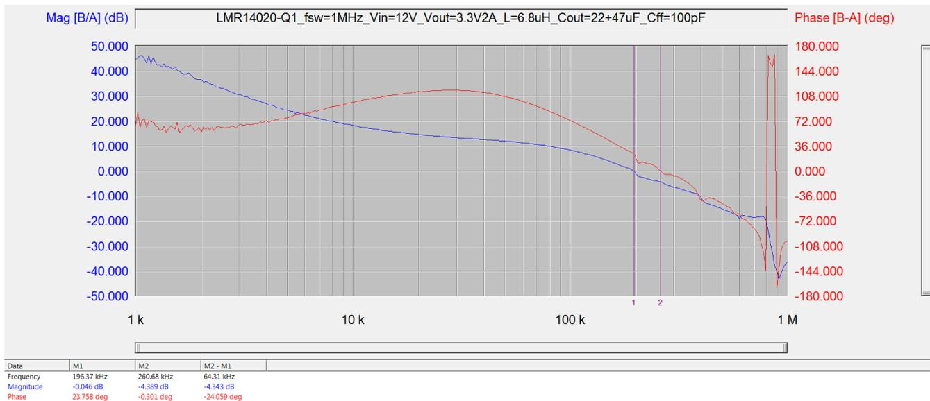
Figure 6. Loop Response With 100-pF Feedforward Capacitor
