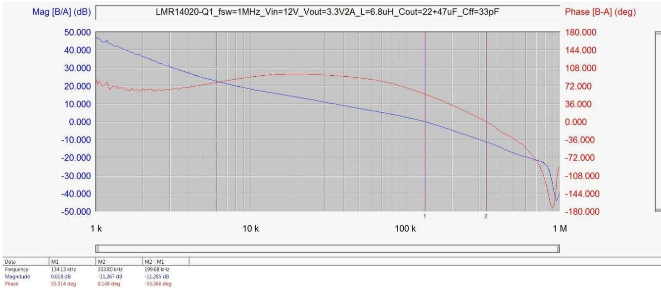
**Figure 9. Loop Response With 33-pF Feedforward Capacitor**
