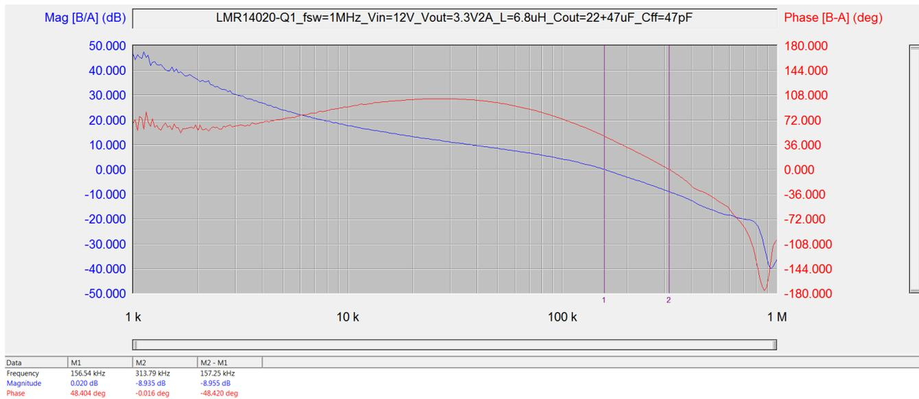
Figure 7. Loop Response With 47-pF Feedforward Capacitor
