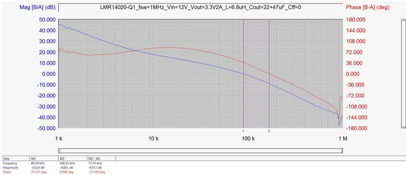
**Figure 3. Original Loop Response Without Feedforward Capacitor**
