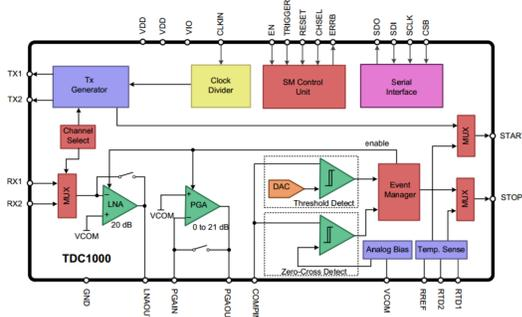
**Figure 2. TDC1000-Q1 Block Diagram**
