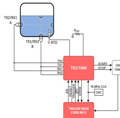
**Figure 3. Level and Concentration Sensing**
