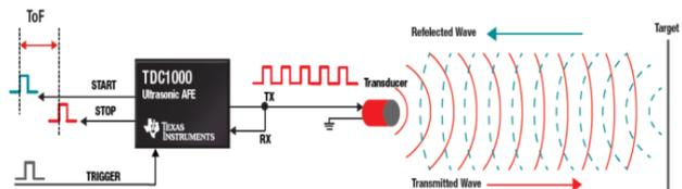
Figure 1. TDC1000 Application Diagram
