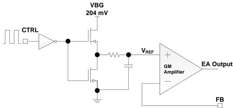
Figure 2. Internal Low-Pass Filter to Error Amplifier
