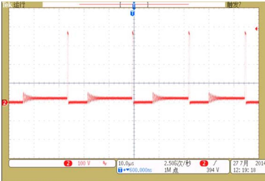
Figure 6. MOSFET Voltage Stress
