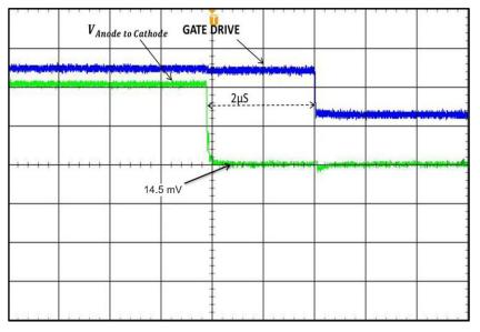
Figure 3. LM74610-Q1 Pull-Down Operation when Negative Polarity is Detected
