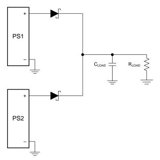
Figure 1. Schottky Diodes Used for OR-ing
