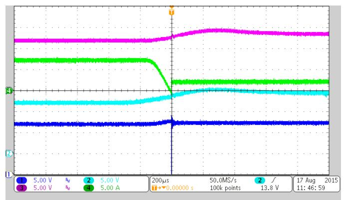
Figure 8. LM74610-Q1 OR-ing Device when PS2 Increases
