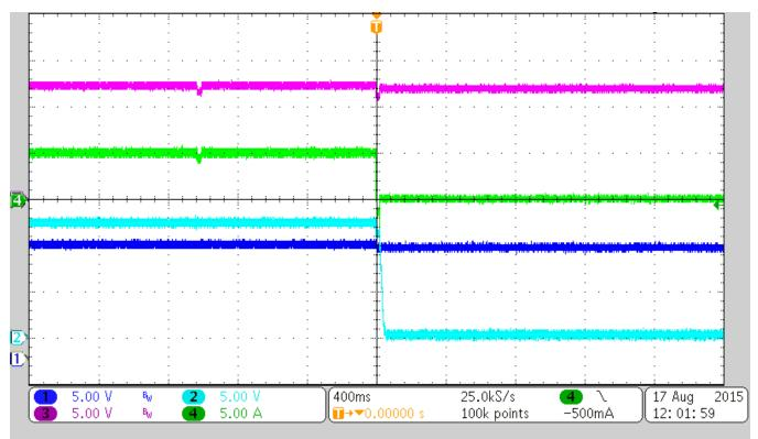
Figure 6. LM74610-Q1 OR-ing Device when P2 Fails
