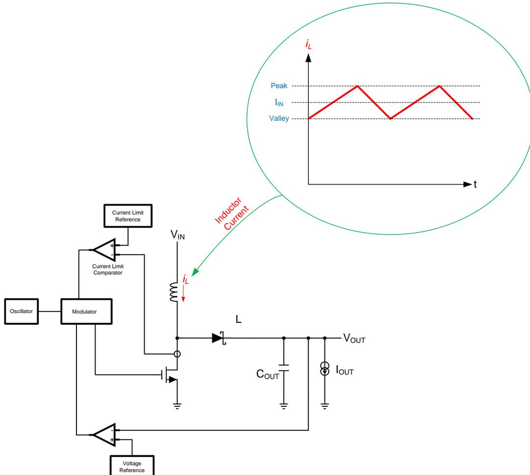
Figure 10. Simple Boost Converter
