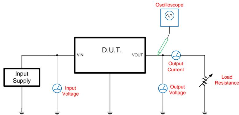
Figure 5. Current Limit Test Setup
