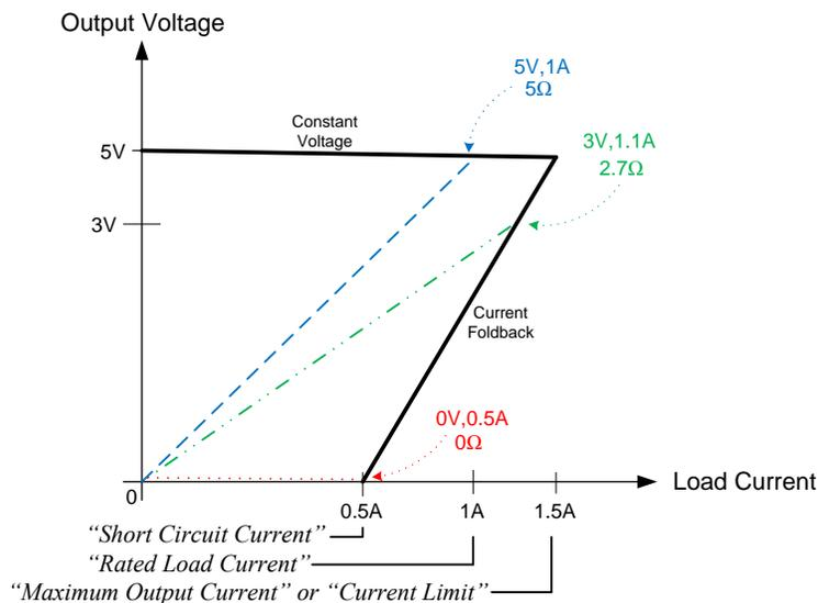
Figure 2. Fold-back Current Limit
