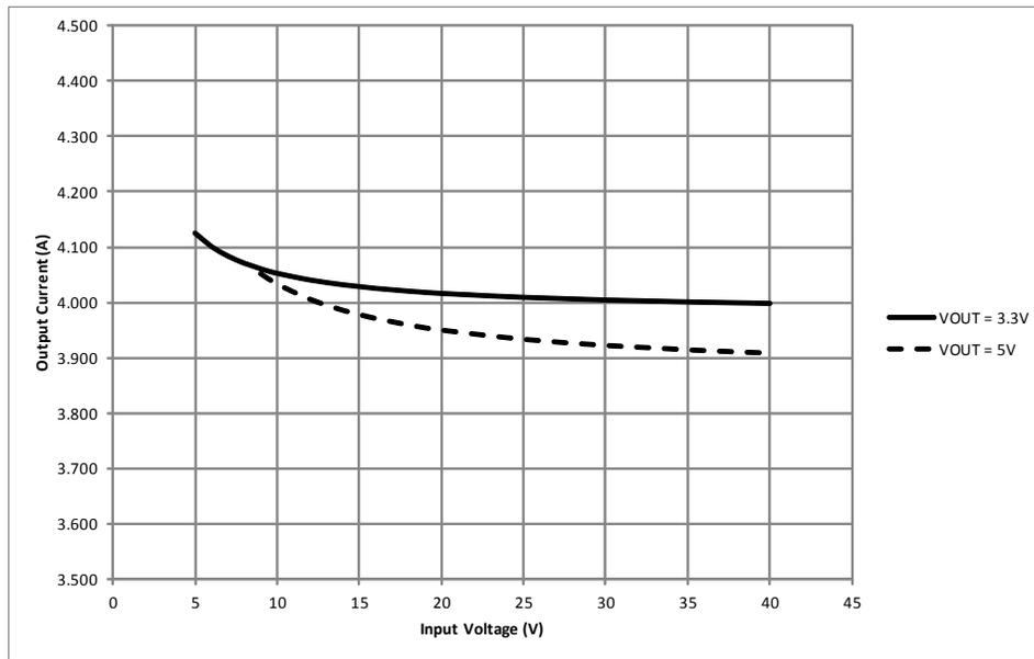
**Figure 7. Maximum Output Current**
