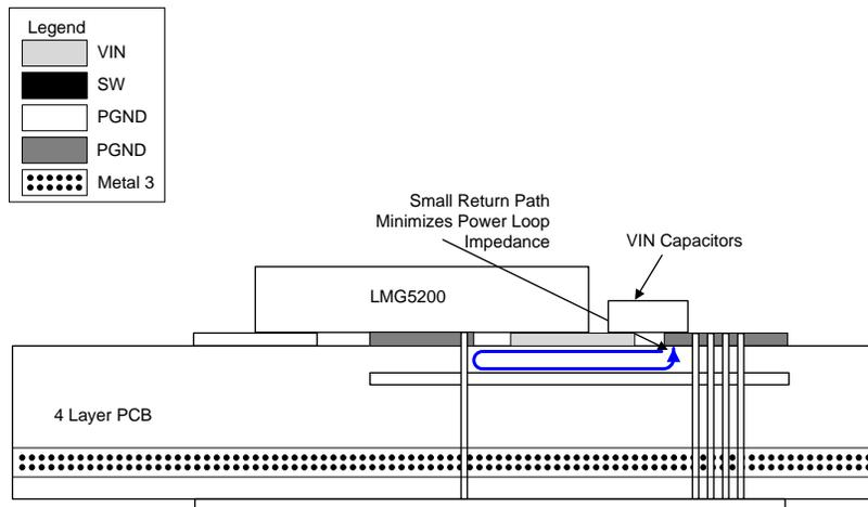
**Figure 3. Cross-Section of the LMG5200 PCB Layout**
