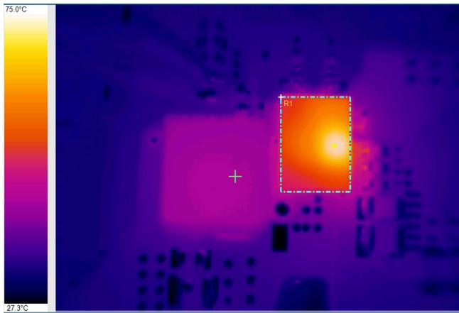
Figure 11. With No Airflow, 2-W Dissipation
