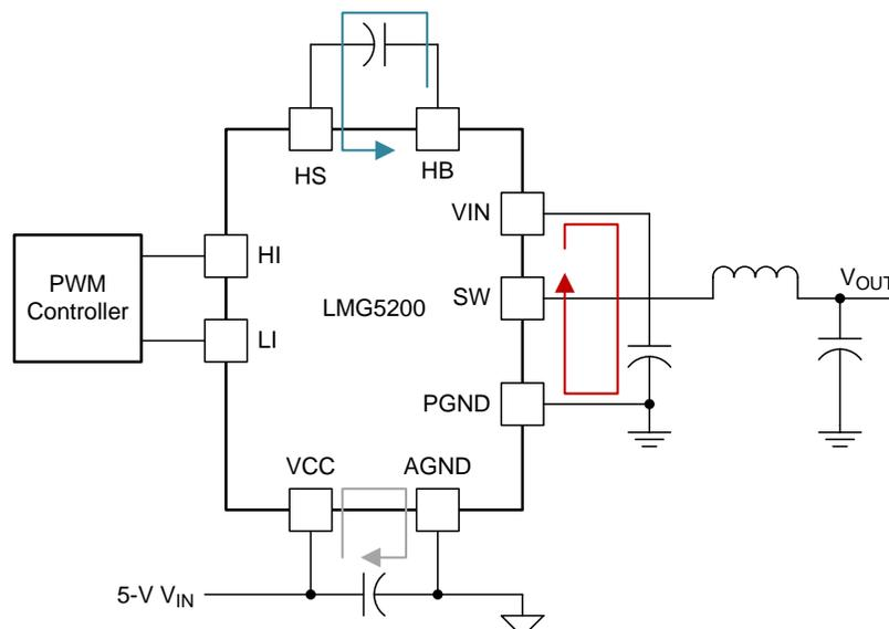
Figure 1. Buck Converter Application Using the LMG5200 Power Stage
