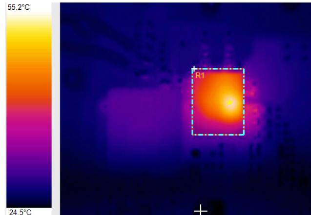
Figure 12. With Airflow, 2-W Dissipation
