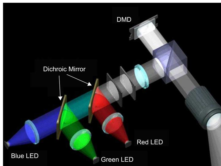
**Figure 1. Optical Layout of DLP® LED Projector**
