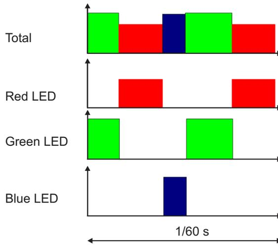
**Figure 2. Conventional LED Driving Scheme in 60 Hz Video**
