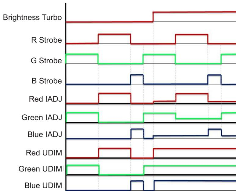
Figure 7. Logic Chart of Brightness Turbo Inputs/Outputs
