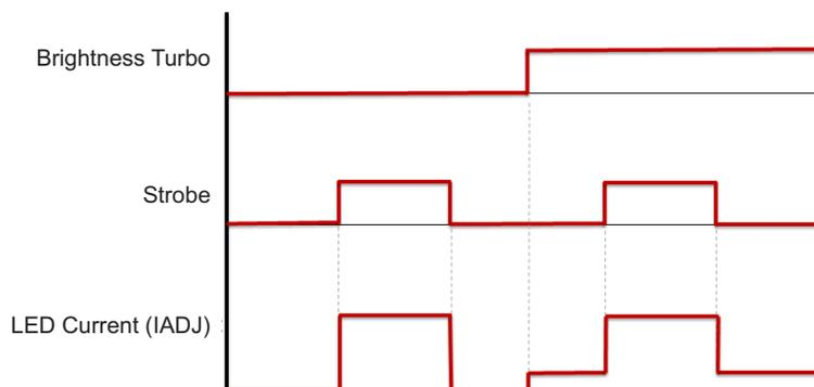
Figure 5. Logic Chart of Control over IADJ
