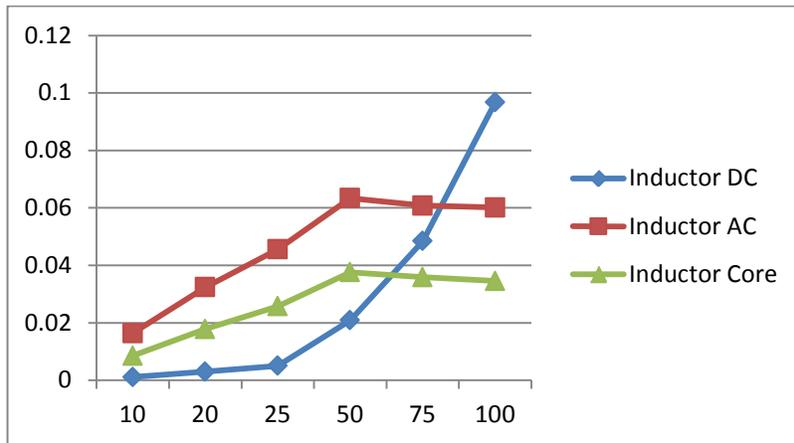
**Figure 7: Variation of Inductor Losses with Brightness**
