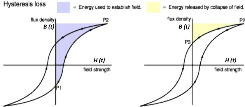
**Figure 3.  $B(t)$  as a function of  $H(t)$  for a sinusoidal input**
