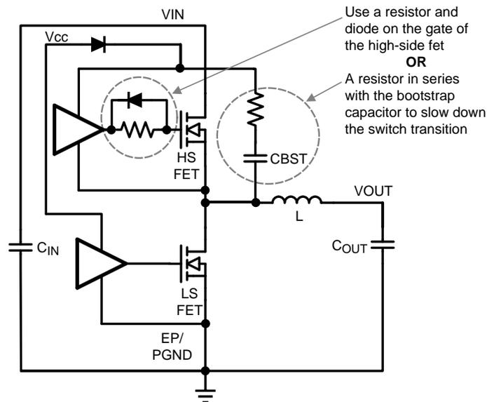
**Figure 2. Methods for Slowing Down the Transition Rise-Time**
