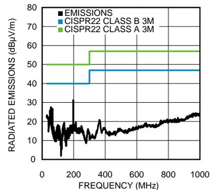
Figure 8. Board 6 (Extend Switch node 4 Layer)
