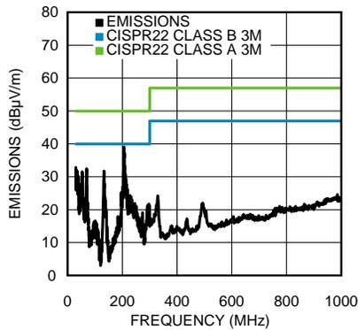
Figure 5. Board 3 (- SW NODE COPPER 2 Layer)
