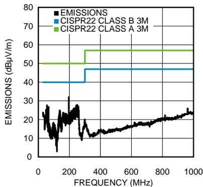
Figure 7. Board 5 (Extend Switch node 2 Layer)
