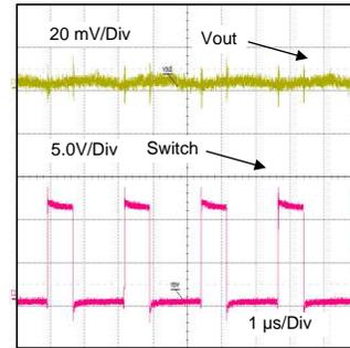
Figure 13. Switching waveform with extra ground plane (Board2)
