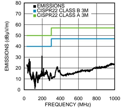
Figure 4. Board 2 (+GND PLANE 4 Layer)
