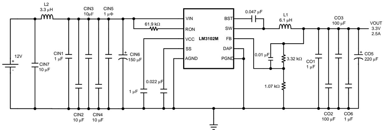
Figure 31. EMI Test Board Schematic
