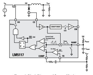
Figure 6. Block Diagram of Current Monitor and Ramp Generator
