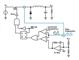
Figure 1. Traditional Cycle-by-Cycle Peak Current Limiting
