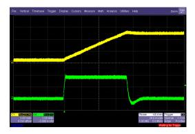
Figure 9. CC and CV Regulation Waveforms (Upper: Output Voltage, Lower: Output Current)
