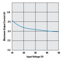
Figure 4. Maximum Output Current vs Input Voltage
