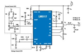
Figure 8. Constant Voltage Regulator with Precision Current Limit
