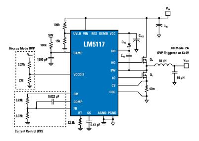
Figure 11. Constant Current Regulator with Hiccup-Mode Over-Voltage Protection
