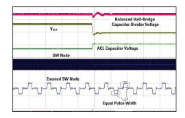
Figure 5. Balanced Half-Bridge Capacitor Waveform in a Soft-Short Condition Employing Average Current Limit
