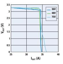
Figure 4. V<sub>out</sub> vs I<sub>out</sub> Curve Illustrating Brickwall Current Limiting
