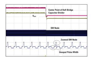
Figure 2. Current Limit Waveforms of Half-Bridge Topology Employing Peak Cycle-by-Cycle Current Limit
