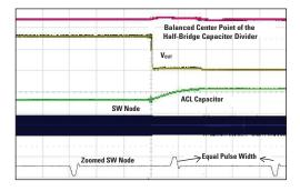
Figure 6. Balanced Half-Bridge Capacitor Waveform in a Hard-Short Condition Employing Average Current Limit
