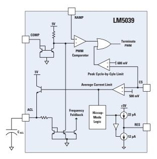
Figure 3. Average Current Limit Circuit Implementation in LM5039 Half-Bridge Controller
