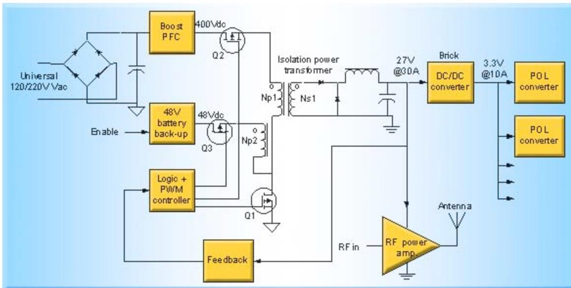
Fig. 3. 3G Base station RF power amp supply
