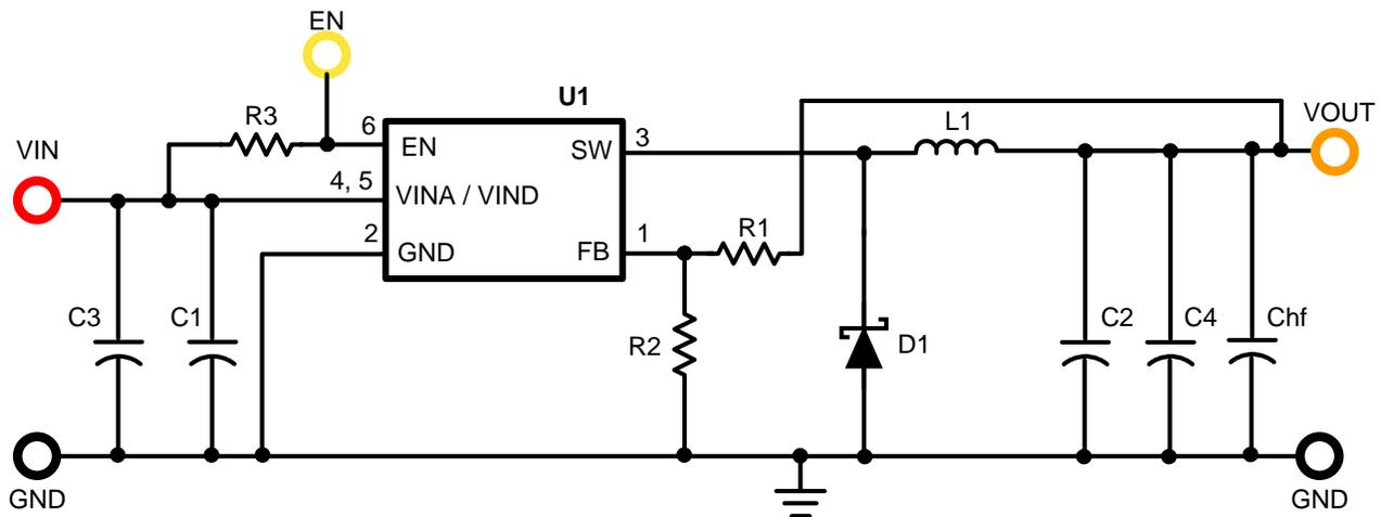
Figure 3. LMR10515 Demo Board Schematic
