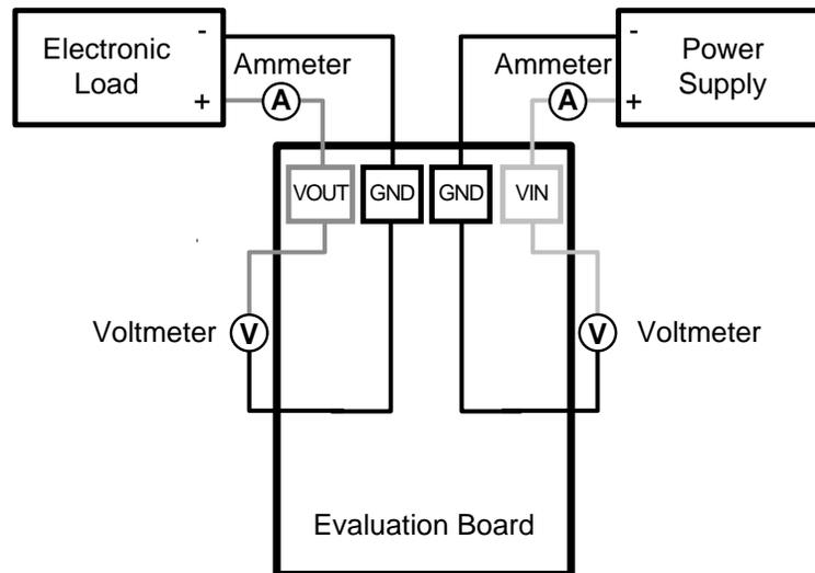
**Figure 5. Efficiency Measurements**
