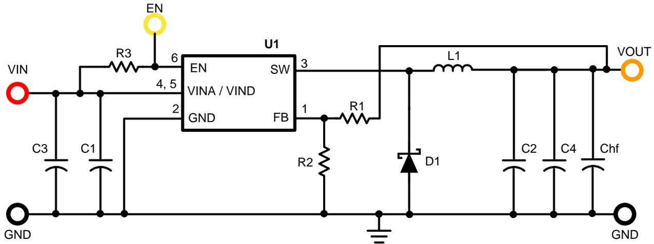
**Figure 4. LMR10520 Demo Board Schematic**
