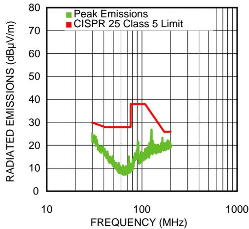
**Figure 18. 30 MHz-200 MHz Vertical 1A Load**
