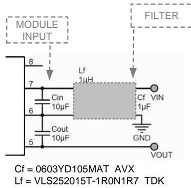
Figure 8. LC Input Filter for Conducted EMI
