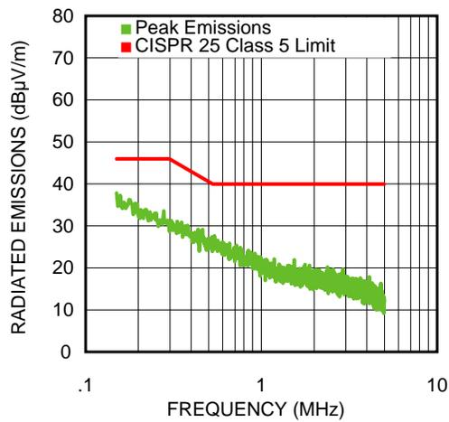
Figure 4. CISPR 25 Class 5 Radiated EMI 1A Load
