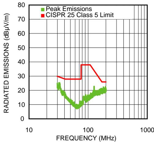
**Figure 16. 30 MHz-200 MHz Horizontal 1A Load**
