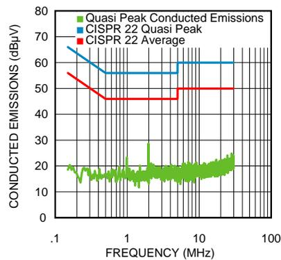
Figure 9. Conducted EMI with the LC Input Filter 1A Load
