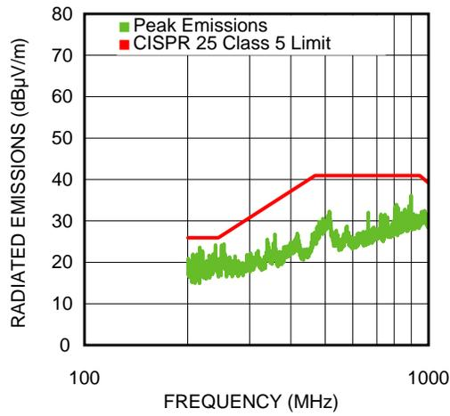
**Figure 23. 200 MHz-1000 MHz Vertical 650 mA Load**
