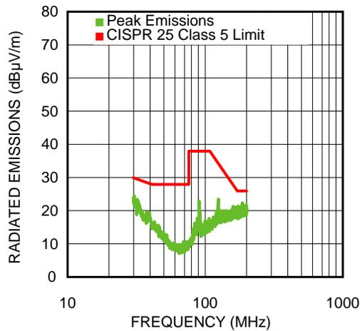
**Figure 19. 30 MHz-200 MHz Vertical 650 mA Load**
