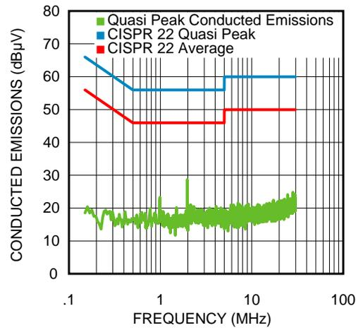
**Figure 2. CISPR 22 Conducted EMI 1A Load
