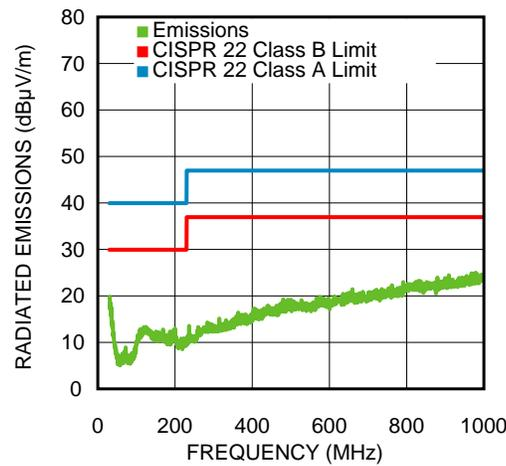
**Figure 3. CISPR 22 Radiated EMI 1A Load
