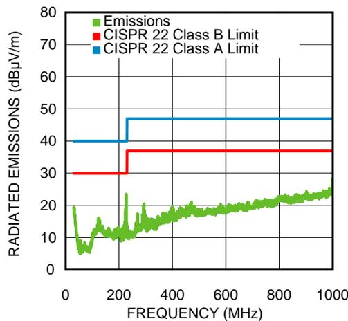
**Figure 1. CISPR 22 Radiated EMI 1A Load
