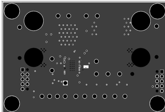
Figure 23. Board Mid Layer 1 (ground plane)
