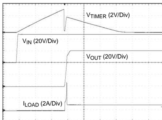
Figure 16. Turn-On Sequence into a  $4\Omega$  Load (50 ms/DIV)
