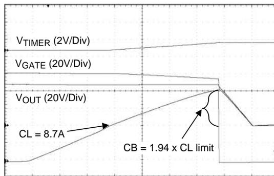
Figure 15. Circuit Breaker Response (500  $\mu$ s/DIV)
