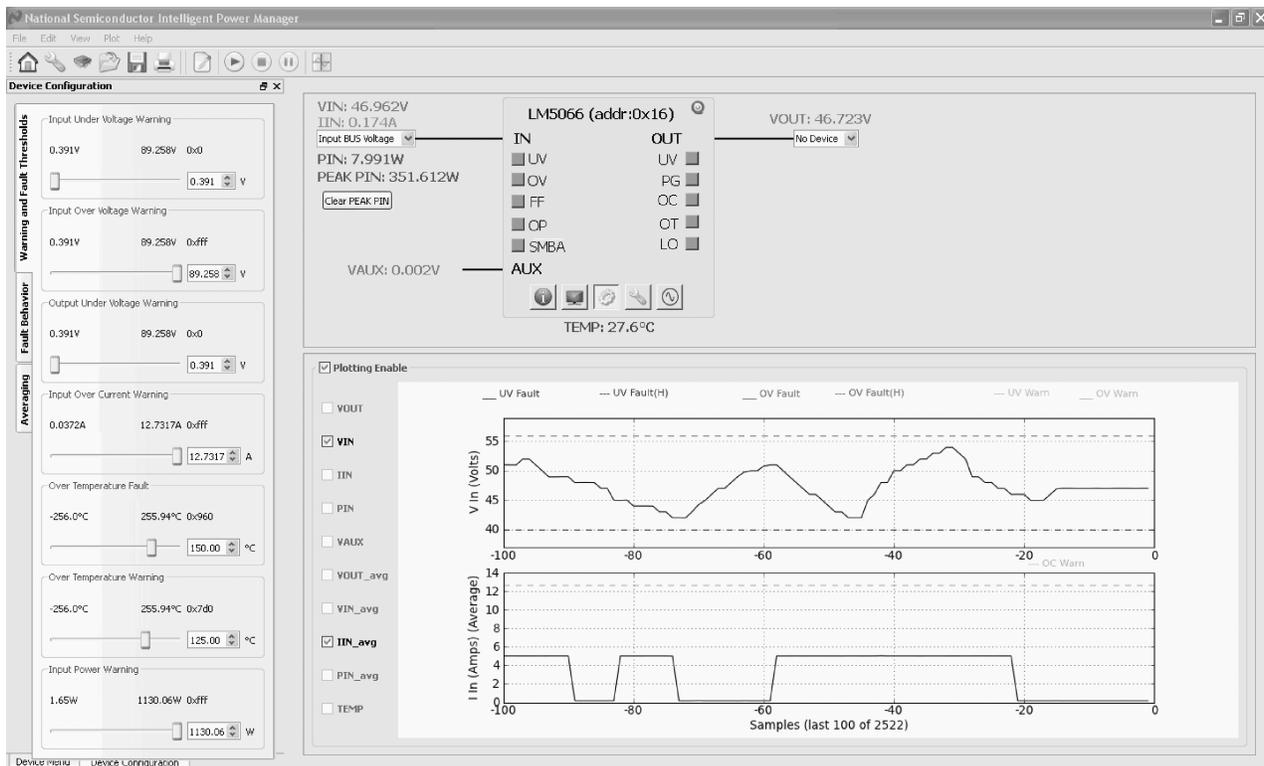
Figure 7. LM5066 GUI with Telemetry Plotting Tool Enabled
