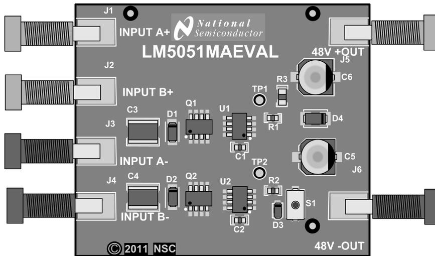
Figure 8. Component Placement
