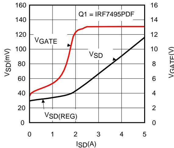
Figure 3. Gate Drive vs Drain to Source Voltage
