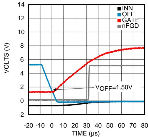
**Figure 5. OFF pin Going Low, Gate Drive Active**
