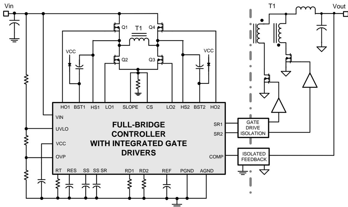
**Figure 1. Simplified Full-Bridge Converter**
