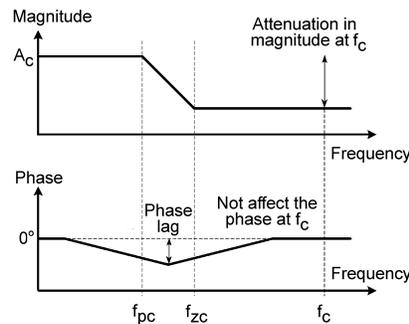
**Figure 3. Frequency Response of a Lag Compensator**
