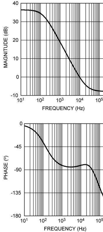
**Figure 5. Frequency Response of the Un-Compensated System**
