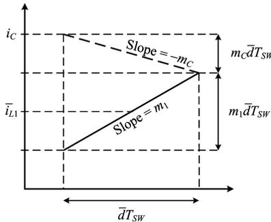
Figure 2. Inductor Current Waveform at the On Period
