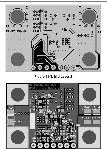
Figure 11-4. Bottom Layer (View From the Bottom)
