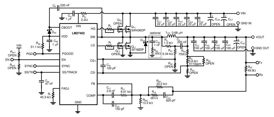
Figure 4-1.  $V_{IN}$  = 4.5 V to 20 V,  $V_{OUT}$  = 1.5 V,  $I_{OUT}$  = 20 A
